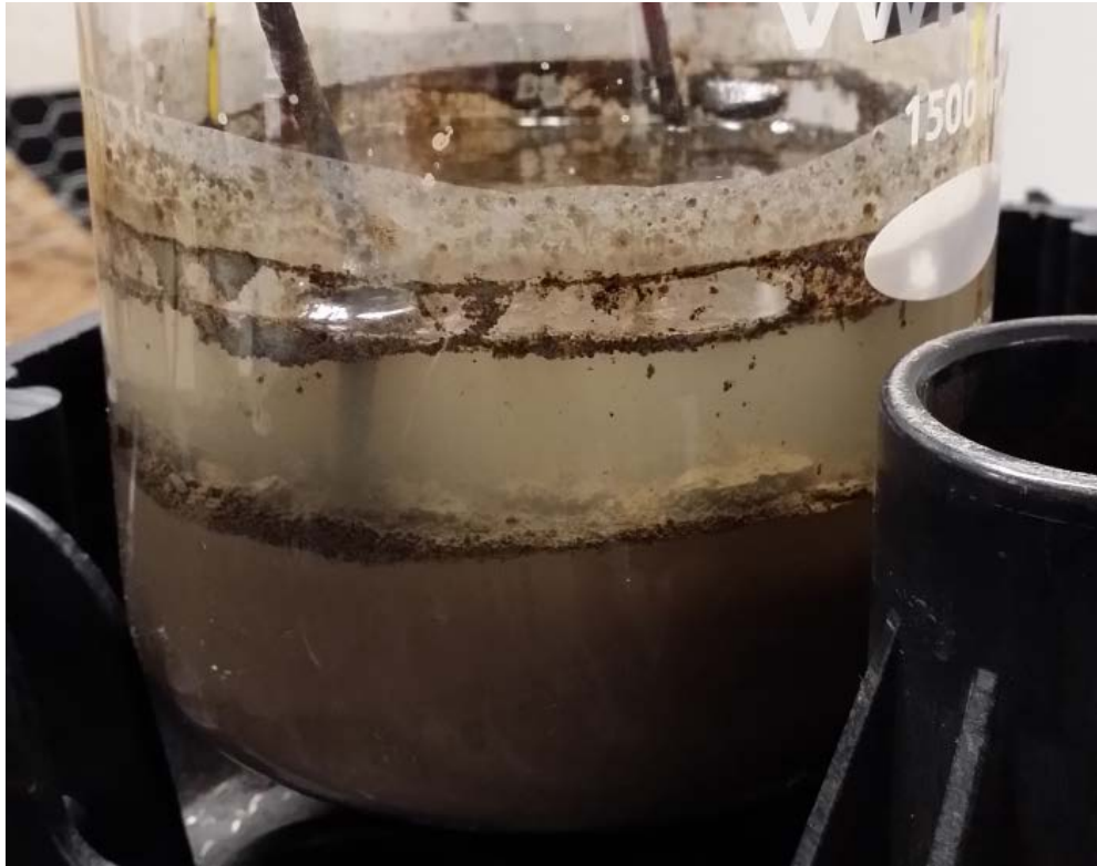
Water layer formation on top after autotransformer treatment (exp-2)
