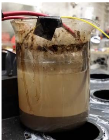
Tailings separation after Auto-transformer treatment
