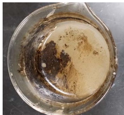
Bitumen layer on top of treated tailings
