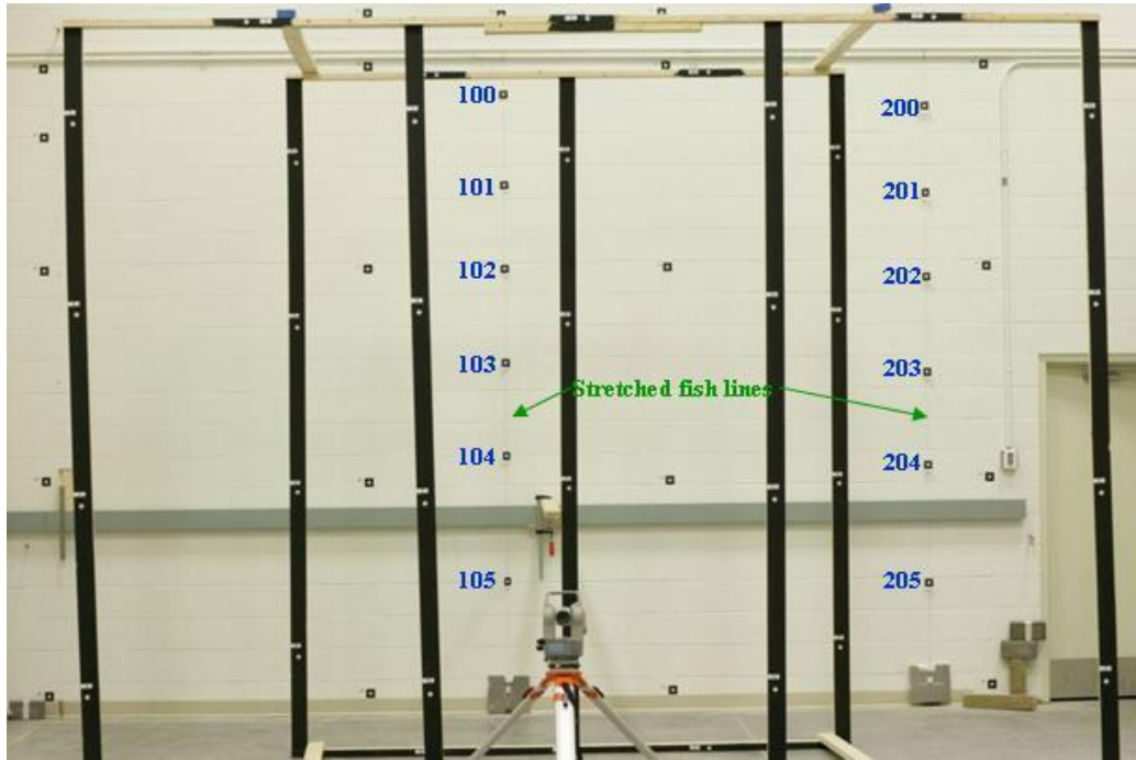
Figure 5.6 Straight-line features at the test range #2
