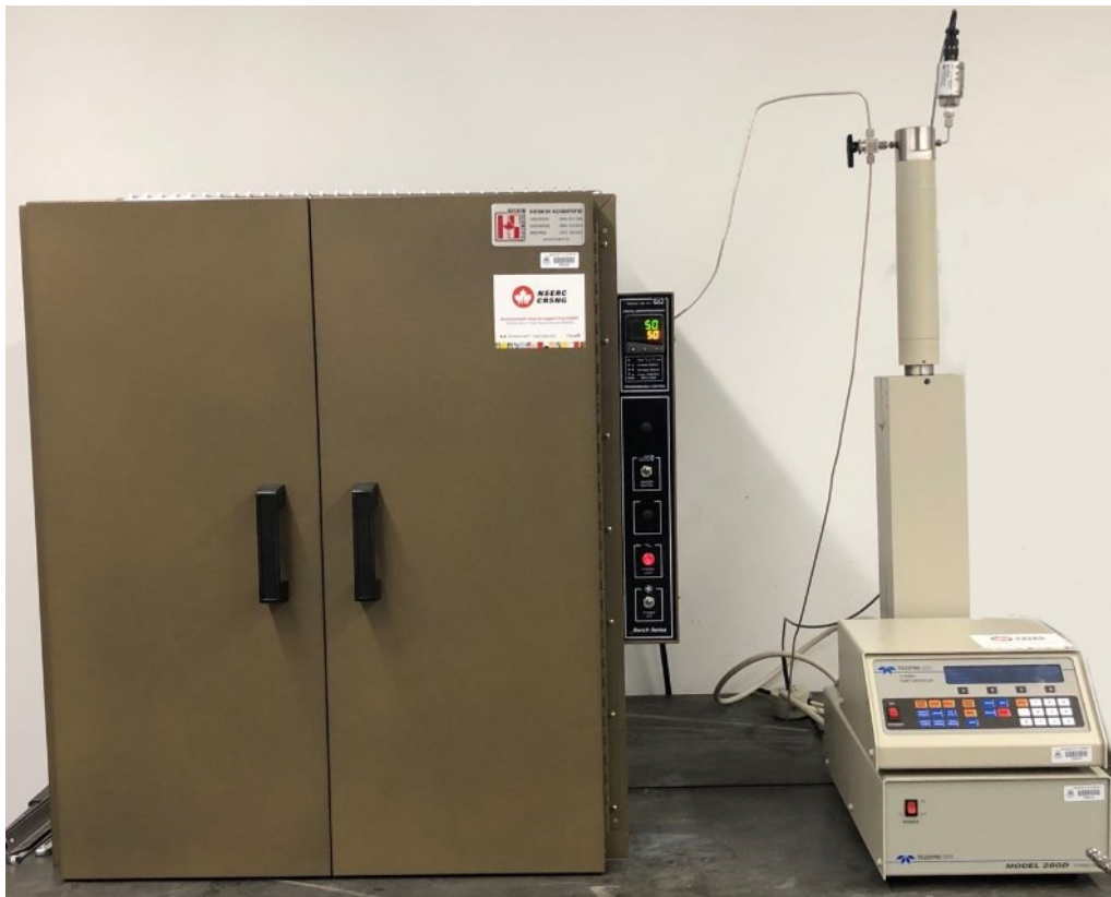
Figure 3-5 Equipment used for curing cement samples.
