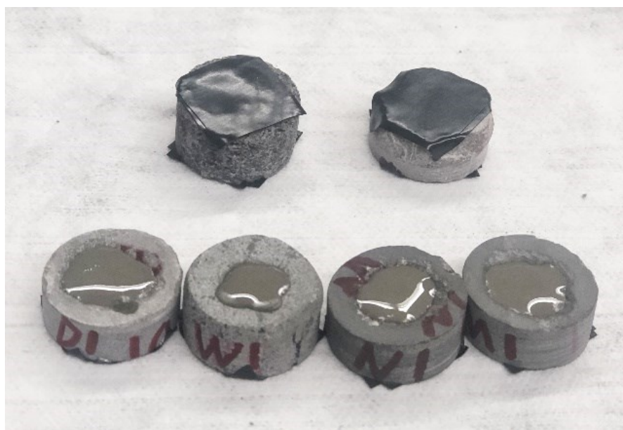
Figure 3-14 Prepared cement-rock samples.
