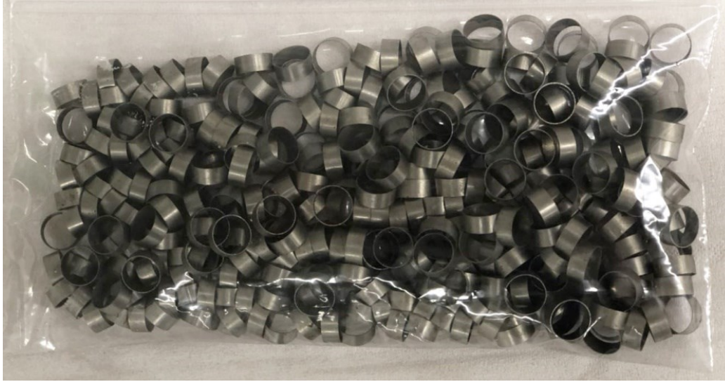
Figure 3-8 Short sections of the 304 stainless steel pipe.
