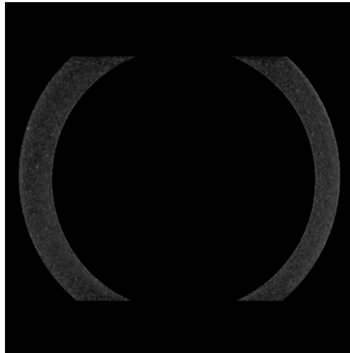
Figure 8-6 Processed CT image after removing casings and white line artifacts.
