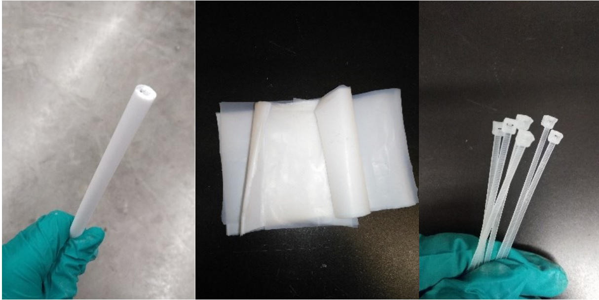
Figure 3-3 High-temperature PTFE (Teflon) pipe, Teflon film, no-gap cable ties.
