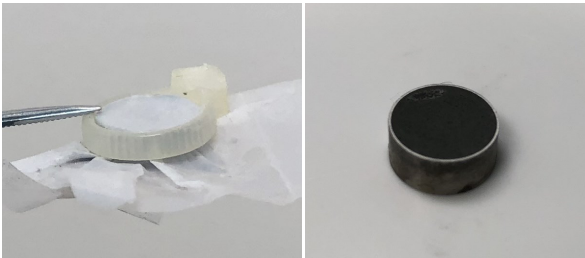
Figure 3-9 Cement-casing sample after curing and after removing the sealing materials.
