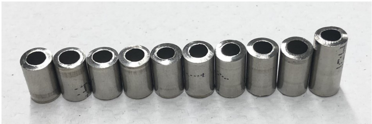
Figure 9-2 Short casing sections machined from 316 stainless steel tubing pipes.
