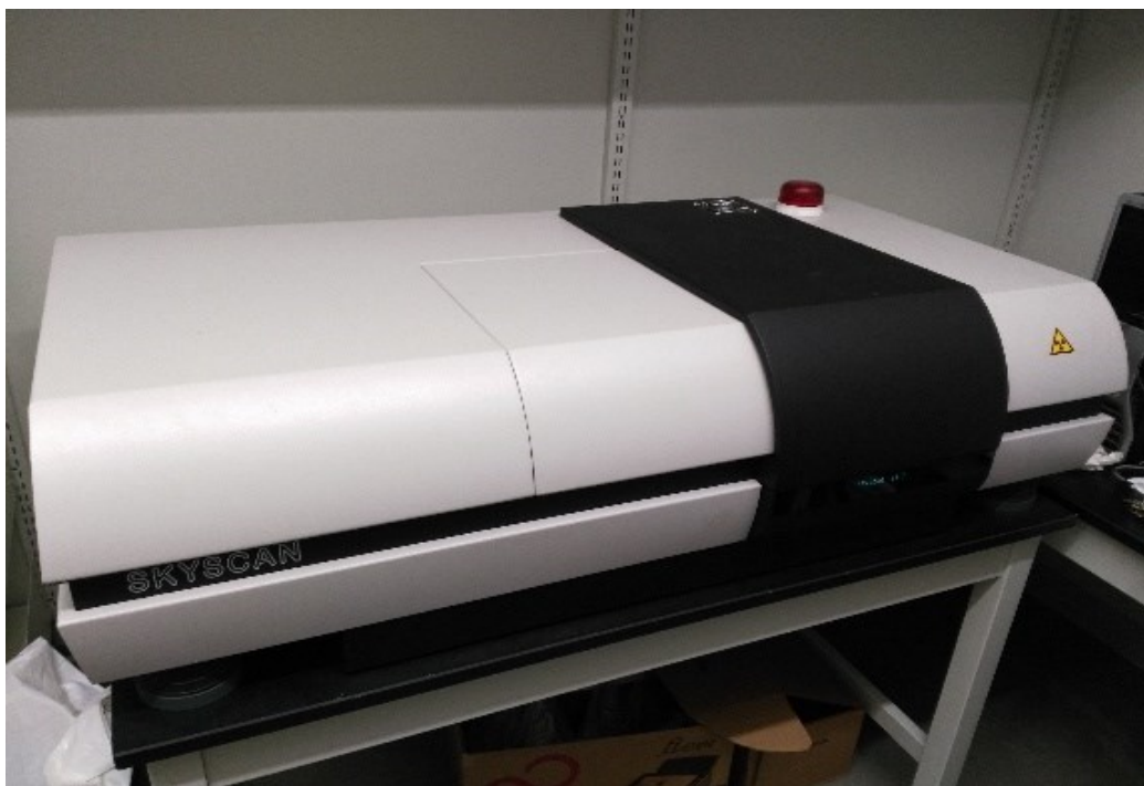
Figure 3-16 SkyScan 1172 desktop X-ray micro-CT scanner.
