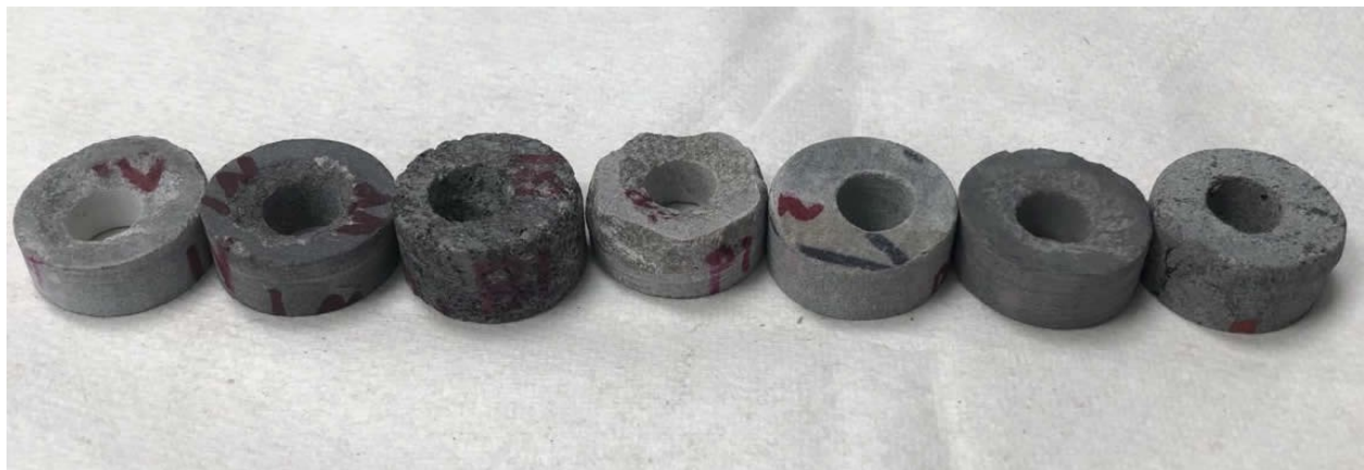
Figure 9-1 Hollow formation rock cylinders.
