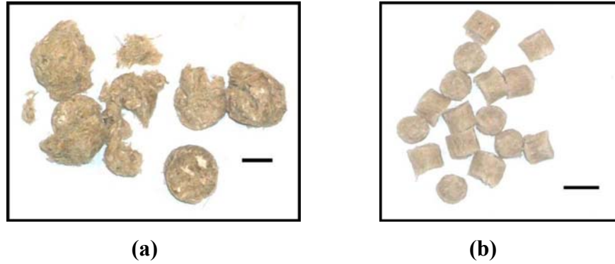
Fig. 3.2 Pellets of (a) hemp bast fibers and (b) 20 wt% hemp-fiber-reinforced HDPE (black line is 5.0 mm)
