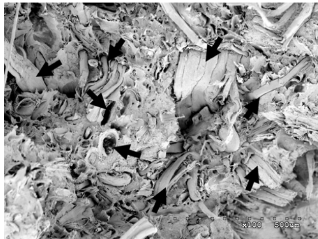
Fig. 6.4 Scanning Electron Microscope (SEM) image of 20% hemp-HDPE sample fatigue fracture surface immersed in water for 35 days under maximum applied fatigue stress ( \sigma_{max} ) of 19.8 MPa. Interfacial separation is noted by arrows.
