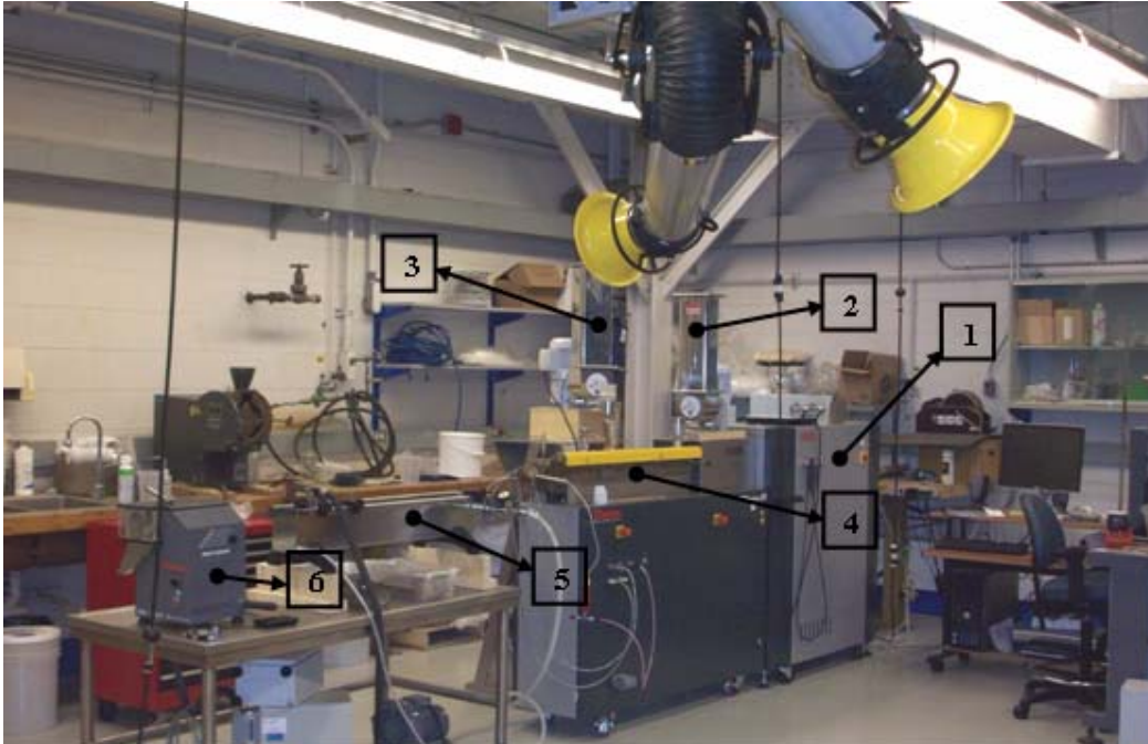
Fig. 3.3 NFRP pellet production line: (1) Control Unit (2) HDPE Pellets Feeder (3) Natural Fiber Pellets Feeder (4) Batch Mixture Extruder (5) Cooling Water Bath (6) Pelletizer.
