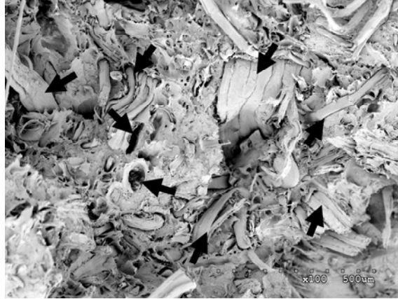
Fig. 2.2 Scanning Electron Microscope (SEM) image of a tension-tension fatigue fracture surface of short-hemp-bast fiber-reinforced HDPE (20% hemp-reinforced HDPE) immersed in water for 35 days; the fatigue test was performed at maximum fatigue stress of 19 MPa with frequency f=3.0 Hz and fatigue stress ratio R=0.1 [36].
