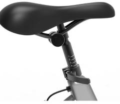
Figure 18: Integrated break cable
