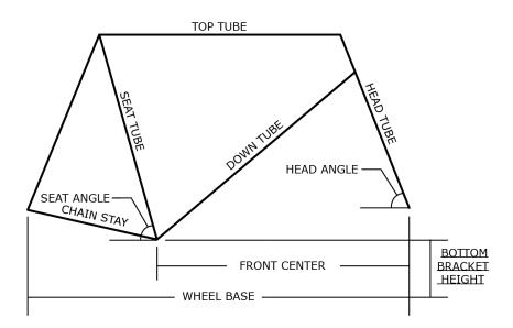
Figure 15: Bike frame structure
