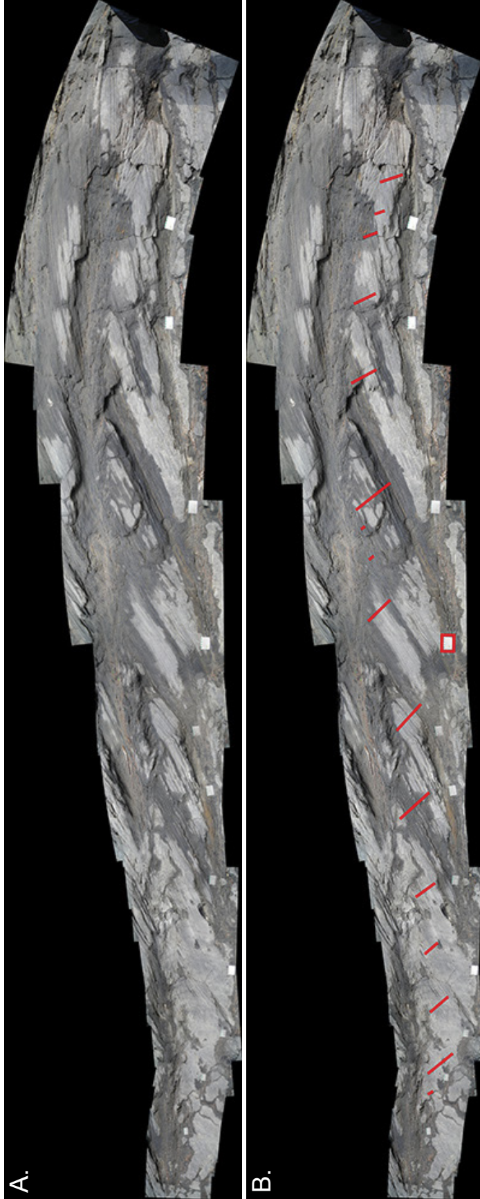
Figure 2.3: A) Photomosaic of the analyzed dune. B) Photomosaic indicating the exact foreset-thickness measurement path, spanning from right to left along the dune. Note that each scale card is 9 cm in length. Thickness measurements were completed in Adobe Photoshop. Calibration of scale was completed using the scale card outlined by the red box.
