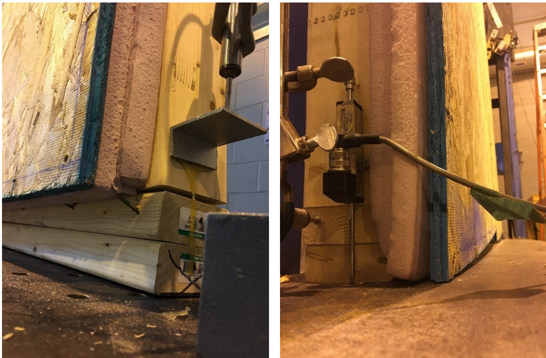
Figure D.4: Failure mode of S7 Shear wall: S7 wall did not fail; the OSB was squashing the insulation as the displacement was increasing
