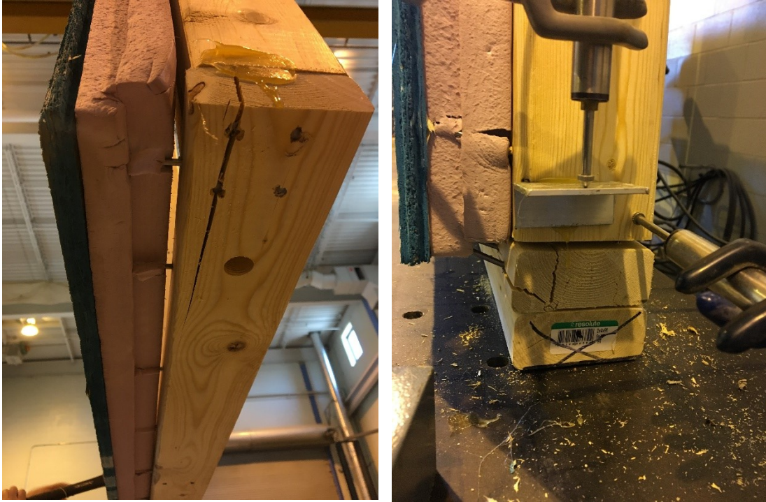
Figure D.3: Failure mode of S5 and S6 Shear wall: nail bending and nail pullout (splitting of the bottom plate occurred during nailing of the framing)
