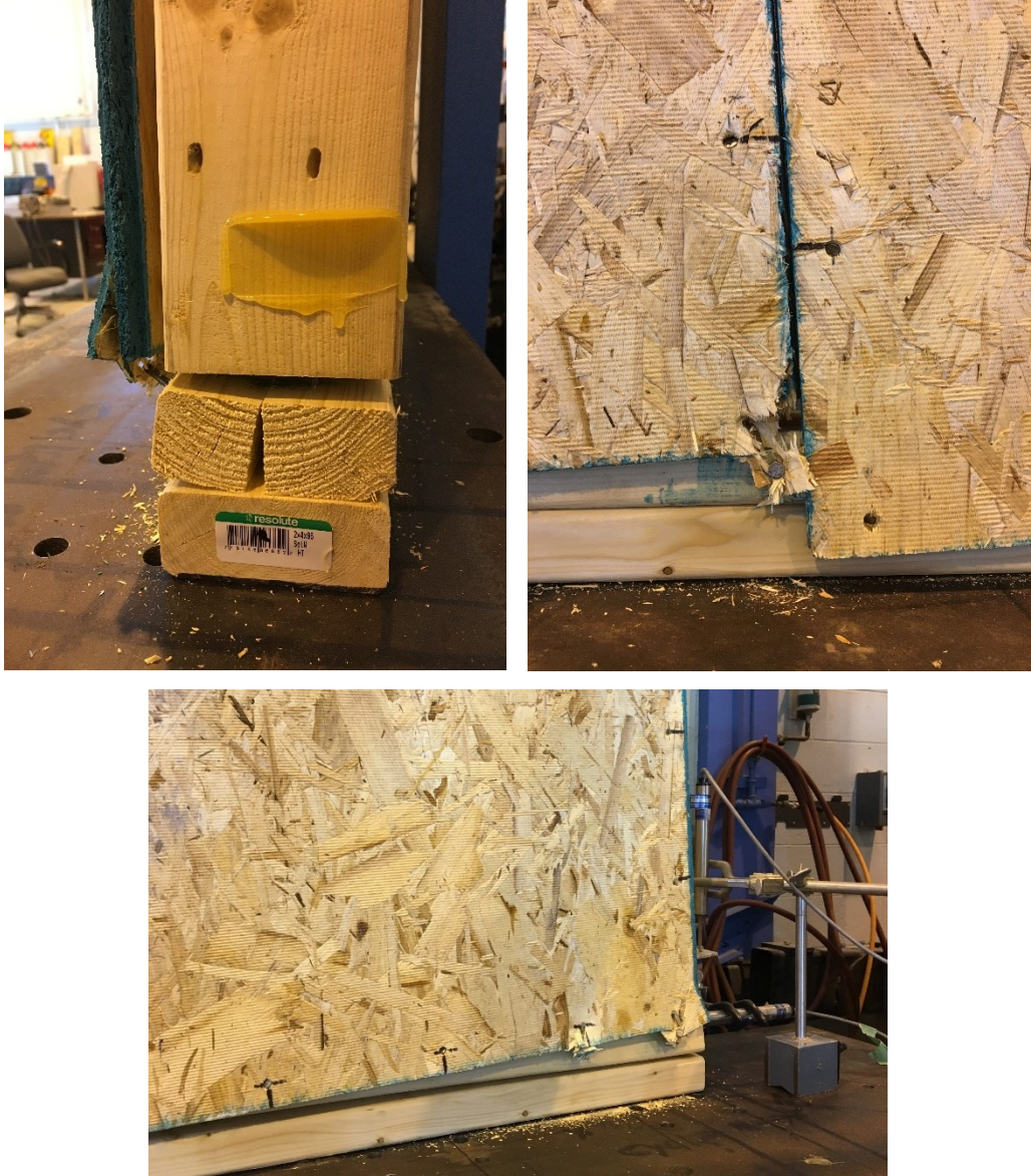
Figure D.1: Failure mode of S1 Shear wall: nail bending, splitting of the bottom plate, sheathing tearing, nail head pull through
