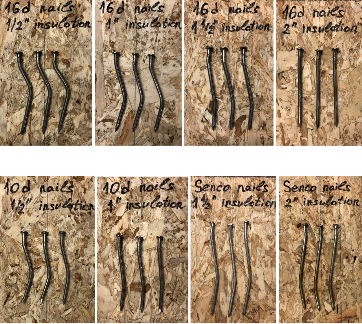
Figure C.2: Nails after the testing of nail joints
