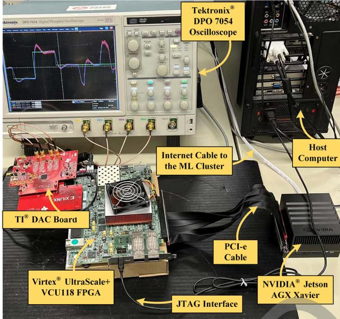
Fig. 10. Hardware components of the real-time IIL emulation system.
