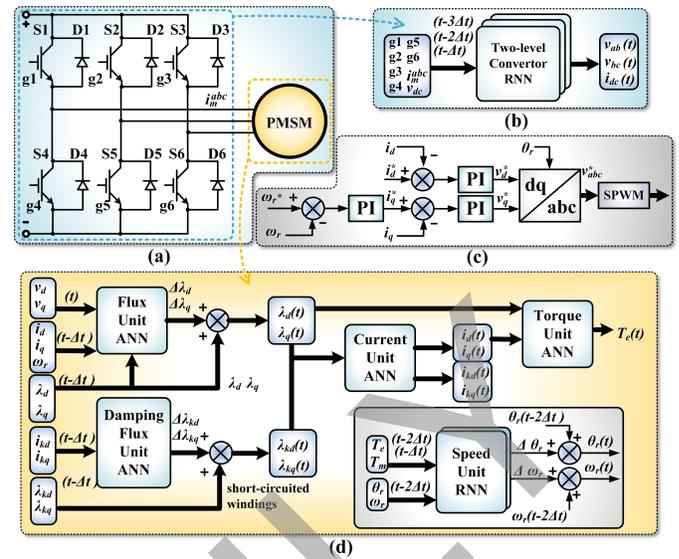
Fig. 7. Two-level converter propulsion subsystem: (a) topology; (b) converter RNN model; (c) control strategy; (d) PMSM ANN-based detailed model.
