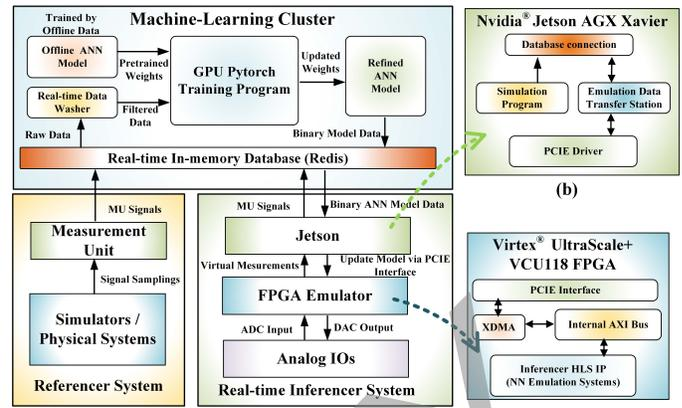
Fig. 8. IIL system software structure: (a) IIL topology and connection; (b) Jetson function; (c) FPGA function.
