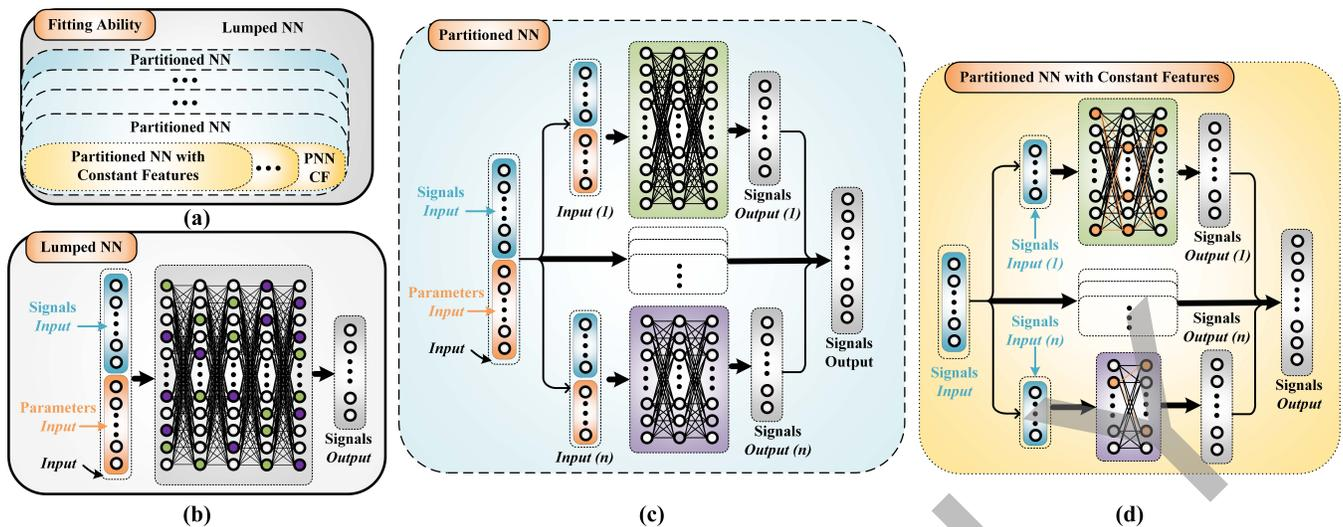
Fig. 1. NN structure: (a) different NNs' fitting ability; (b) lumped NN; (c) partitioned NN; (d) partitioned NN with constant features.
