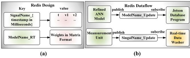
Fig. 9. Real-time in-memory database (Redis): (a) internal design; (b) dataflow.
