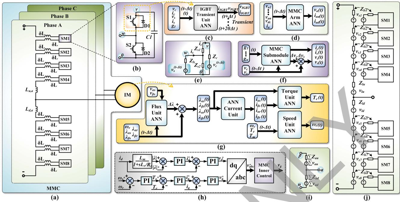
Fig. 5. MMC-IM propulsion subsystem: (a) MMC-IM subsystem topology; (b) MMC submodule topology; (d) MMC arm ANN model; (e) MMC submodule equivalent circuit; (f) MMC submodule ANN model; (g) IM ANN detailed model; (h) control strategy; (i) MMC single-phase equivalent circuit; and (j) MMC single-phase TLM equivalent circuit.
