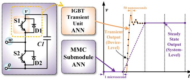
Fig. 6. SiC IGBT hybrid model output waveform.
