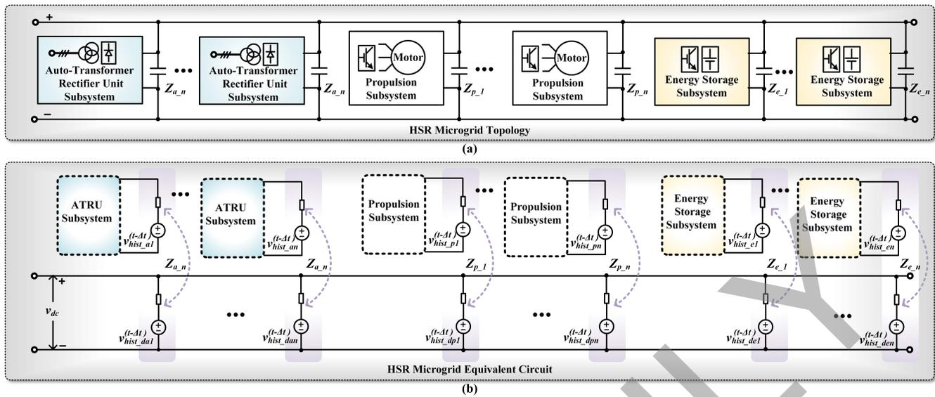
Fig. 2. HSR microgrid: a) general topology; b) equivalent circuit.
