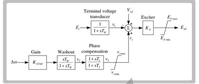
Fig. 10. Excitation system with AVR and PSS.
