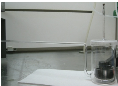
Figure 3-1: Vertical quartz reactor designed to fit into the fixed-bed muffle furnace set-up.
