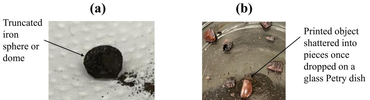
Figure 8.2: (a) Freeze casted iron dome (b) Freeze casted object shattered into pieces due to the lack of heat treatment.
