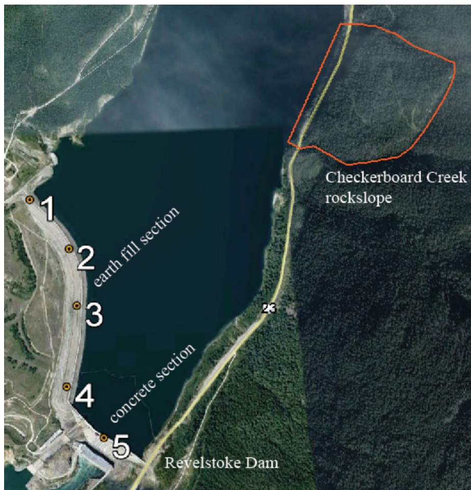
Figure 4-12 Revelstoke Dam and Checkerboard Creek rock slope with locations where the impulse wave run up characteristics were estimated. Ground image extracted from Google Inc. (2012).
