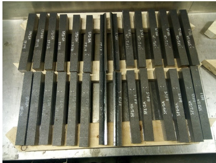
Figure 3-11: Sectioning strips for residual stress measurements (Unsworth et al. 2019)
