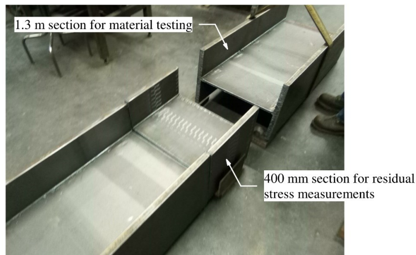
Figure 3-16: Ancillary girder used for residual stress measurements and material testing (adapted from Unsworth et al. 2019)
