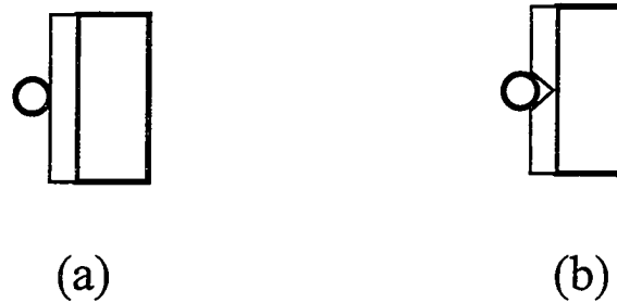
Figure 2.3: Extensometer Grip Modification (a) The original blade geometry (b) Modified blade geometry by filing a notch in the center of the blade. This modification improved the ease of installation and reduced the drift in the extensometer as the specimen rotated under torsional loading.
