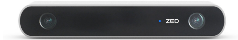
Figure 6.12: ZED camera used for localization
