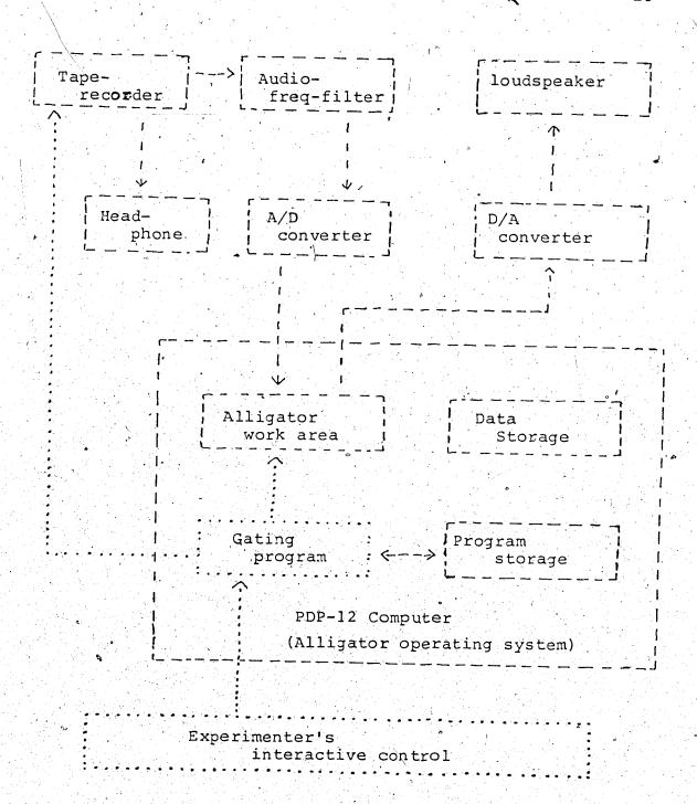
Figure 1: Block diagram of digital gating and segmentation.
