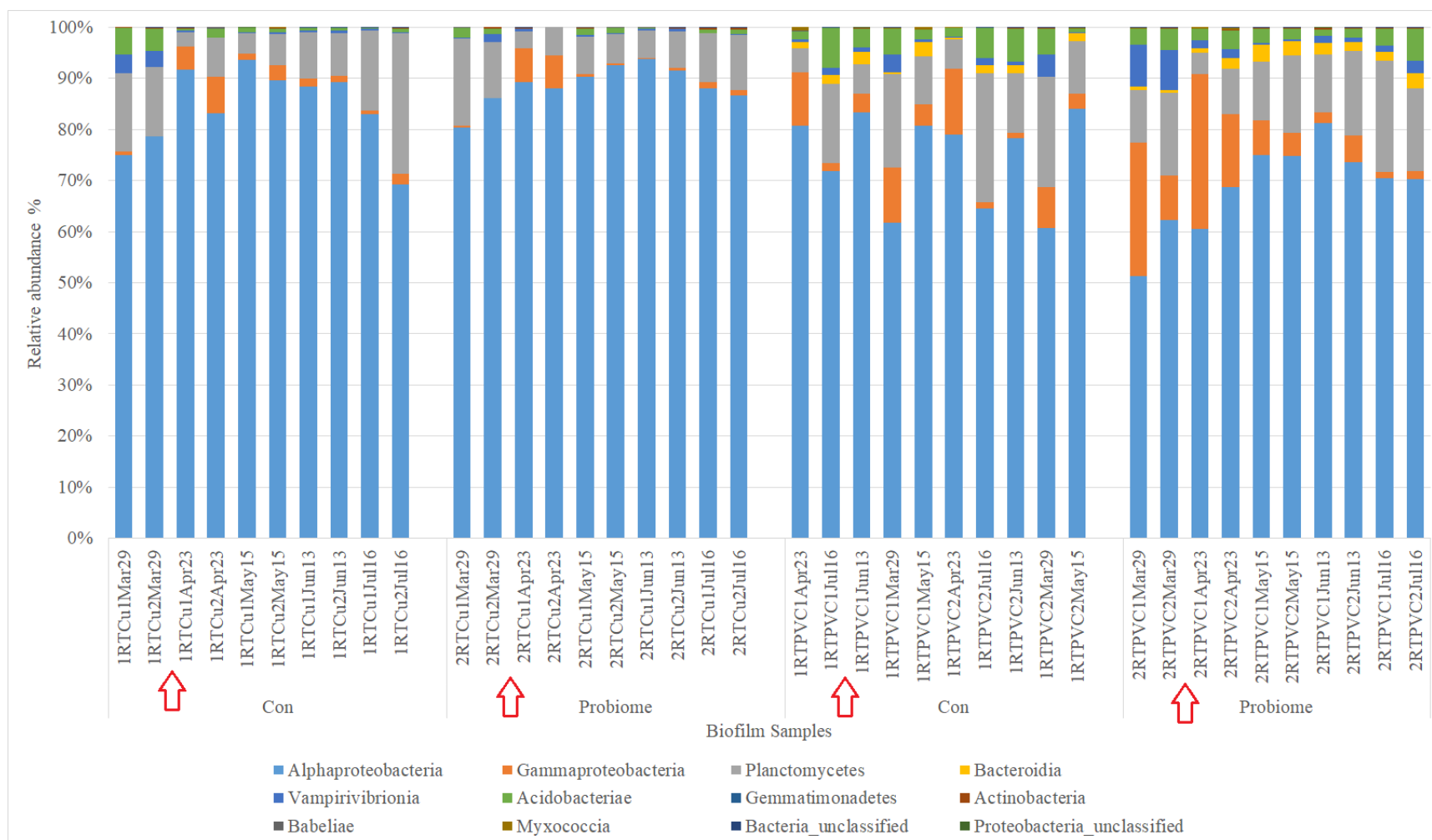
Figure S5.2: RA of different bacterial taxa in class level in biofilms on Cu and PVC coupons under HT (Top) and RT (Bottom) with and without probiome. L. pneumophila and upstream probiome were introduced after Mar29 samples (Red Arrow).
