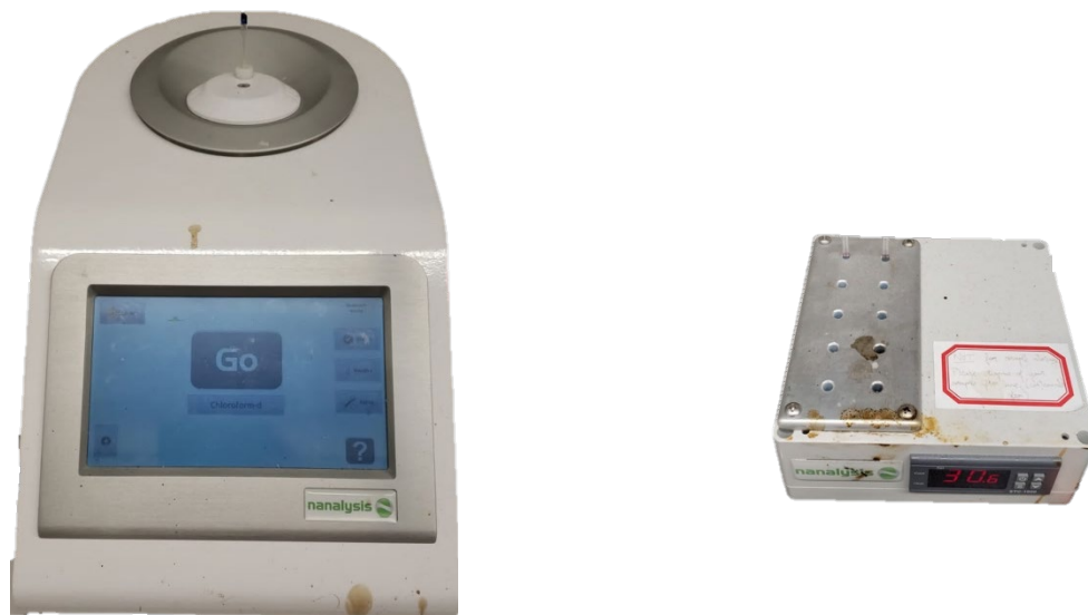
Figure 3.11. (left) Nanalysis 60 MHz NMReady – 60 Nuclear Magnetic Resonance (NMR) Spectrometer, (right) heating area for the samples used. The temperature set point was 30 °C.
