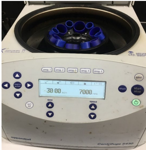
Figure 3.4. (left) The Eppendorf Centrifuge 5430 used in the centrifugation for the separation of the components of the froth treatment tailings, (right) rotor used alongside the centrifuge for the separation of the tailings.
