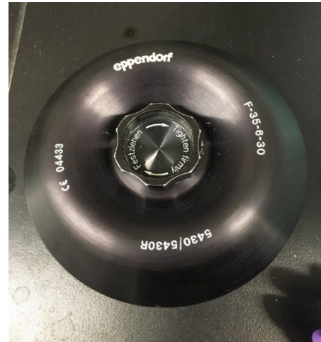
Figure 3.4. (left) The Eppendorf Centrifuge 5430 used in the centrifugation for the separation of the components of the froth treatment tailings, (right) rotor used alongside the centrifuge for the separation of the tailings.
