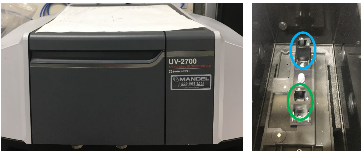
Figure 3.10. (left) The Shimadzu UV-2700 Spectrophotometer used for the qualitative analysis of the toluene and heptane analysis; (right) interior of the spectrophotometer, with the back position for the baseline cuvette (highlighted in blue) and for the sample (highlighted in green).
