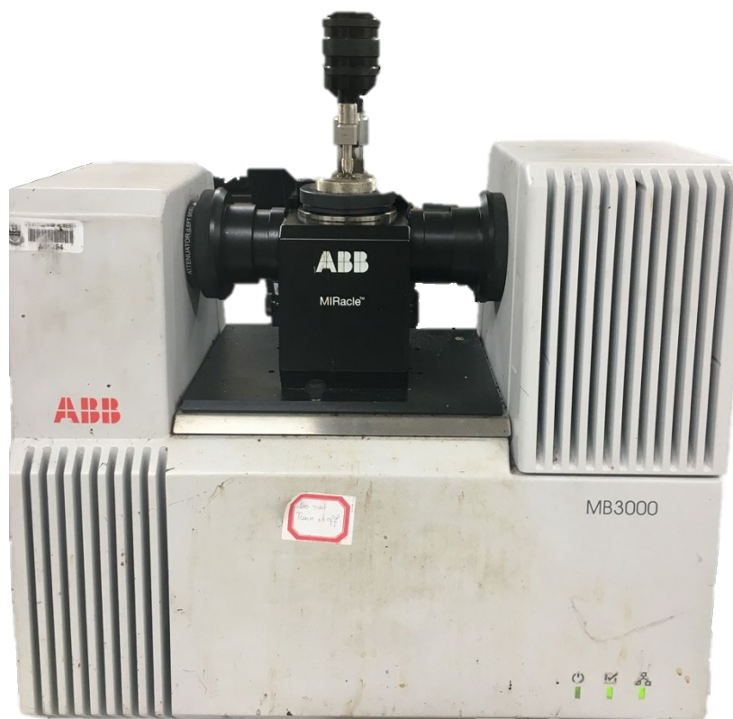
Figure 3.9. ATR-FTIR used for the qualitative analysis of the chloroform extracts for various experimental conditions.
