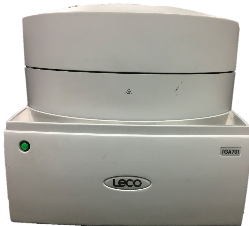
Figure 3.3. LECO Thermogravimetric Analyzer – TGA 701 Instrument
