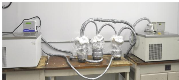
Figure 3. Freezing test setup during freezing all three samples.
