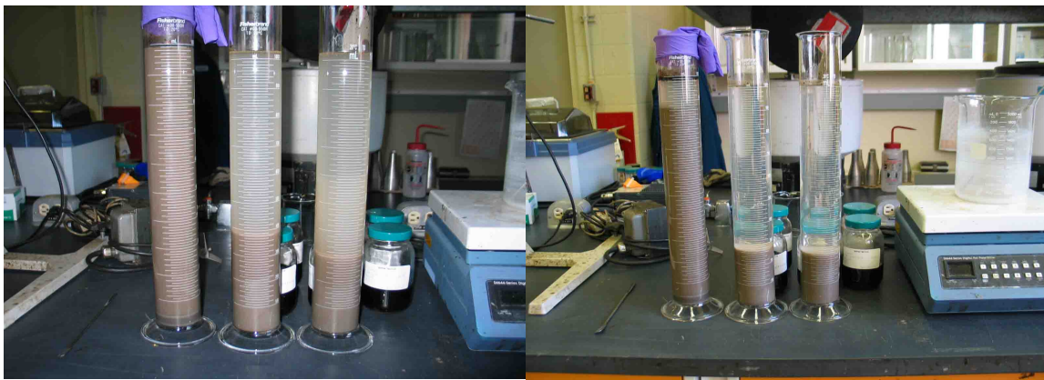
Figure 8. The effect of mechanical energy on tailings clay dispersion. From left to right, the 4x dilution MFT was stirred for ten, five, and one minutes respectively. The photo on the left is after 24h settling and the photo on the right is after 72h.
