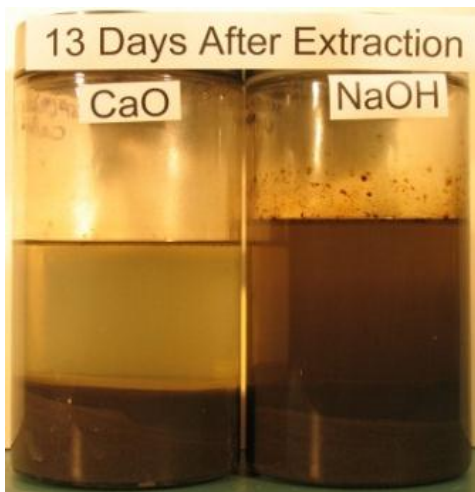
Figure 4. Filtered (<45 \mu\text{m} ) fraction of non-additive and \text{CaO} and \text{NaOH} additive extraction tailings.
