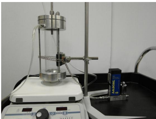
Figure 1. Apparatus used for solvent release experiments.
