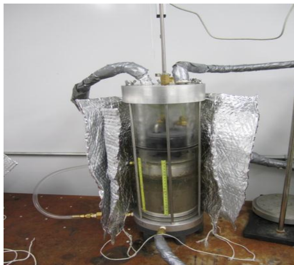
b) Frozen/thawed MFT consolidometer
