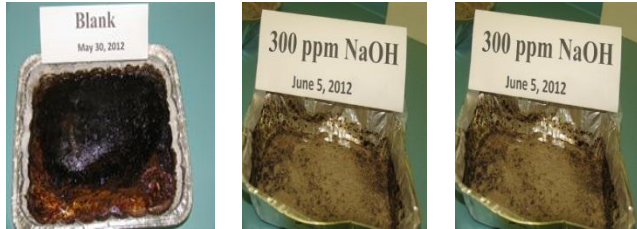
Figure 3. Images of oven dried tailings.
