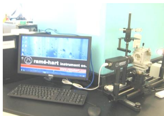
Figure 5. Contact angle of distilled water on the coated glass squares was measured by an advanced goniometer.
