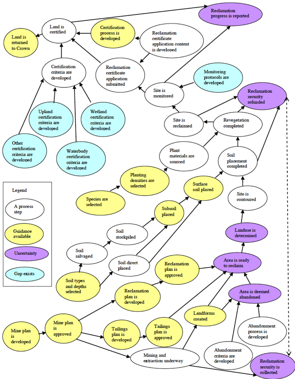
Figure 6. Simplified process-oriented view of the "reclamation system". (R.K. Jones and D. Forrest, October 2010).
