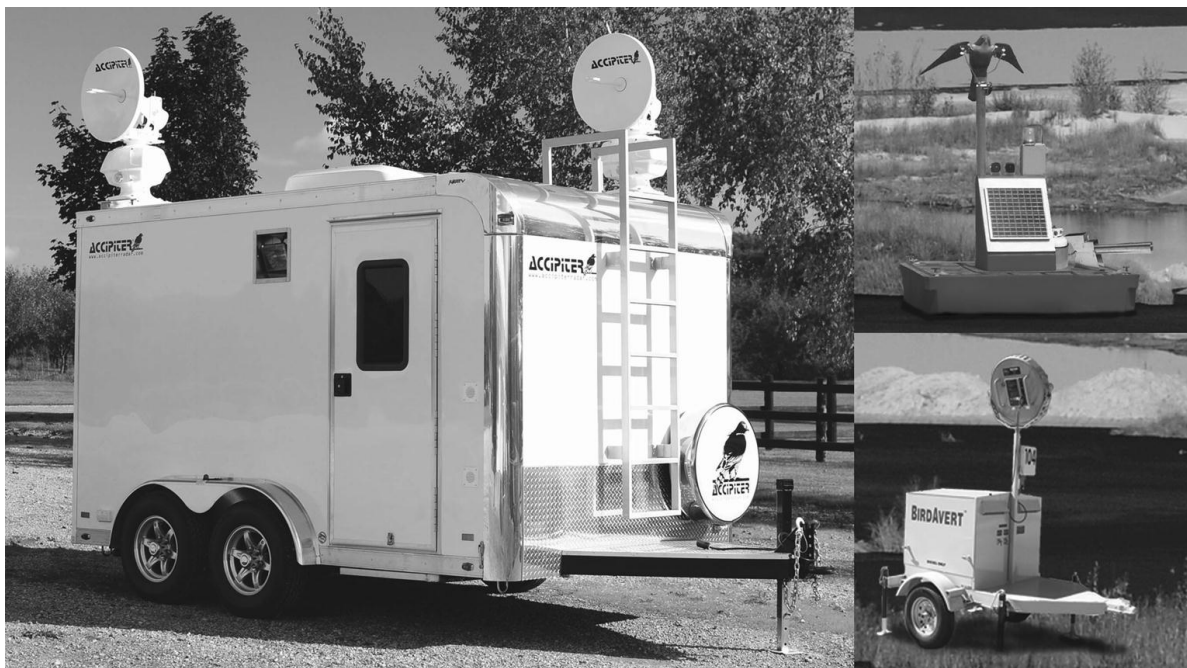
Figure 2. Radar-activated deterrent system subsystems: dual-radar trailer, floating deterrent, and HPAD deterrent.
