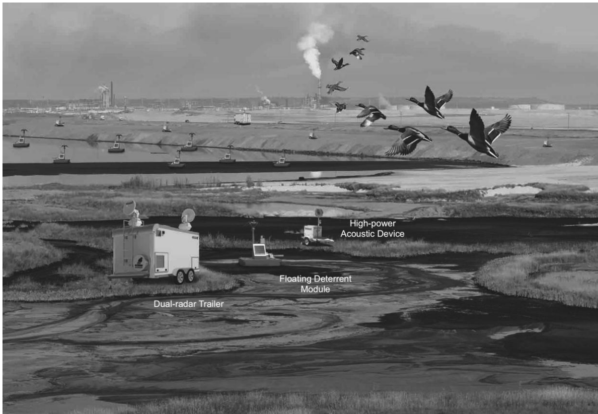
Figure 1. Illustration of radar-activated deterrent system protecting tailings pond showing a trailer with two X-band radars, shore-mounted high-power acoustic devices, and floating deterrent modules.
