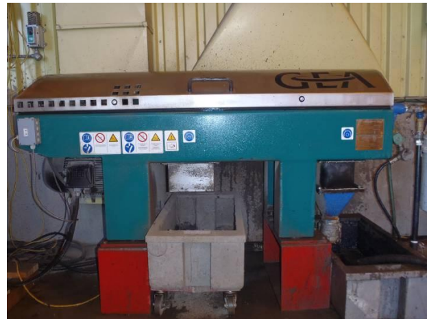
Figure 1. Photograph of GEA decanter centrifuge used in studies.
