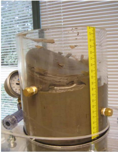
Figure 8. Shrinkage of the Oil Sands tailings from the walls of the column.
