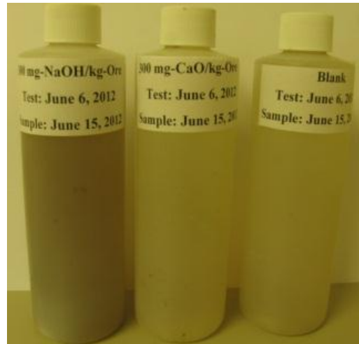
Figure 5. Extraction tailing, \text{CaO} and \text{NaOH} additives after 13 days.
