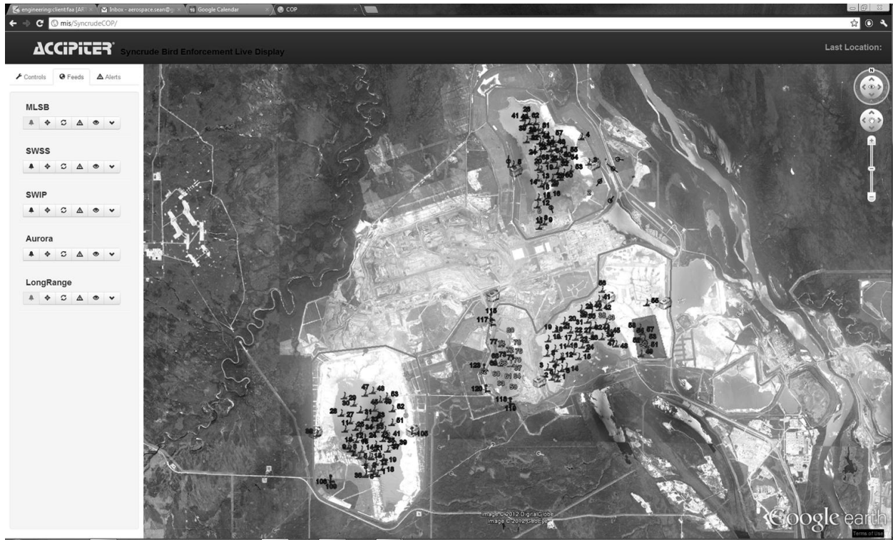
Figure 4. Common operating picture for real-time viewing and command and control of system. The symbols on the ponds represent floating deterrent modules.
