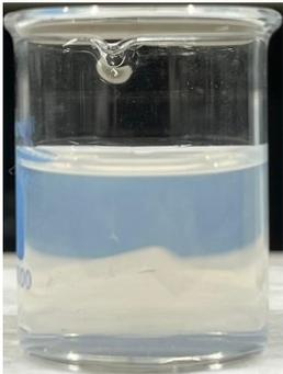
A glass beaker containing a blue liquid on top and a white precipitate at the bottom, representing the state after a reaction at 35 °C.   |
