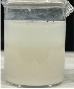
A glass beaker containing a white, opaque precipitate that has formed at the bottom of the liquid, representing the state after a reaction at 30 °C. |
