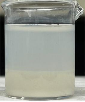
A glass beaker containing a blue liquid on top and a white precipitate at the bottom, representing the state after a reaction at 35 °C.              |
