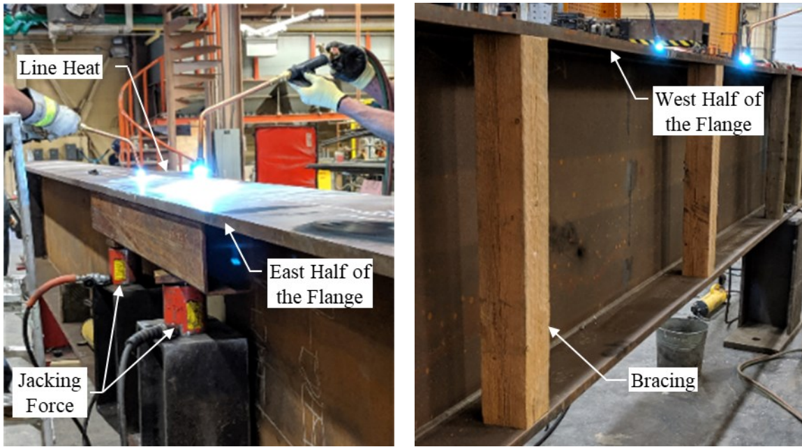
Figure 3-23: Line heat procedure performed on G8-390-25-2-p
