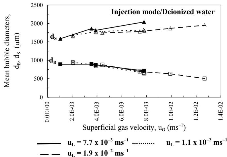
Figure 21. Effects of  $u_G$  and  $u_L$  on  $d_B$  and  $d_S$  in deionized water.
