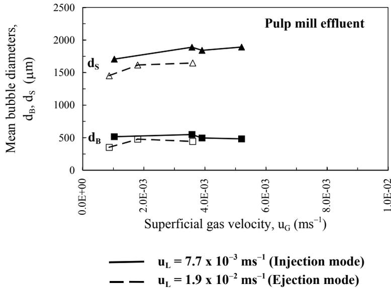
Figure 26. Effects of  $u_G$  and  $u_L$  on  $d_B$  and  $d_S$  in raw Kraft pulp mill effluent.
