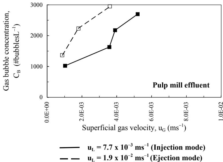
Figure 28. Effects of  $u_G$  and  $u_L$  on  $C_B$  in raw Kraft pulp mill effluent.
