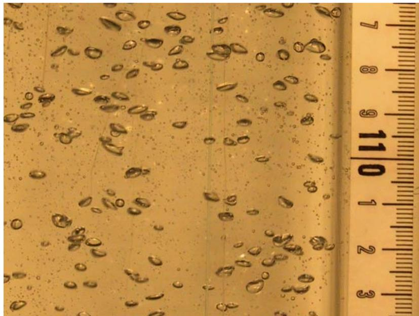
Figure 18. A digital image of the air bubbles at  $u_L = 7.7 \times 10^{-3} \text{ ms}^{-1}$  and  $u_G = 1.0 \times 10^{-3} \text{ ms}^{-1}$ .
