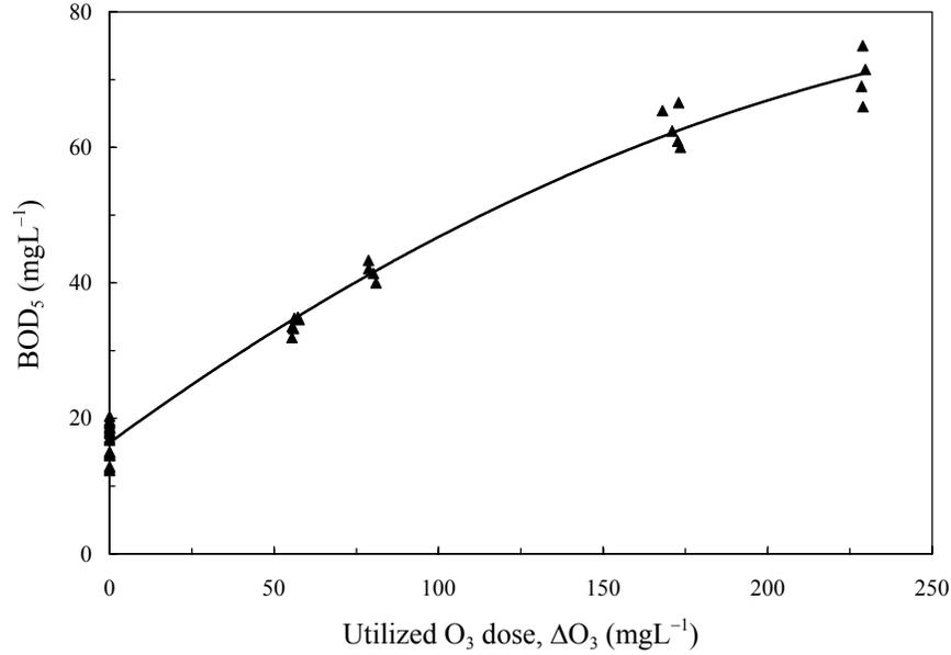
Figure 5. The effect of ozonation on the BOD<sub>5</sub> of the pulp mill wastewater treated in the extra-coarse-bubble diffuser ozone contactor.
