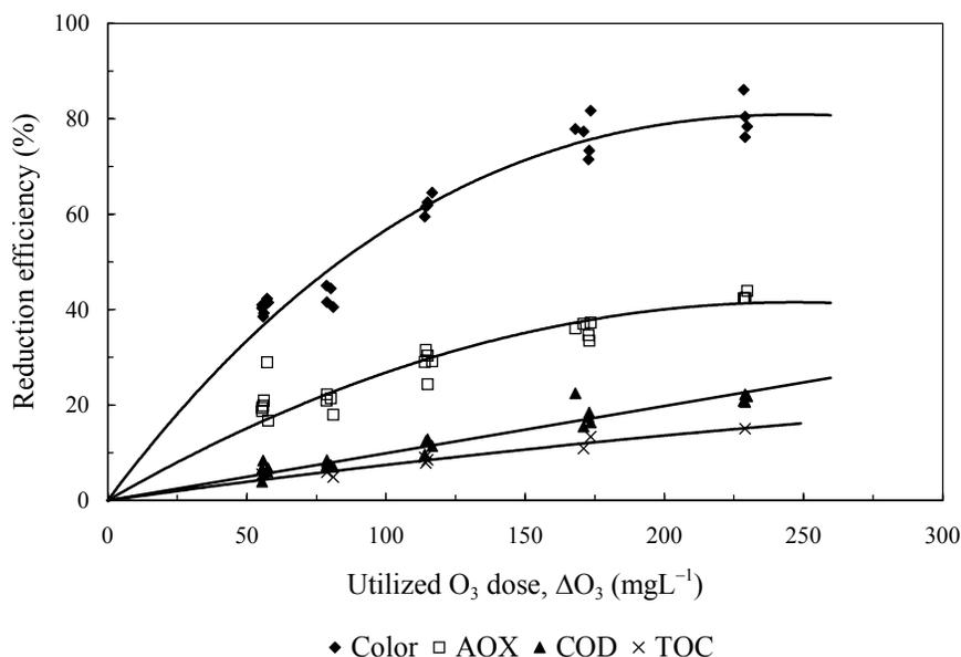
Figure 4. Reduction efficiencies of color, AOX, COD, and TOC in the extra-coarse-bubble diffuser ozone contactor.
