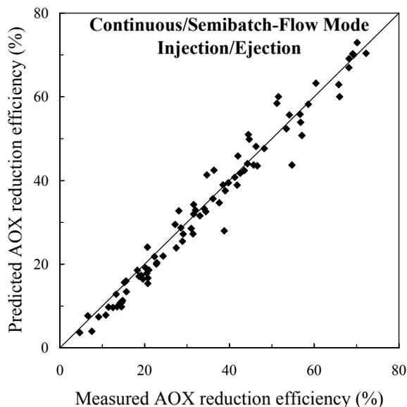
Figure 17. A comparison between the predicted and the measured reduction efficiencies of AOX.
