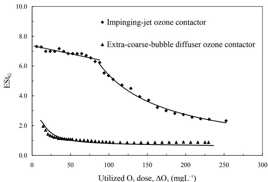
Figure 12. The effect of ozonation on the  $ES_{tG}$  values in two different ozone contactors operated in a semibatch-flow mode.
