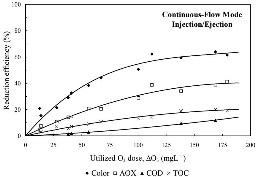
Figure 7. Reduction efficiencies of color, AOX, COD, and TOC in the impinging-jet ozone contactor operated in a continuous-flow mode.
