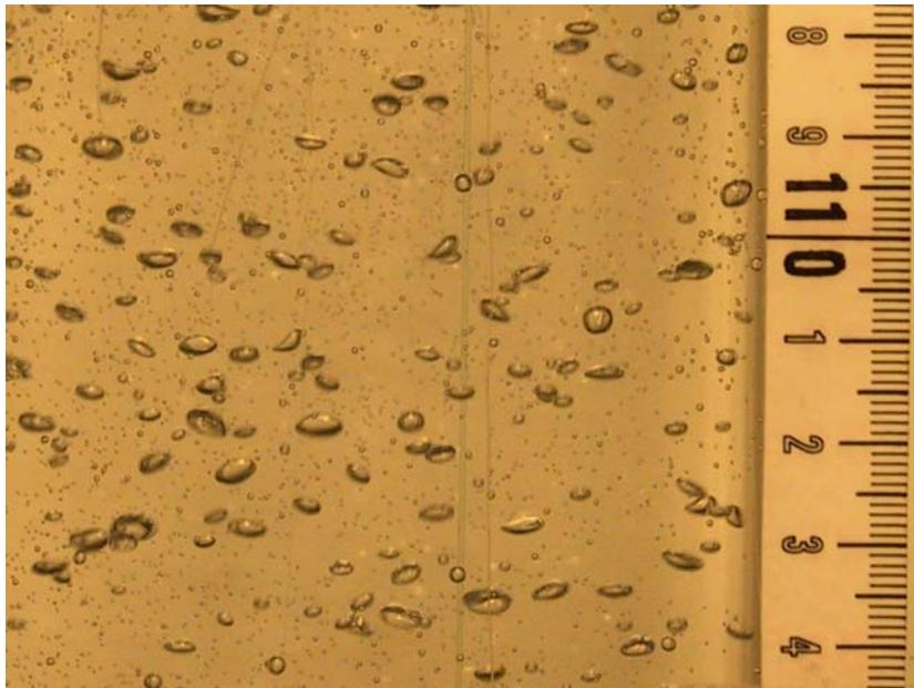
Figure 20. A digital image of the air bubbles at  $u_L = 1.9 \times 10^{-2} \text{ ms}^{-1}$  and  $u_G = 8.7 \times 10^{-4} \text{ ms}^{-1}$ .
