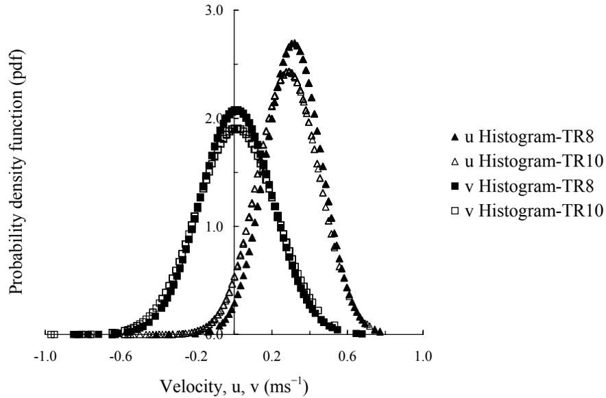
Figure 24. Typical probability density distributions of the gas-phase  $u$  and  $v$  in deionized water.
