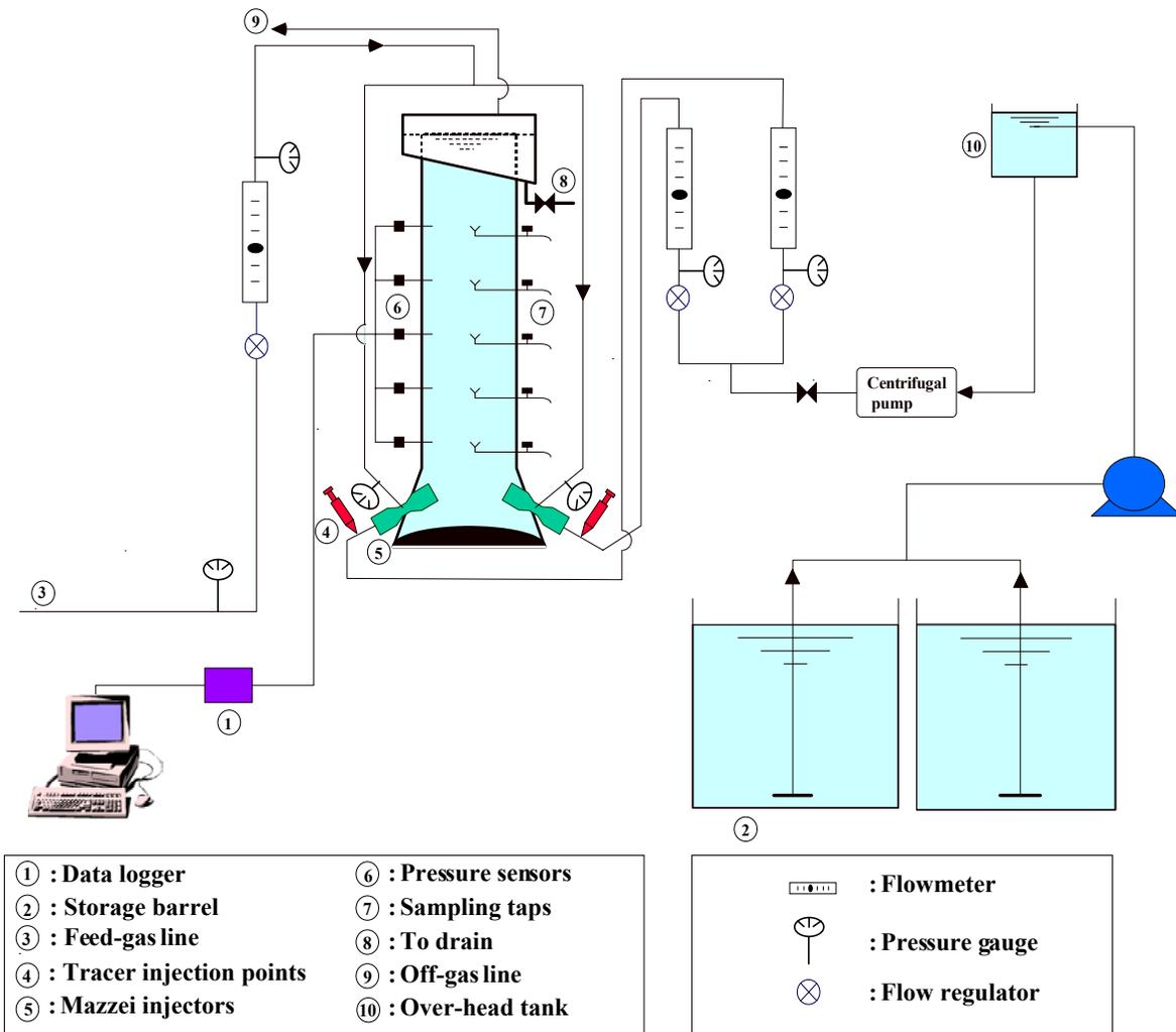
Figure 2. Schematic of the experimental set-up of the pilot-scale impinging-jet ozone contactor.
