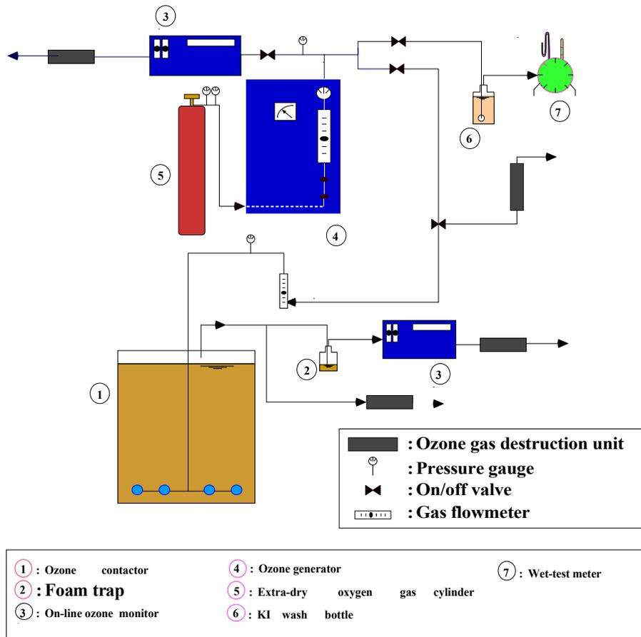
Figure 1. Schematic of the experimental set-up of the extra-coarse-bubble diffuser ozone contactor.
