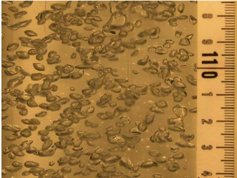
Figure 19. A digital image of the air bubbles at  $u_L = 7.7 \times 10^{-3} \text{ ms}^{-1}$  and  $u_G = 7.8 \times 10^{-3} \text{ ms}^{-1}$ .
