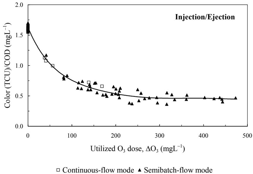
Figure 14. The effect of ozonation on the color/COD ratio of the treated Kraft pulp mill wastewater in the impinging-jet ozone contactor.
