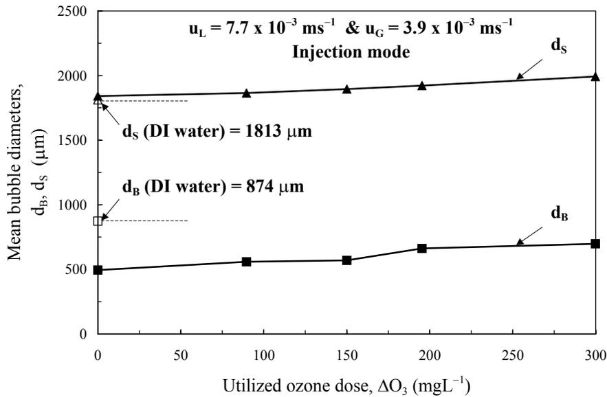
Figure 27. Effects of  $\Delta O_3$  on  $d_B$  and  $d_S$  in Kraft pulp mill effluent.
