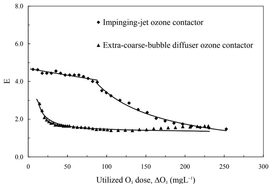
Figure 11. The effect of ozonation on the E values in two different ozone contactors operated in a semibatch-flow mode.
