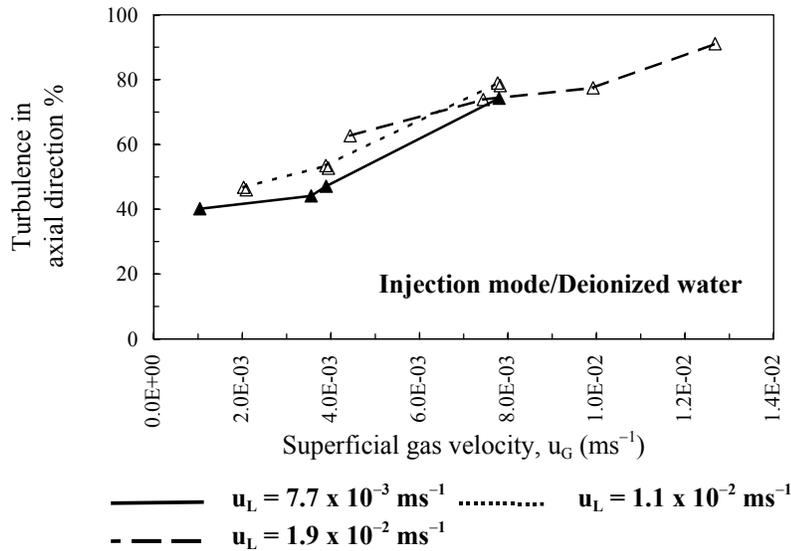
Figure 23. Effects of  $u_G$  and  $u_L$  on the gas-phase axial turbulence % in deionized water.
