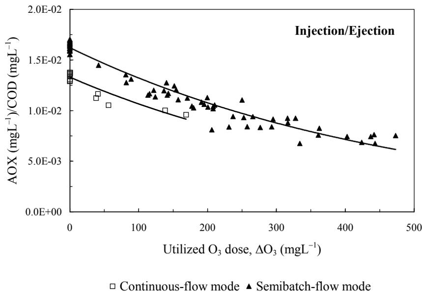
Figure 15. The effect of ozonation on the AOX/COD ratio of the treated Kraft pulp mill wastewater in the impinging-jet ozone contactor.
