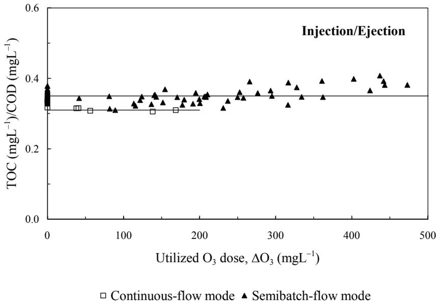
Figure 16. The effect of ozonation on the TOC/COD ratio of the treated Kraft pulp mill wastewater in the impinging-jet ozone contactor.
