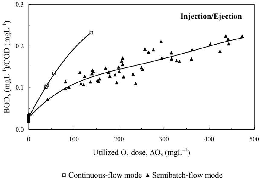
Figure 13. The effect of ozonation on the BOD<sub>5</sub>/COD ratio of the treated Kraft pulp mill wastewater in the impinging-jet ozone contactor.
