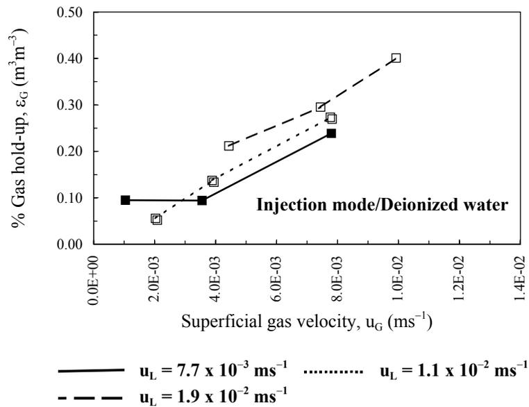
Figure 25. Effects of  $u_G$  and  $u_L$  on  $\epsilon_G$  in deionized water.
