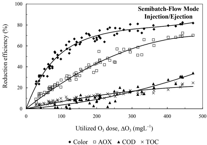
Figure 6. Reduction efficiencies of color, AOX, COD, and TOC in the impinging-jet ozone contactor operated in a semibatch-flow mode.
