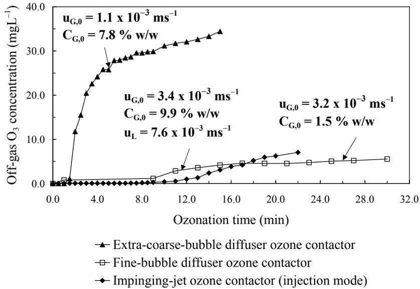
Figure 9. The effect of ozonation on the off-gas ozone concentration profiles in three different ozone contactors operated in a semibatch-flow mode.
