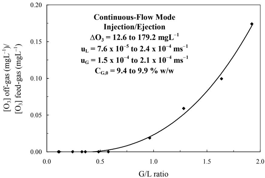
Figure 10. The effect of ozonation on the off-gas to the feed-gas ozone concentrations' ratio in the impinging-jet ozone contactor operated in a continuous-flow mode.
