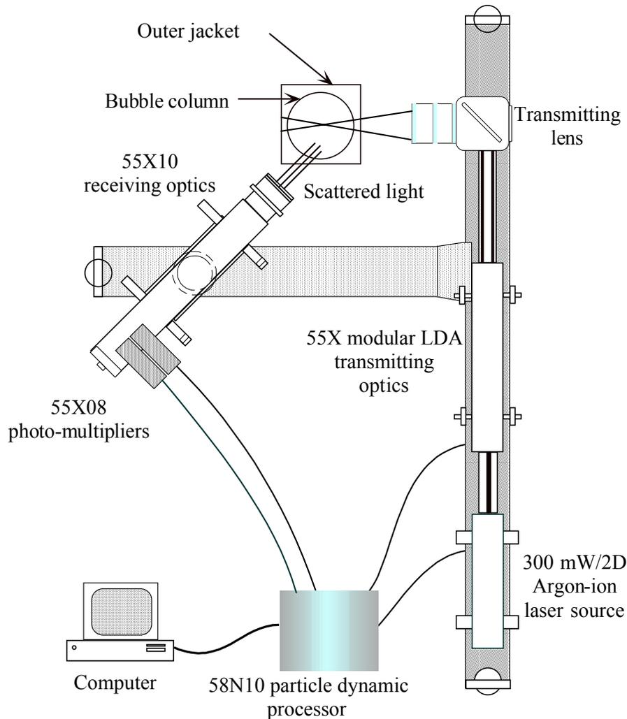
Figure 3. Components of the particle dynamics analyzer set-up (adapted from Shawwa 1998).
