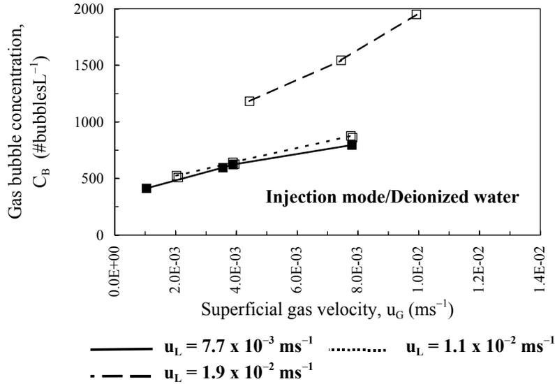
Figure 22. Effects of  $u_G$  and  $u_L$  on  $C_B$  in deionized water.
