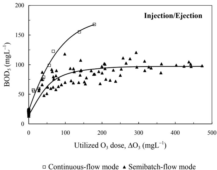
Figure 8. The effect of ozonation on the BOD<sub>5</sub> of the pulp mill wastewater treated in the impinging-jet ozone contactor.
