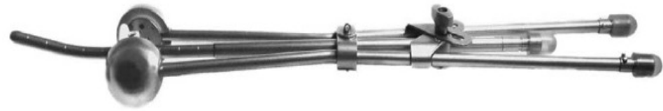
Figure 1-3. Tandem & ovoid applicators: (A) Manchester-style; (B) Fletcher LDR (lower part) and HDR (upper part) applicator (from Rownd 2005); (C) Henschke applicator (designed for Nucletron low-dose-rate Selectron afterloading system, from Thirion et al. 2005).
