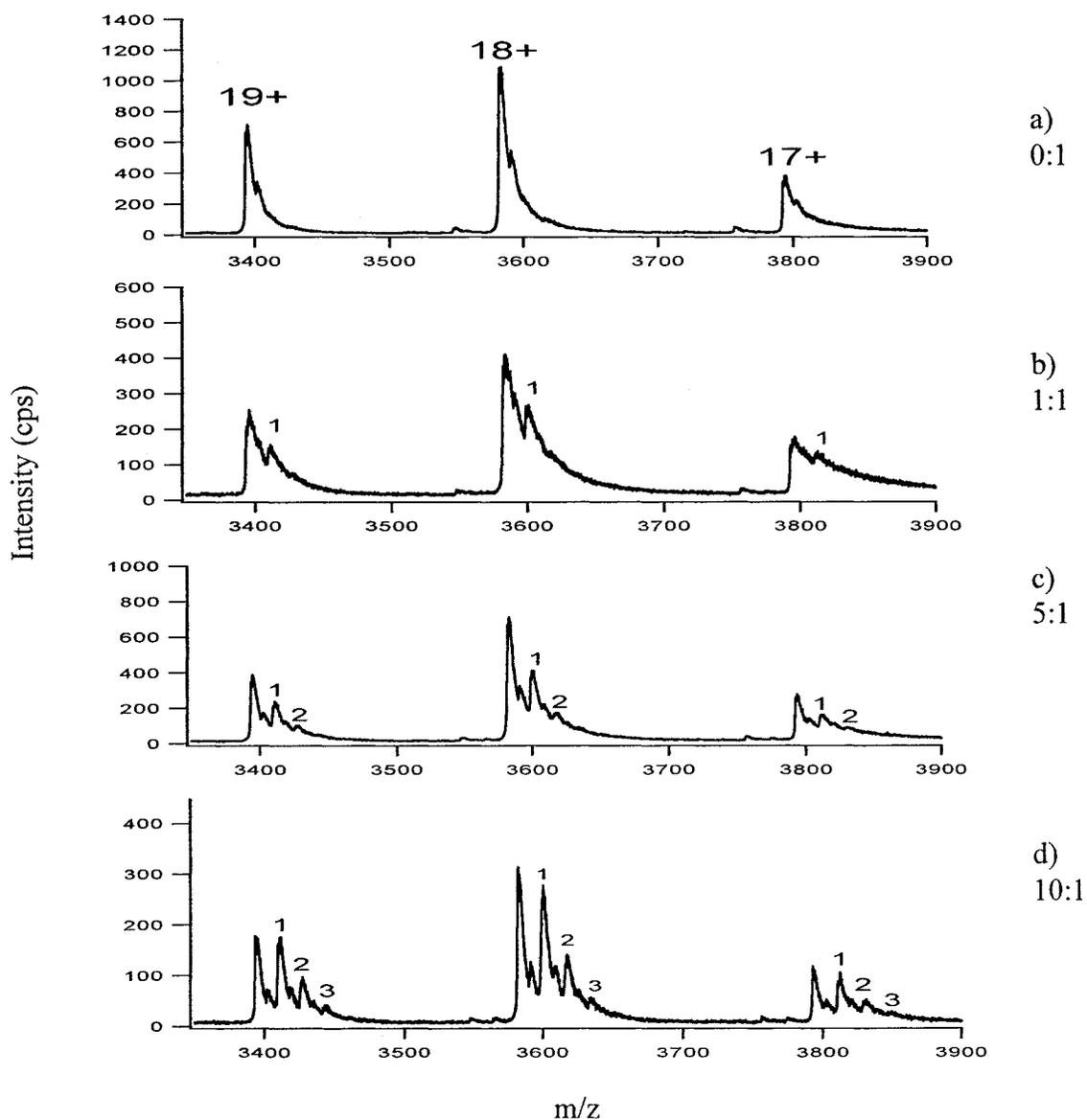
Figure 3.1 Typical nanoESI mass spectra of oxaliplatin-Hb complexes formed in reaction mixtures of oxaliplatin and Hb at oxaliplatin:Hb molar ratio of a) 0:1 , b) 1:1 , c) 5:1 , d) 10:1 . The reaction mixtures of oxaliplatin and Hb were incubated at 37 °C for 24 hours. The additional peaks labelled 1, 2, and 3 indicate three different Hb-drug complex species.
