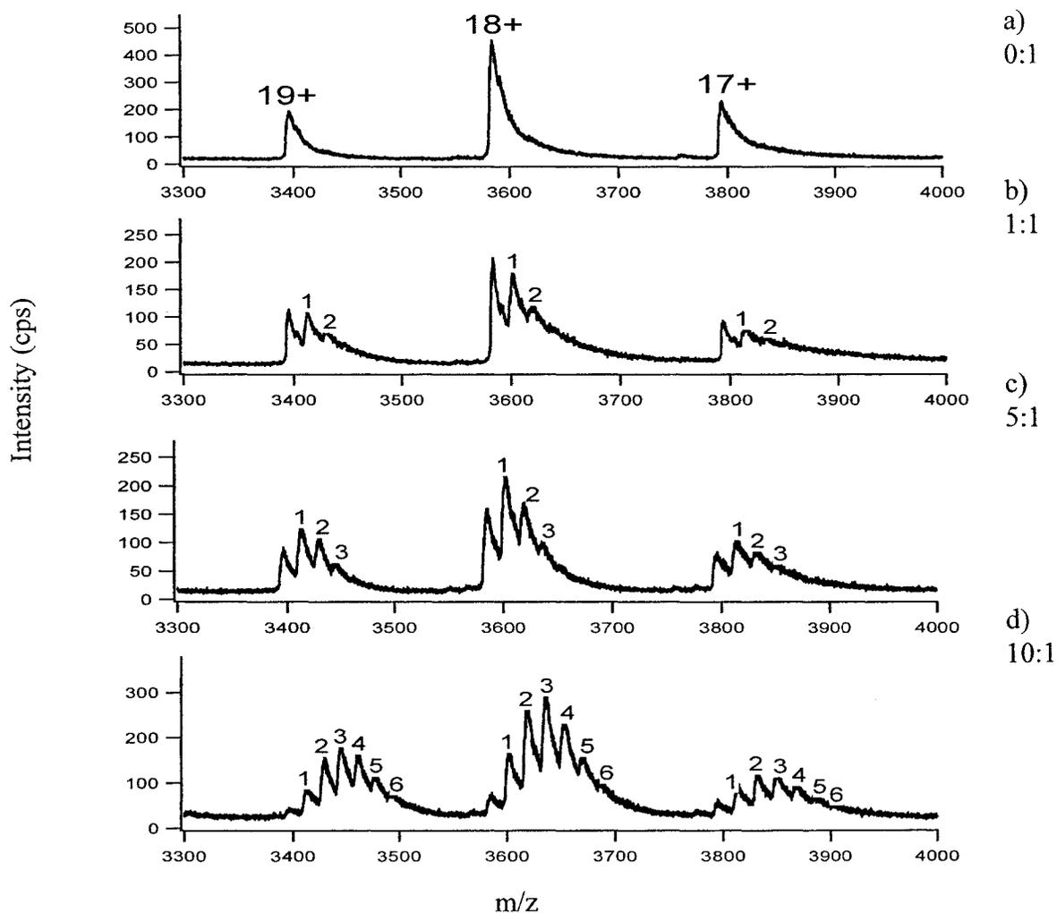
Figure 3.3 Typical nanoESI mass spectra of oxaliplatin-Hb complexes formed in reaction mixtures of oxaliplatin and Hb at oxaliplatin:Hb molar ratio of a) 0:1, b) 1:1, c) 5:1, and d) 10:1. The reaction mixtures were incubated at 37°C for 5 days. The peaks labelled 1, 2, 3, 4, 5, and 6 indicate the different species of Hb-1drug, Hb-2drug, Hb-3drug, Hb-4drug, Hb-5drug and Hb-6drug complex, respectively.
