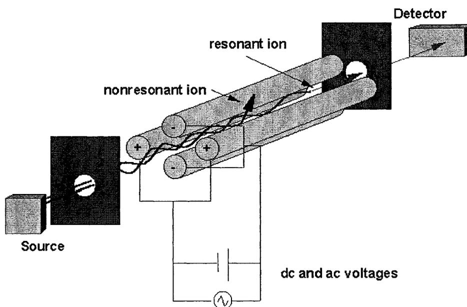
Figure 1.5 Schematic diagram of a quadrupole mass filter.
