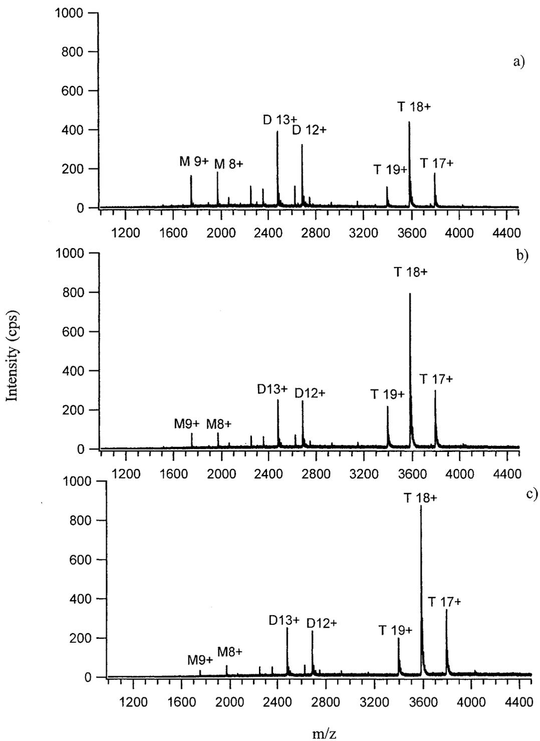
Figure 2.5 Mass spectra of 10  $\mu$ M Hb in 5 mM ammonium acetate buffer using different CAD values: a) CAD 2, b) CAD 5, c) CAD 7. T = Hb tetramer; D = Hb dimer; M = Hb monomer
