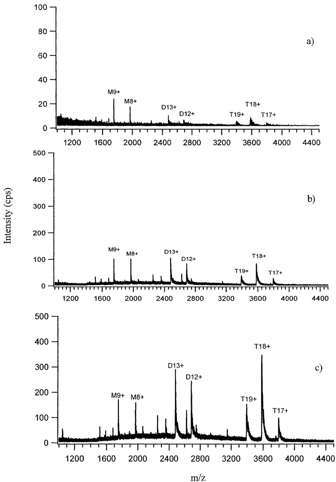
Figure 2.3 NanoESI mass spectrum of 10  $\mu$ M Hb in 5 mM ammonium acetate buffer using three different CE values: a) CE 11 eV, b) CE 4 eV, c) CE 3 eV. T = Hb tetramer; D = Hb dimer; M = Hb monomer
