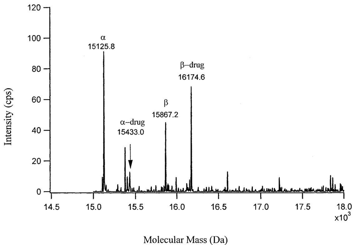
Figure 3.6 Partial deconvoluted product ion spectrum of precursor ion  $m/z$  2714 (from molecular mass 14500 to 18000 Da). The molecular mass of  $\alpha$ -chain and  $\alpha$ -drug is 15125.8 and 15433.0 Da, respectively, and the mass difference is 307.2 Da. The molecular mass of  $\beta$ -chain,  $\beta$ -drug is 15867.2 and 16174.6 Da, respectively, and the mass difference is 307.4 Da.
