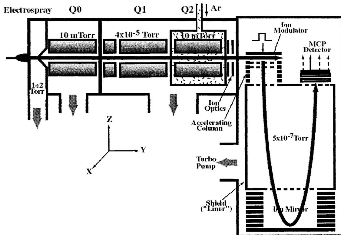
Figure 1.6 Diagram of the quadrupole/time-of-flight mass spectrometer (Applied Biosystems/MDS Sciex).
