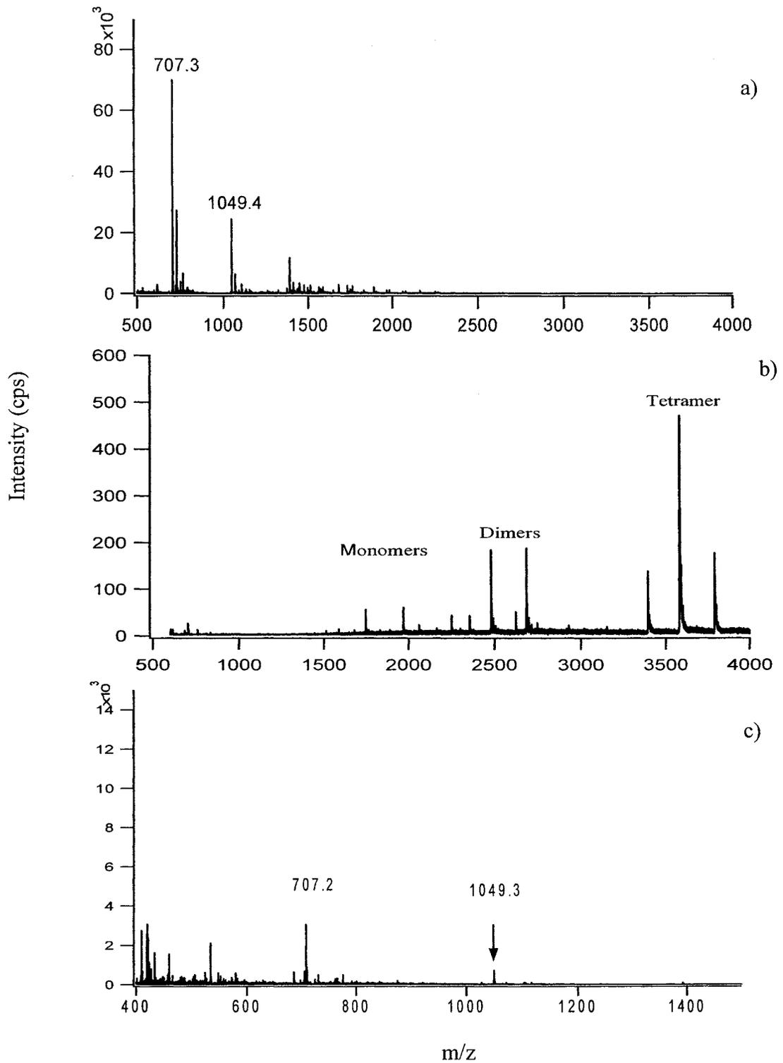
Figure 2.2 a) NanoESI mass spectrum of 10  $\mu$ M Hb without desalting, b) nanoESI mass spectrum of 10  $\mu$ M Hb after desalting, c) nanoESI mass spectrum of the filtrate (the fraction of molecular mass less than 10 kDa) using a Microcon YM-10 centrifugal filter.
