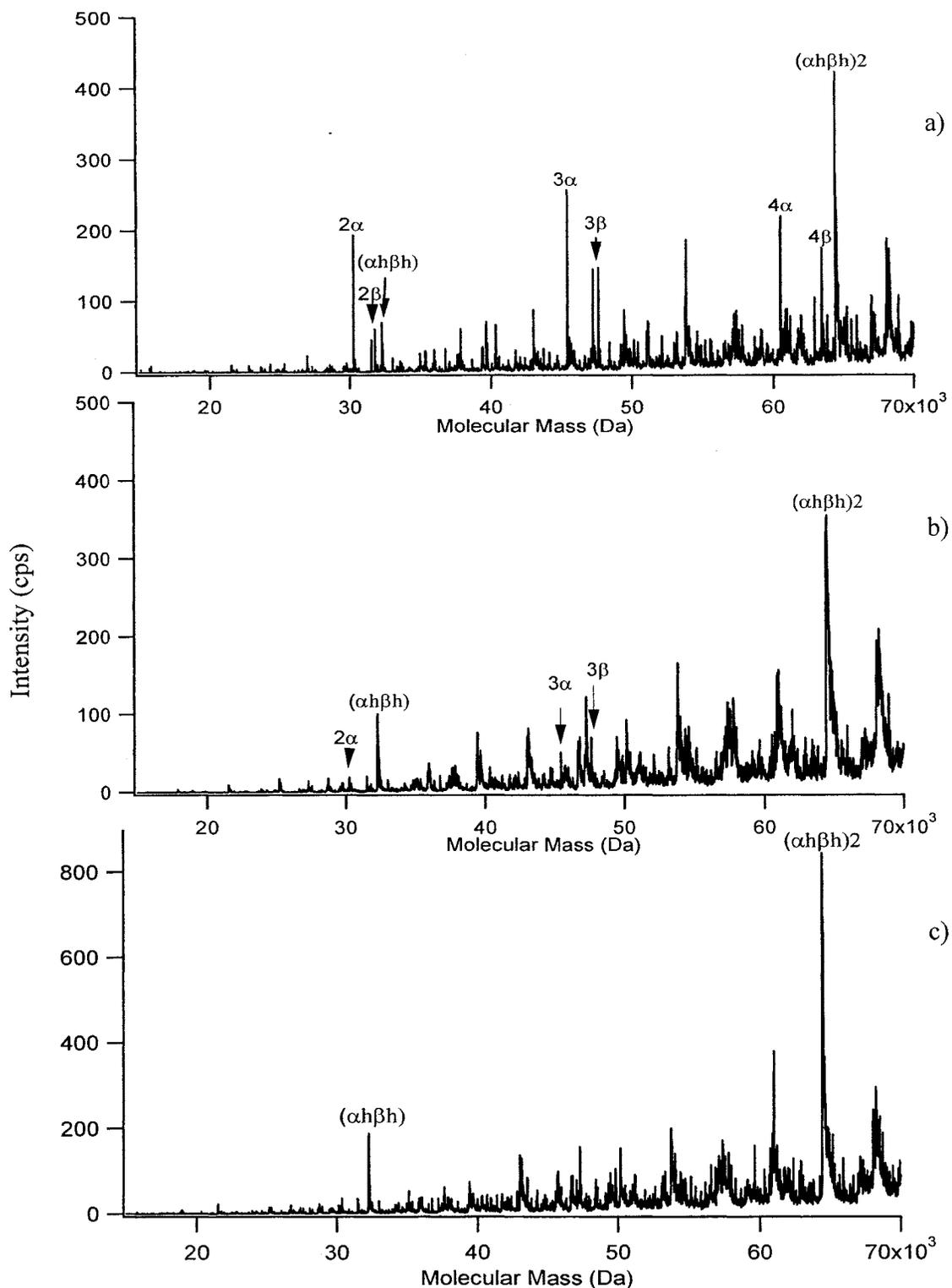
Figure 2.4 Deconvoluted mass spectrum of 10  $\mu\text{M}$  Hb in 5 mM ammonium acetate using three different DP1 and FP values: a) DP1 65, FP 215; b) DP1 45, FP 180; c) DP1 30, FP 150.  $(\alpha\text{h}\beta\text{h})_2$  represents the intact heme-bound tetramer;  $(\alpha\text{h}\beta\text{h})$  represents the heme-bound dimer;  $\alpha$ ,  $\beta$  represent the  $\alpha$ -globin chain and  $\beta$ -globin chain, respectively.
