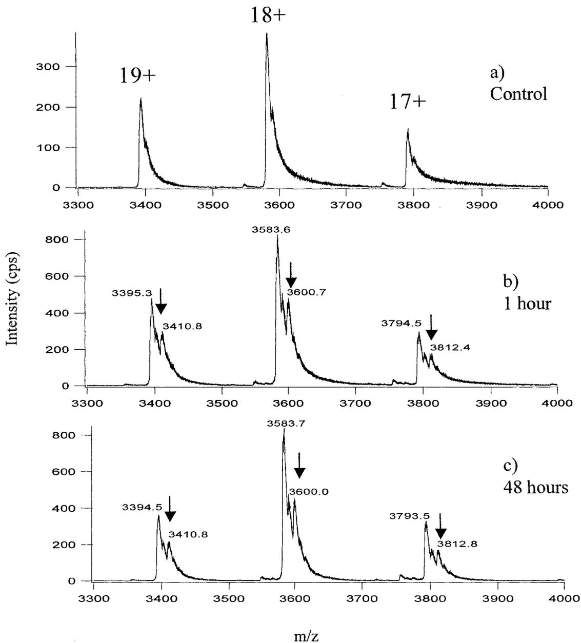
Figure 3.10 NanoESI mass spectra of Hb-oxaliplatin complexes in RBCs hemolysate from a cancer patient's blood sample: a) normal control; b) collected 1 hour after infusion; c) collected 48 hours after infusion.
