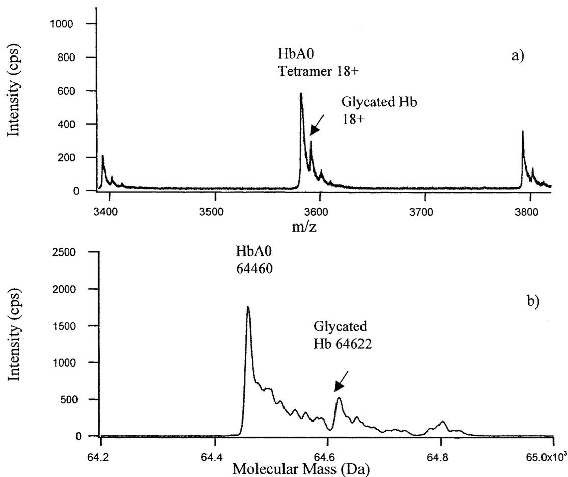
Figure 2.6 a) NanoESI mass spectrum of 10  $\mu$ M HbA0 in 5 mM aqueous ammonium acetate buffer in the mass range 3300-3900 m/z; b) deconvoluted mass spectrum of HbA0 and glycated Hb.
