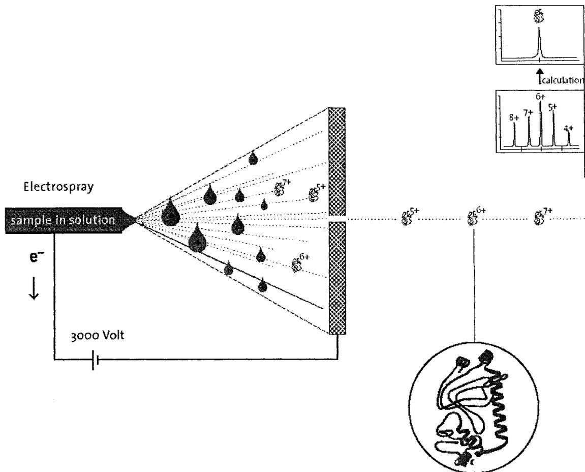
Figure 1.4 Diagram of how ESI-MS analyzes a protein sample.
