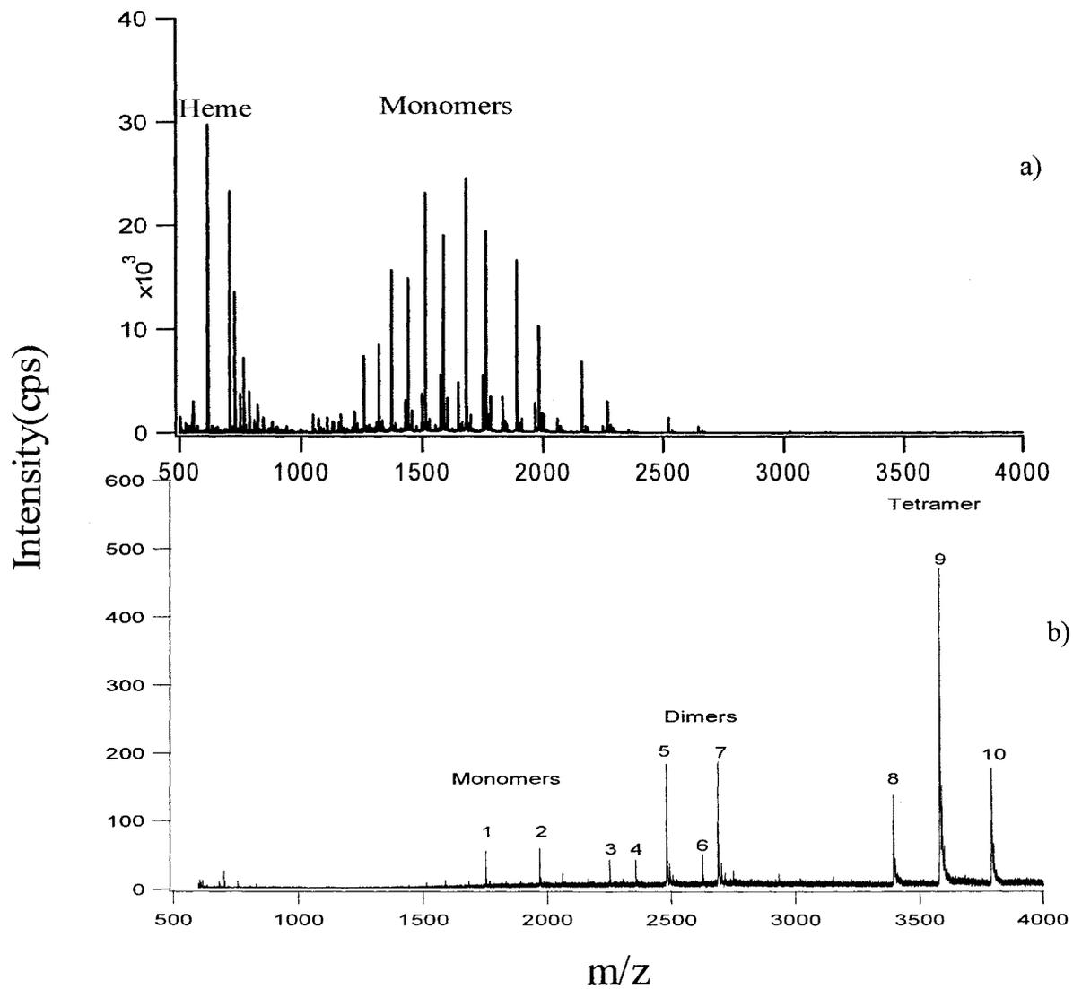
Figure 2.1 Typical nanoESI mass spectrum of 10  $\mu$ M Hb in: a) 10% methanol solution containing 0.01% formic acid (pH 4), b) 5 mM aqueous ammonium acetate buffer (pH 6.5).
