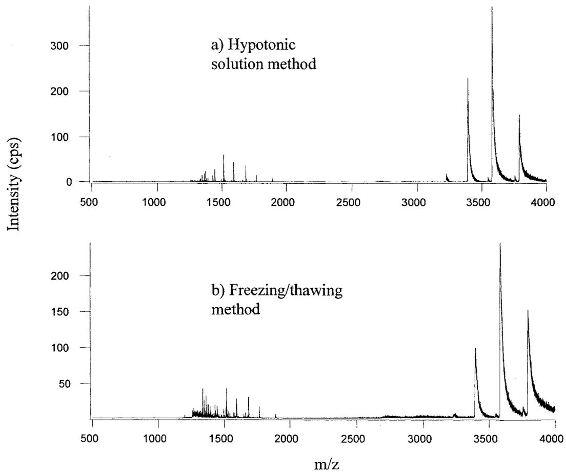
Figure 3.9 NanoESI mass spectra of the hemolysate of RBCs from one healthy volunteer using two lysing methods: a) hypotonic solution method and b) freezing/thawing method.
