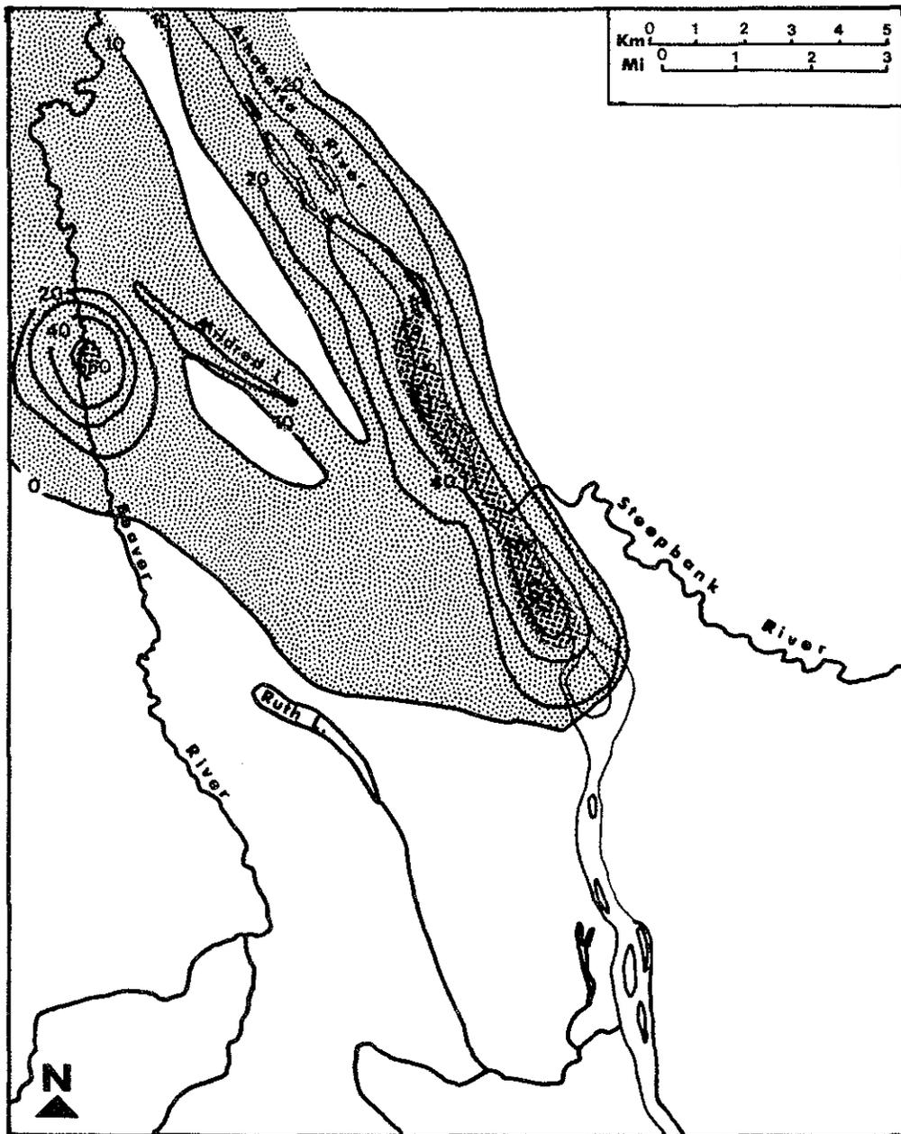
Figure 11. Estimated areal coverage of ground level fog during fog event of 9 January 1977. Information derived from sketches made by an aircraft observer. Light shading indicates fog depth of more than 10 m but less than 50 m. Heavy shading represents those areas estimated to have fog heights greater than 50 m.
