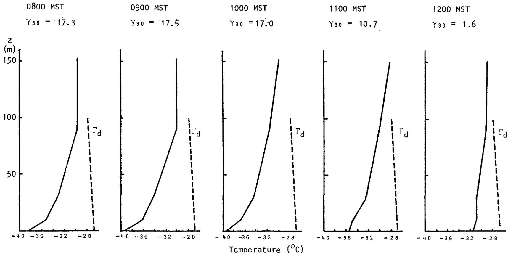
Figure 10. Hourly temperature profiles from data collected at the meteorological tower for 9 January 1977.  $\gamma_{30}$  is the temperature gradient from the 1.5 m to the 30 m level.  $\Gamma_d$  is the dry adiabatic lapse rate.
