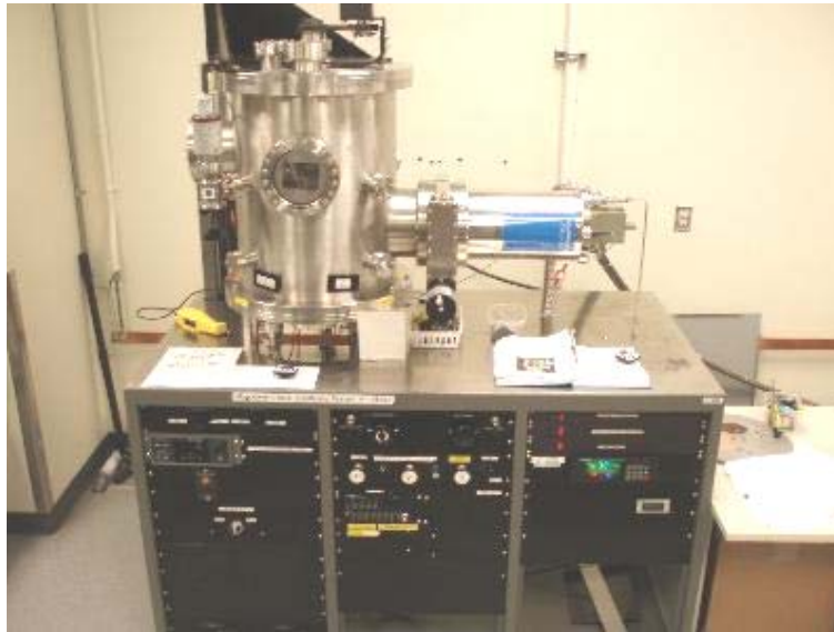
Figure 3.4 Sputtering system BOB
