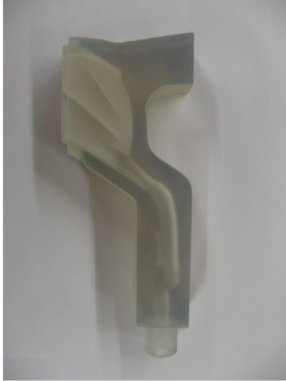
Figure 6: VeroClear throat with detachable VeroWhite septum.
