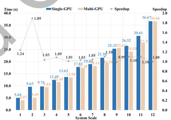
Fig. 14: Performance of the multi-GPU implementations.
