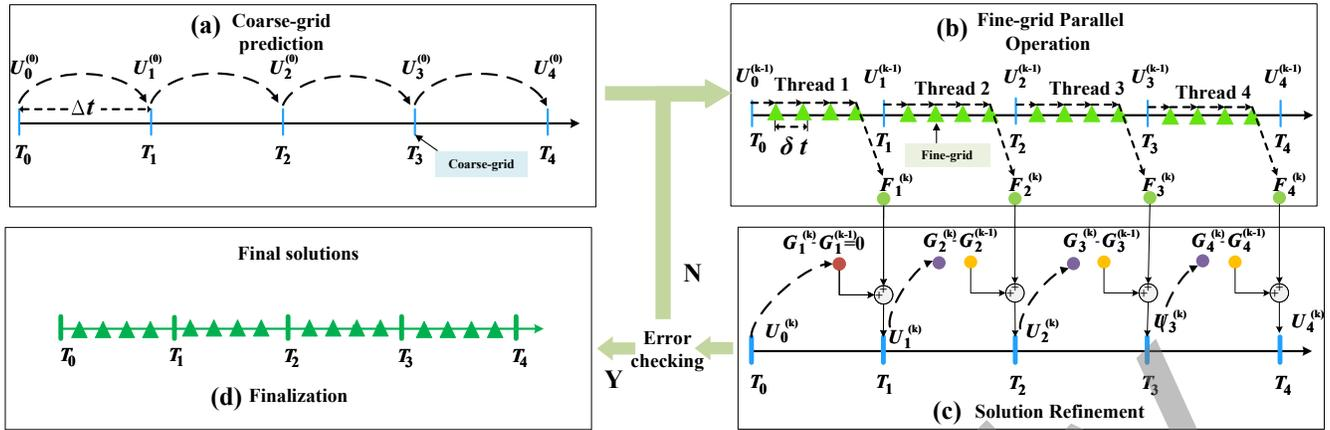
Fig. 5: Sequence of operations in the Parareal algorithm: (a) Initialize  $U_j^{(0)}$  which equals to  $G_j^{(0)}$ ; (b) Produce fine-grid solution  $F_j^k$ ; (c) Refine  $U_j^{(k)}$  with  $U_j^{(k)} = G_j^{(k)} + F_j^k - G_j^{(k-1)}$ , then continue (b) to start a new iteration.
