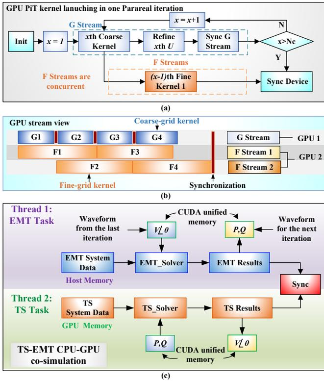
Fig. 9: Algorithm implementations of the PiT+PiS hybrid CPU-GPU TS-EMT co-simulation: (a) GPU PiT kernel launching within one Parareal iteration; (b) kernel execution graph in multi-stream/multi-GPU scenarios; (c) PiT+PiS TS-EMT co-simulation on hybrid CPU-GPU platform.
