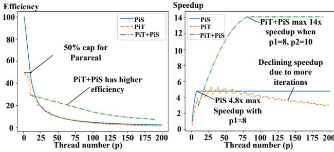
Fig. 6: Theoretical performance comparisons of PiS, PiT and PiT+PiS methods: (a) theoretical parallel efficiency; (b) theoretical speedup.
