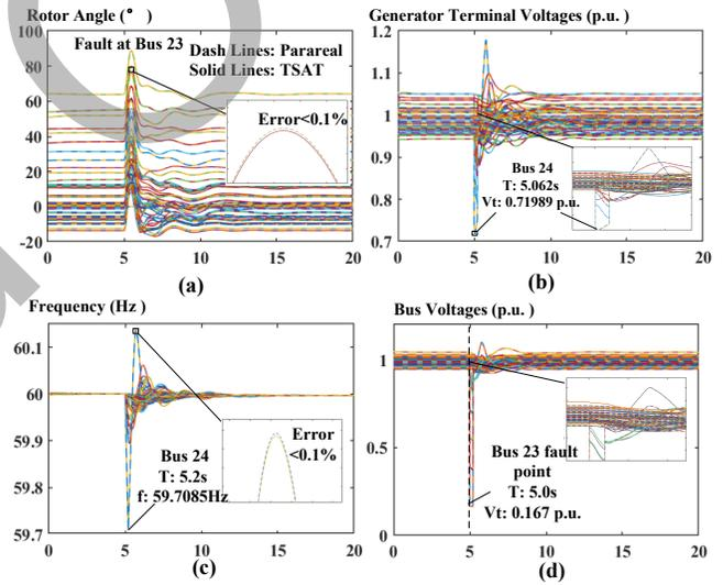
Fig. 11: Waveform of Case 1 test system: (a) generator rotor angles; (b) terminal voltages of all generators; (c) frequencies of all generators.
