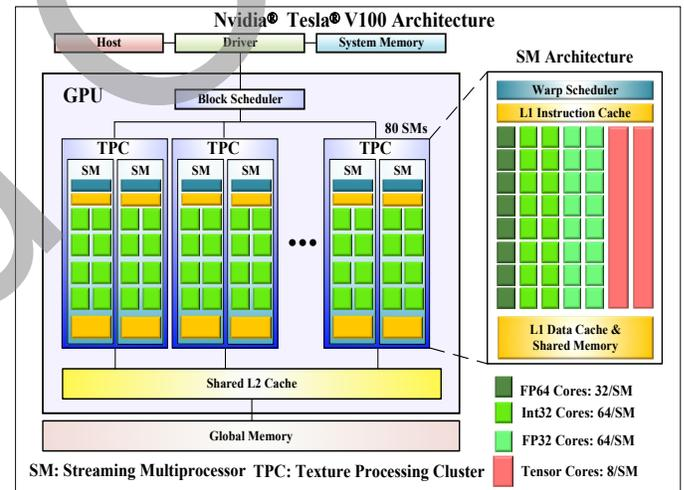
Fig. 8: General architecture of NVIDIA<sup>®</sup> Volta GPUs.
