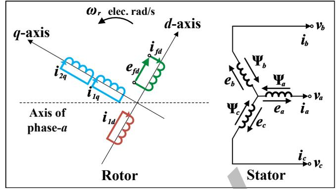
Fig. 1: Rotor and stator circuits of a Model 2.2 synchronous machine.
