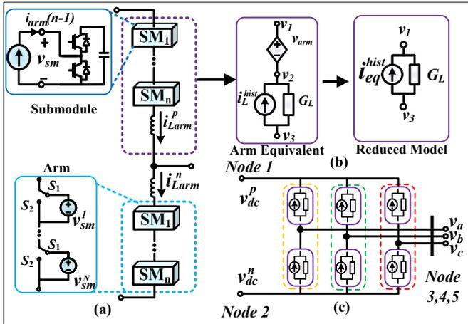
Fig. 4: Three-phase MMC model: (a) the MMC arm submodules are equivalent to a series of voltage sources; (b) the choke inductor can be merged to omit one internal node; (c) the final MMC equivalent circuit in the main circuit.
