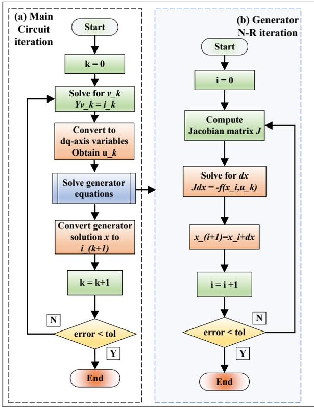
Fig. 3: Transient stability simulation process: (a) loop for solving voltages in main circuit; (b) loop for solving generator state variables.
