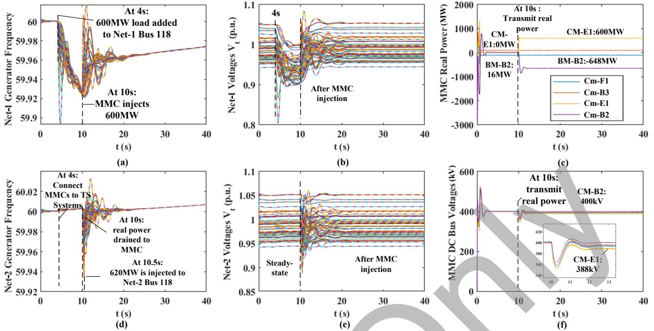
Fig. 12: Waveforms of Study Case 2: (a) Frequencies of the generators in Net-1; (b) Terminal Voltages of the generators in Net-1; (c) Real power of 4 MMCs; (d) Frequencies of the generators in Net-2; (e) Terminal Voltages of the generators in Net-2; (f) DC Voltages of four MMC terminals.
