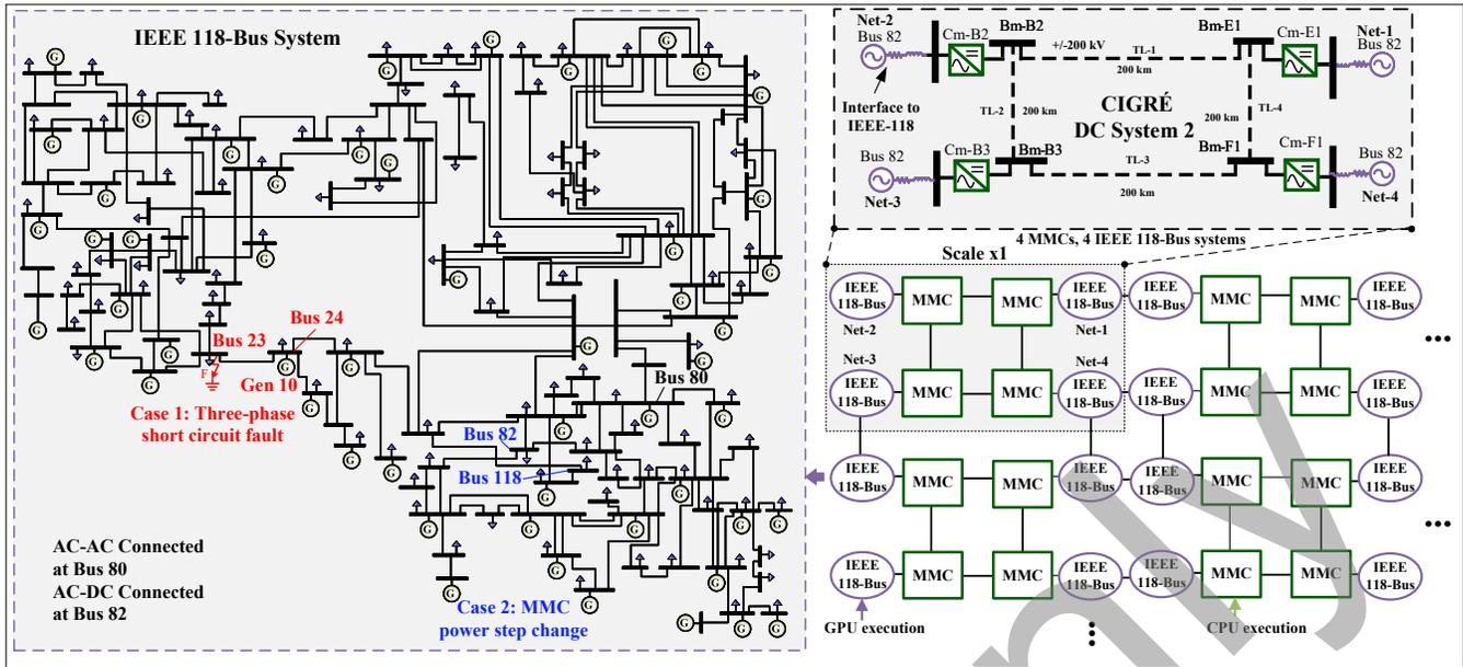
Fig. 10: Synthetic system for case studies and performance evaluations.
