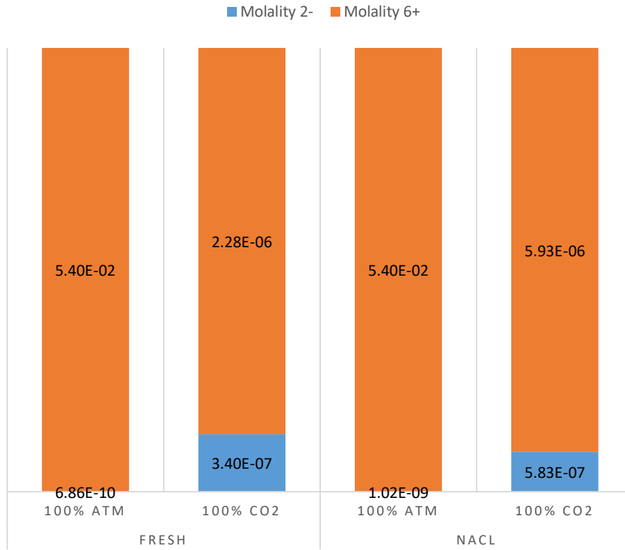
Figure D-1: Modelled speciation and molality of leached sulfur during experiments with Core 2 under atmospheric headspace conditions and 100 % CO 2 headspace, so simulate an anoxic environment.
