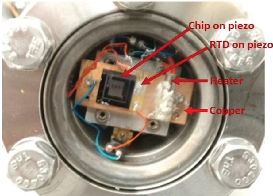
Figure 6.8: **A photo of the front-view of the measurement chamber.** The chip is glued by Ag epoxy on the piezo surface. RTD sensor close to chip also glued by the same epoxy on the piezo. The piezo shaker containing the chip and RTD sensor was further glued on a copper plate. The resistive heater is placed on the copper by epoxy.
