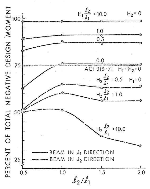
FIGURE 5.10 NEGATIVE COLUMN-STRIP MOMENT, INTERIOR PANEL,
