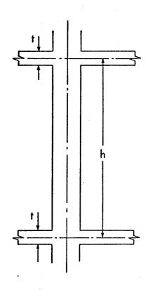
Stiffness of the column is  $K_{c} = k_{c} \frac{E_{c}I_{c}}{h}$
