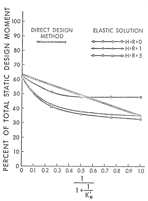
FIGURE 5.5 POSITIVE DESIGN MOMENT, EXTERIOR PANEL
