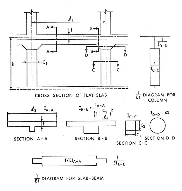
FIGURE 3.2 CROSS-SECTIONS FOR CALCULATING STIFFNESSES OF EQUIVALENT FRAME
