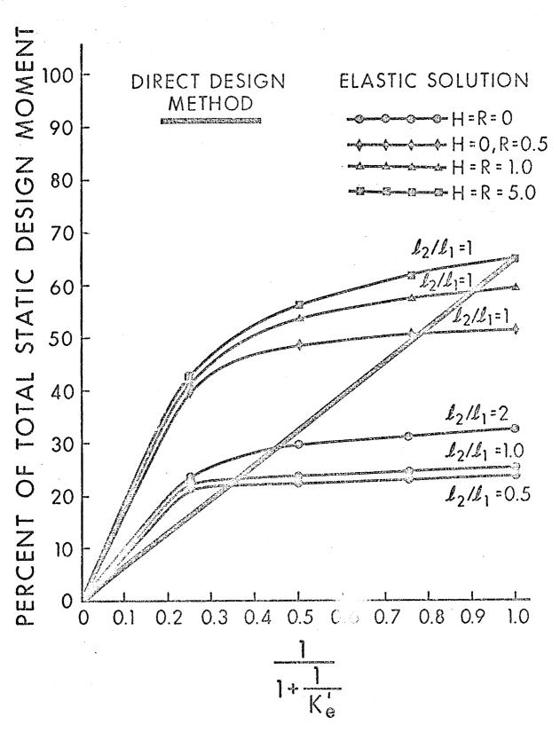
FIGURE 5.4 EXTERIOR NEGATIVE DESIGN MOMENT, EXTERIOR PANEL
