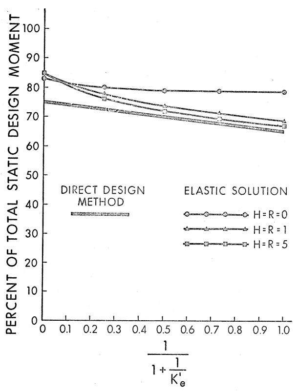
FIGURE 5.3 INTERIOR NEGATIVE DESIGN MOMENT, EXTERIOR PANEL
