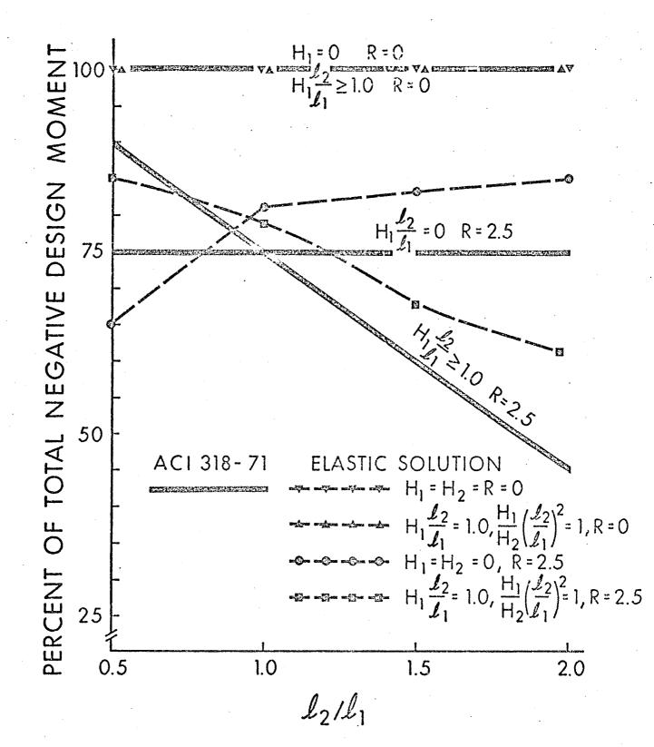
FIGURE 5.15 NEGATIVE COLUMN-STRIP MOMENT, EXTERIOR PANEL
