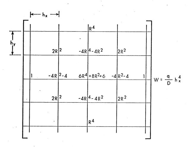
FIGURE B.3 FINITE DIFFERENCE PATTERN
