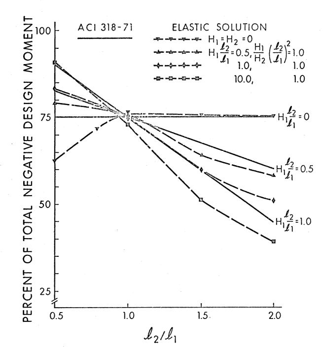
FIGURE 5.13 NEGATIVE COLUMN-STRIP MOMENT, INTERIOR PANEL
