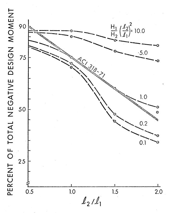
FIGURE 5.14 NEGATIVE COLUMN STRIP MOMENT, INTERIOR PANEL,  $H_1 \ell_2 / \ell_1 = 1$
