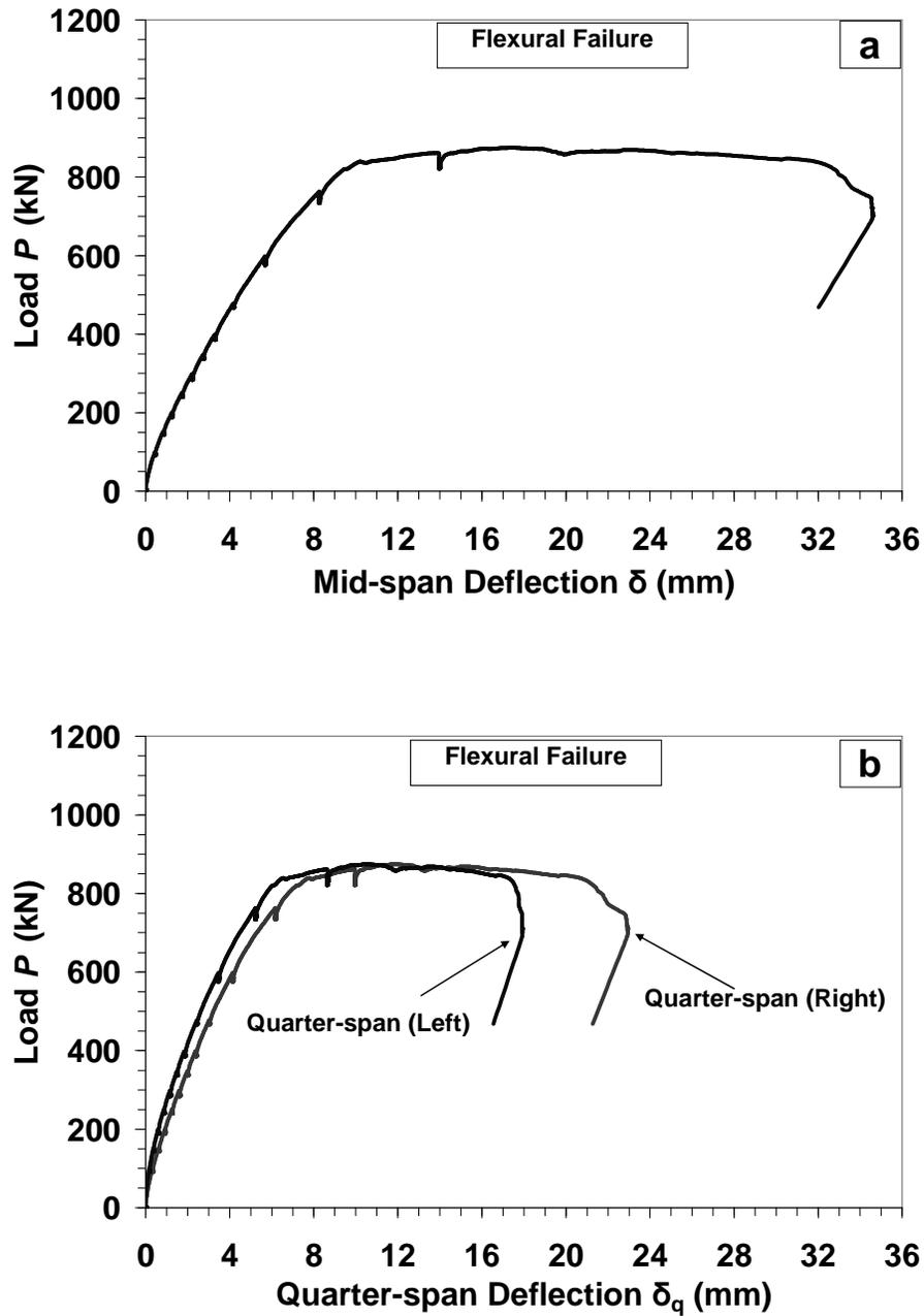
Figure B-34: Load-Deflection response for specimen *H61* at (a) mid-span; (b) quarter-span. (Note: all presented deflection data were corrected for the measured support settlement)
