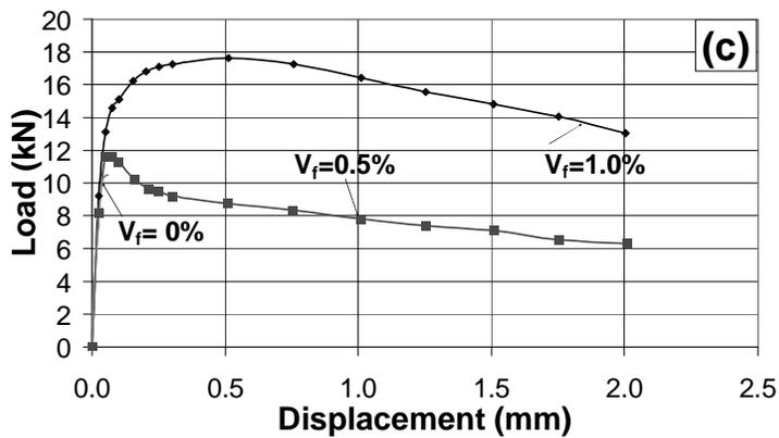
Figure 4-2: Representative Flexural Response of a) Normal Strength Regular Concrete; b) Lightweight concrete and c) High Strength Concrete.
