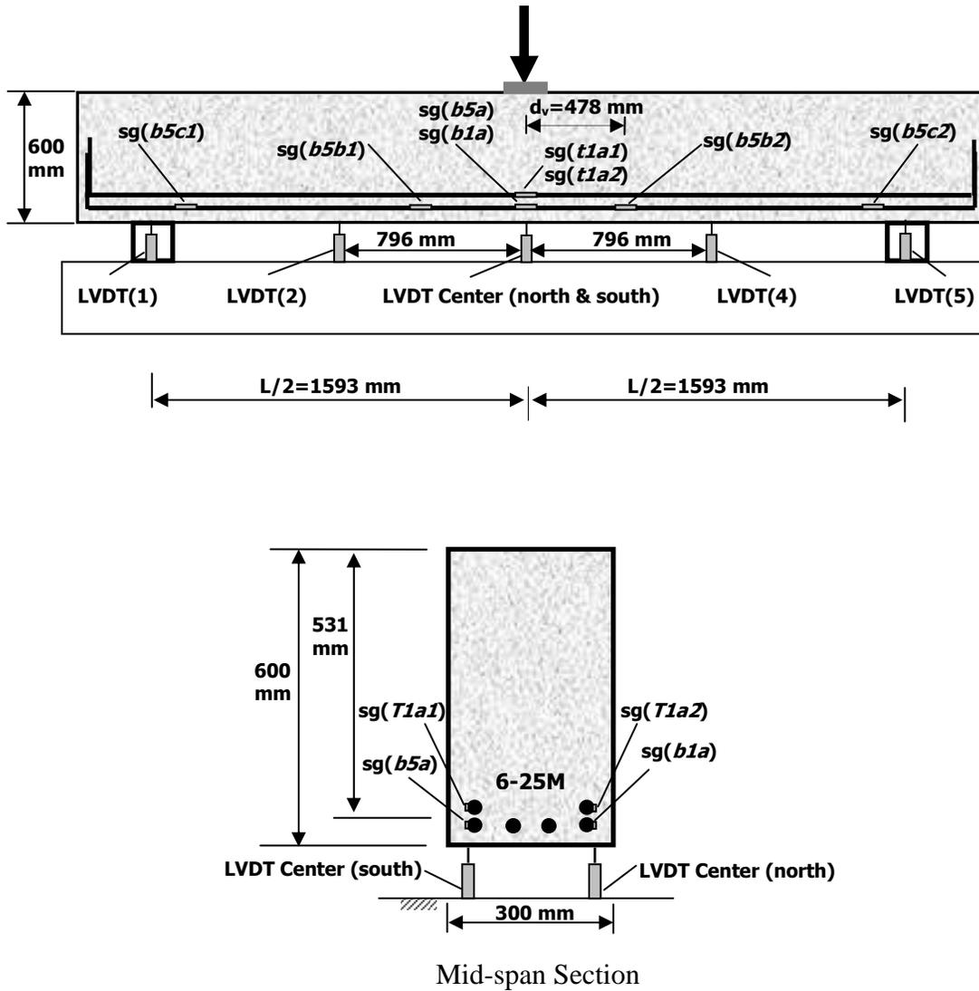
Figure B-33: Instrumentation for specimen *H61* (sg: strain gauge).
