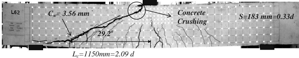
Figure 8-6: Crack patterns after shear failure for specimen *L62* with  $h = 600 \text{ mm}$ ,  $f'_c = 30 \text{ MPa}$ , and  $\rho = 1.21 \%$ . Size of grid on the specimen surface is  $100 \text{ mm}$ .
