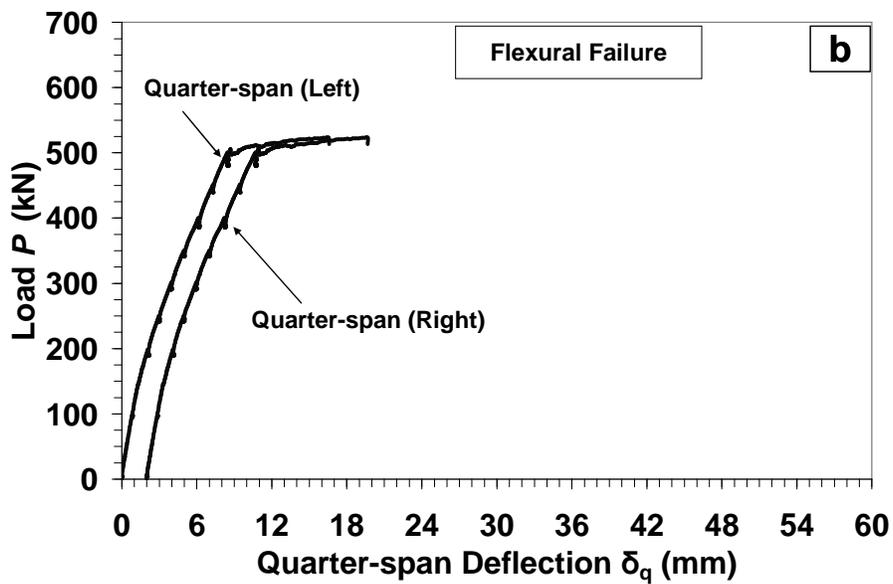
Figure B-66: Load-Deflection response for specimen *L10-1* at (a) mid-span; (b) quarter-span. (Note: all presented deflection data were corrected for the measured support settlement)
