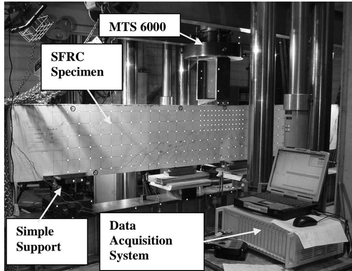
Figure 5-8: SFRC specimen *L61* under loading during test
