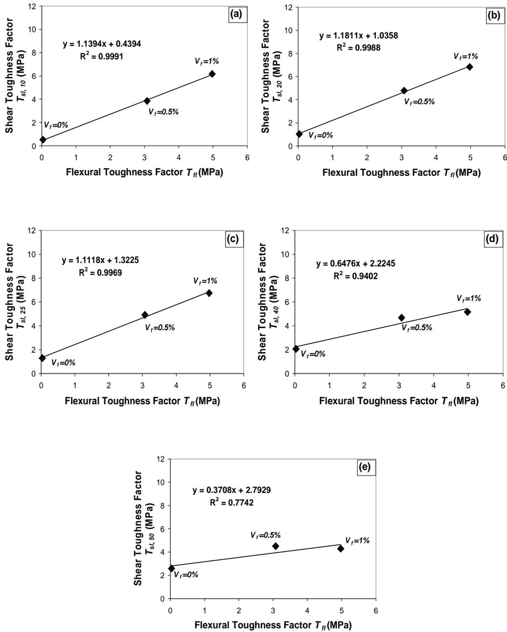
Figure 4-11: Correlation between the Flexural and Shear Toughness Factors of Lightweight Concrete for a)  $\delta_s = h/10$  b)  $\delta_s = h/20$  c)  $\delta_s = h/25$  d)  $\delta_s = h/40$  e)  $\delta_s = h/50$
