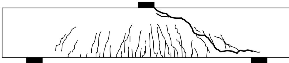
(b) After shear failure ( $P_{max}=1261\text{ kN}$ )
