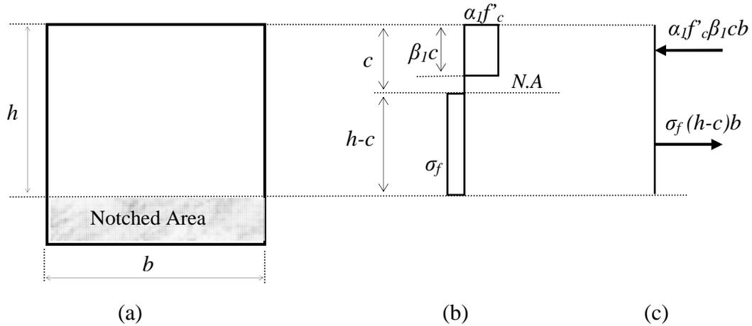
Figure 4-16: The equivalent uniform stress across the section of an SFRC prism in flexural test a) The notched section at mid-span b) Stress distribution c) Compression and Tension forces.
