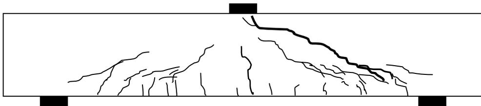
(b) After shear failure ( $P_{max} = 595 \text{ kN}$ )
