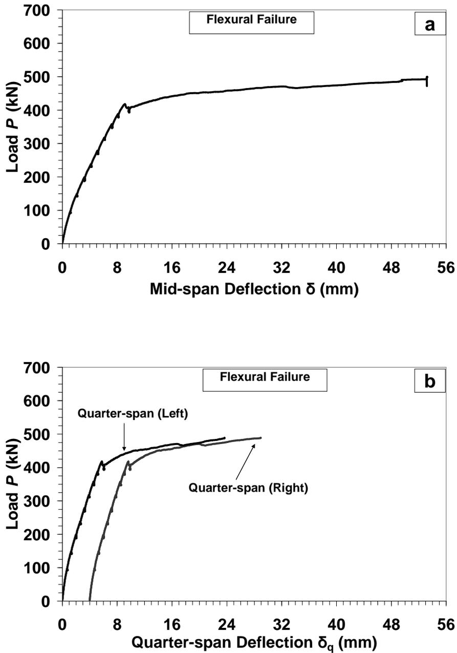
Figure B-42: Load-Deflection response for specimen *L6I* at (a) mid-span; (b) quarter-span. (Note: all presented deflection data were corrected for the measured support settlement)
