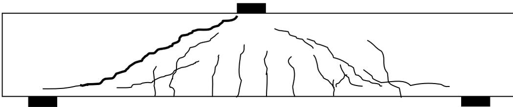
(b) After shear failure ( $P_{max}=420\text{ kN}$ )
