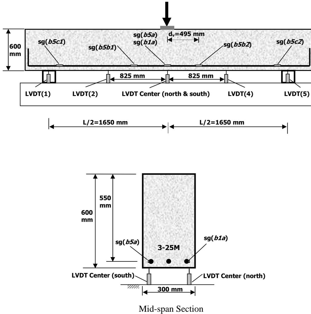
Figure B-41: Instrumentation for specimen *L61* (sg: strain gauge).
