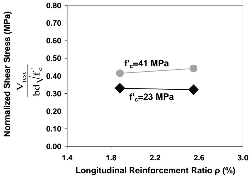
Figure 6-20: Effect of longitudinal reinforcement ratio on the shear capacity of SFRC specimens with  $h=600$  mm.
