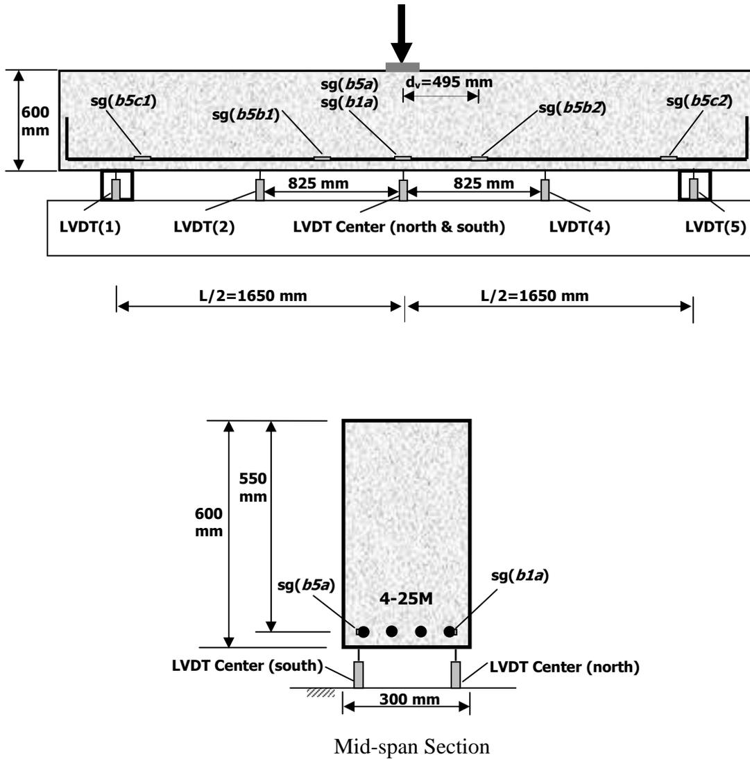
Figure B-45: Instrumentation for specimen *L62* (sg: strain gauge).
