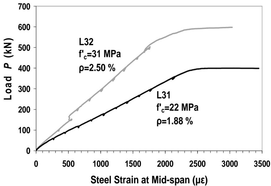
Figure 8-3: Load-steel strain response at mid-span for lightweight SFRC specimens with  $h=308$  mm.
