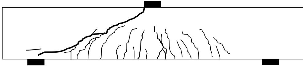
(b) After shear failure ( $P_{max}=612\text{ kN}$ )
