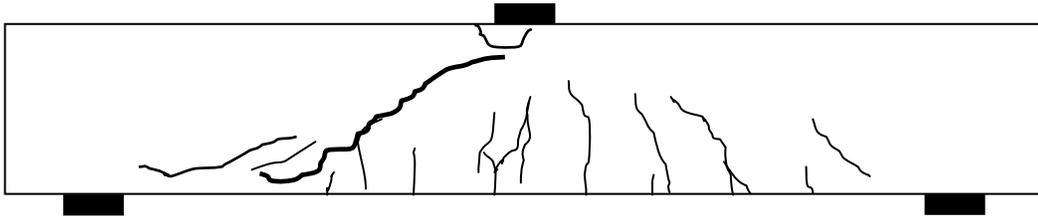
(b) After shear failure ( $P_{max}=554\text{ kN}$ )
