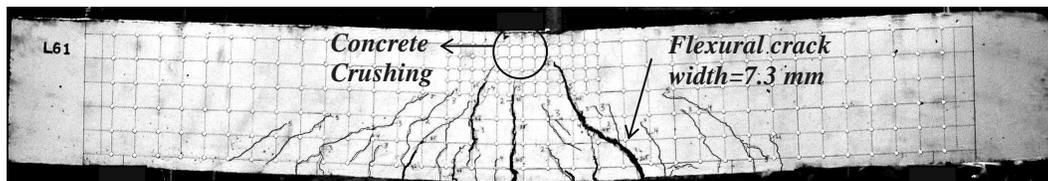
Figure 8-7: Crack pattern after flexural failure for specimen *L61* with  $h = 600 \text{ mm}$ ,  $f'_c = 30 \text{ MPa}$ , and  $\rho = 0.91 \%$ . Size of grid on the specimen surface is  $100 \text{ mm}$ .
