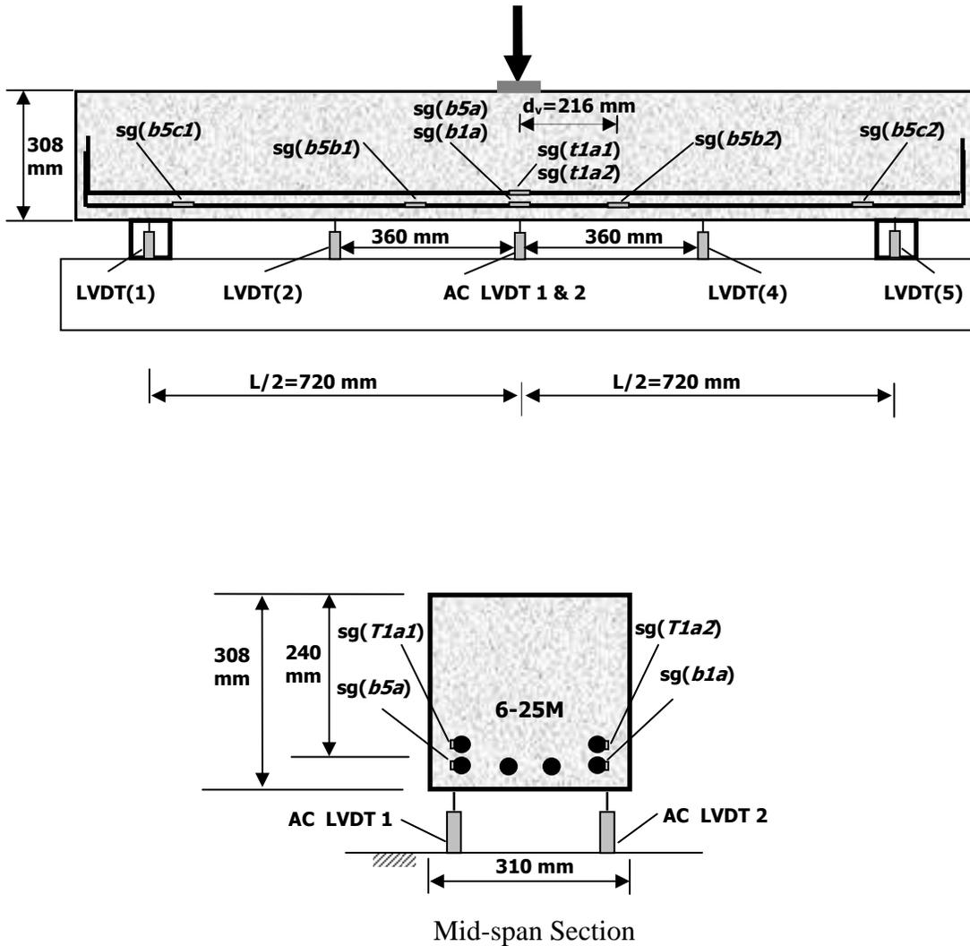
Figure B-13: Instrumentation for specimen *H32* (sg: strain gauge).
