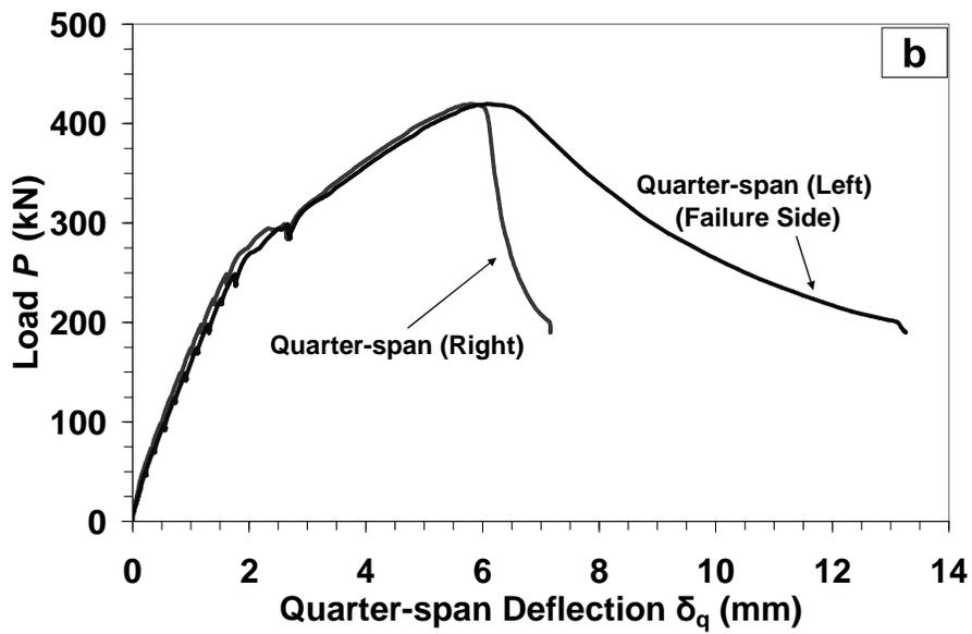
Figure B-2: Load-Deflection response for specimen N31 at (a) mid-span; (b) quarter-span. (Note: all presented deflection data were corrected for the measured support settlement)
