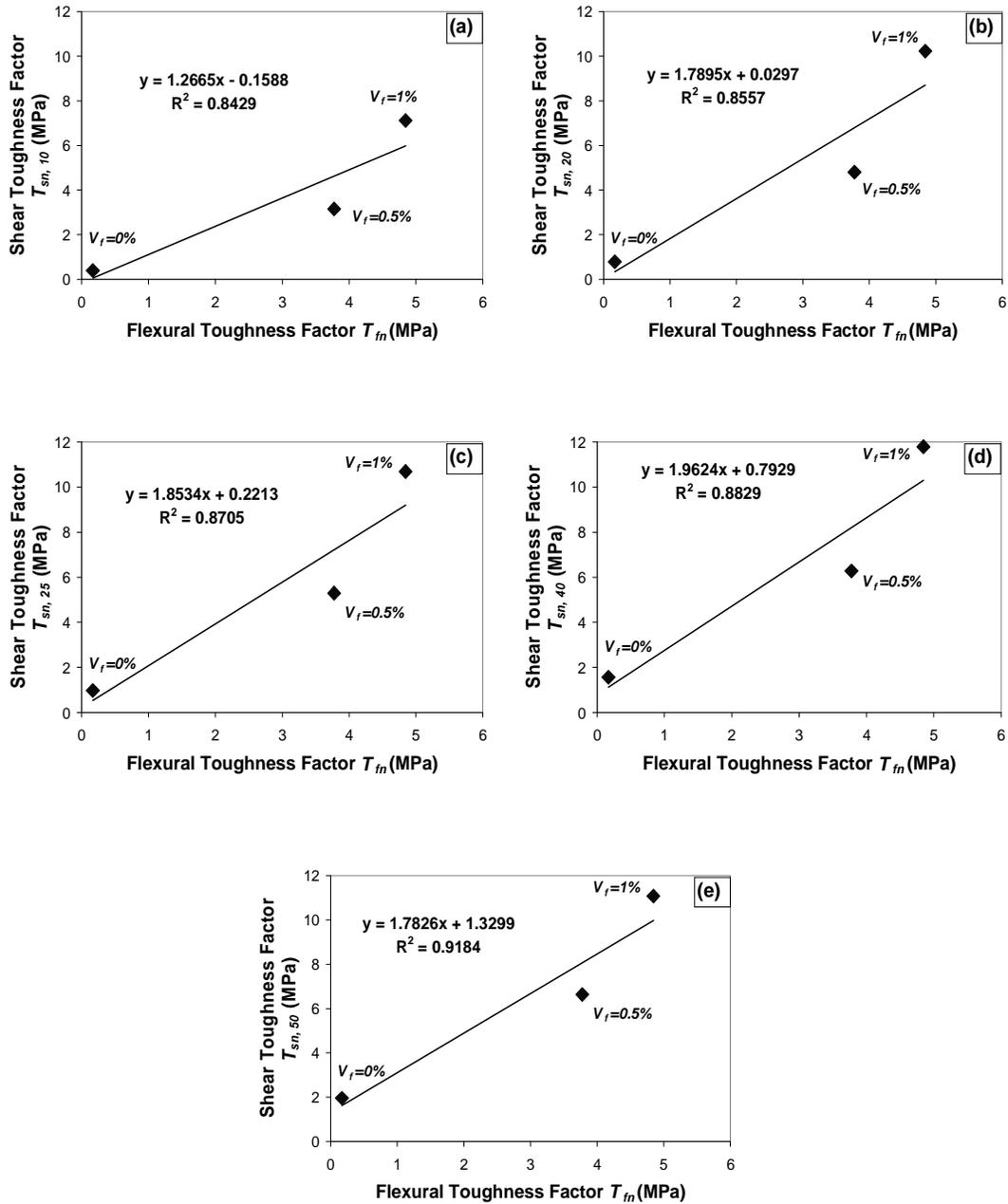
Figure 4-10: Correlation between the Flexural and Shear Toughness Factors of Normal Strength Concrete for a)  $\delta_s = h/10$  b)  $\delta_s = h/20$  c)  $\delta_s = h/25$  d)  $\delta_s = h/40$  e)  $\delta_s = h/50$
