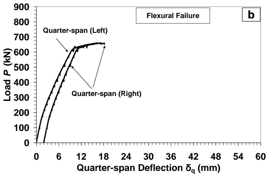
Figure B-70: Load-Deflection response for specimen *L10-2* at (a) mid-span; (b) quarter-span. (Note: all presented deflection data were corrected for the measured support settlement)
