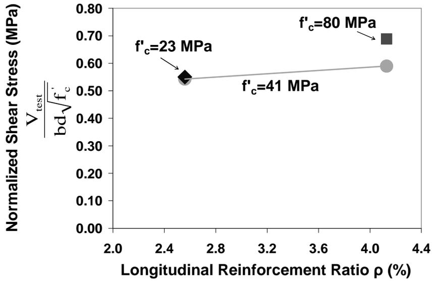
Figure 6-19: Effect of longitudinal reinforcement ratio on the shear capacity of SFRC specimens with  $h=308$  mm.
