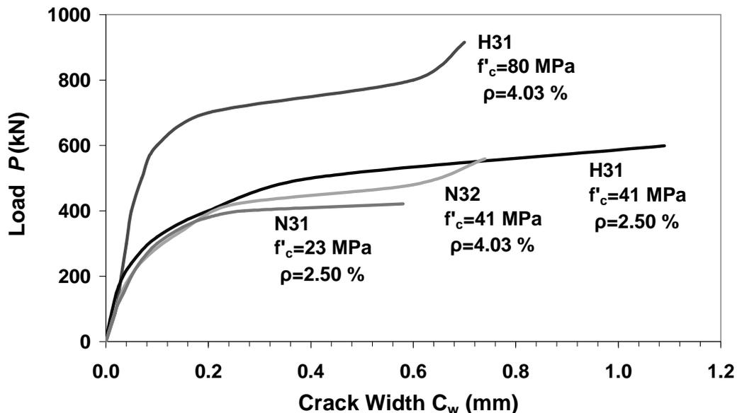
Figure 6-4: Load-crack width response for critical shear crack at level of longitudinal reinforcement in specimens with  $h=308$  mm.
