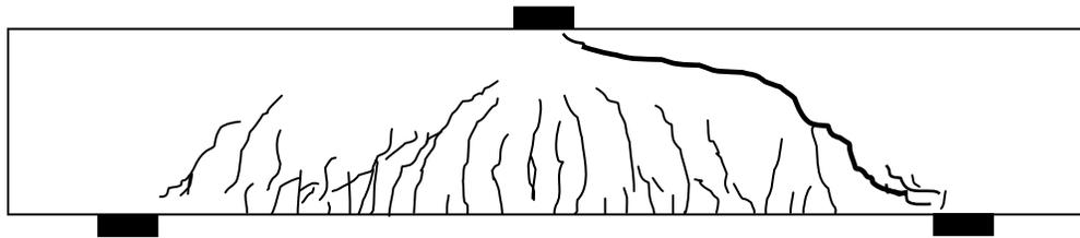
(b) After shear failure ( $P_{max}=968\text{ kN}$ )
