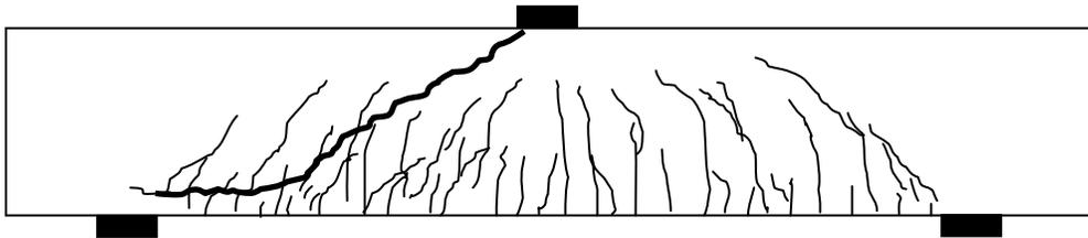
(b) After shear failure ( $P_{max}=958\text{ kN}$ )
