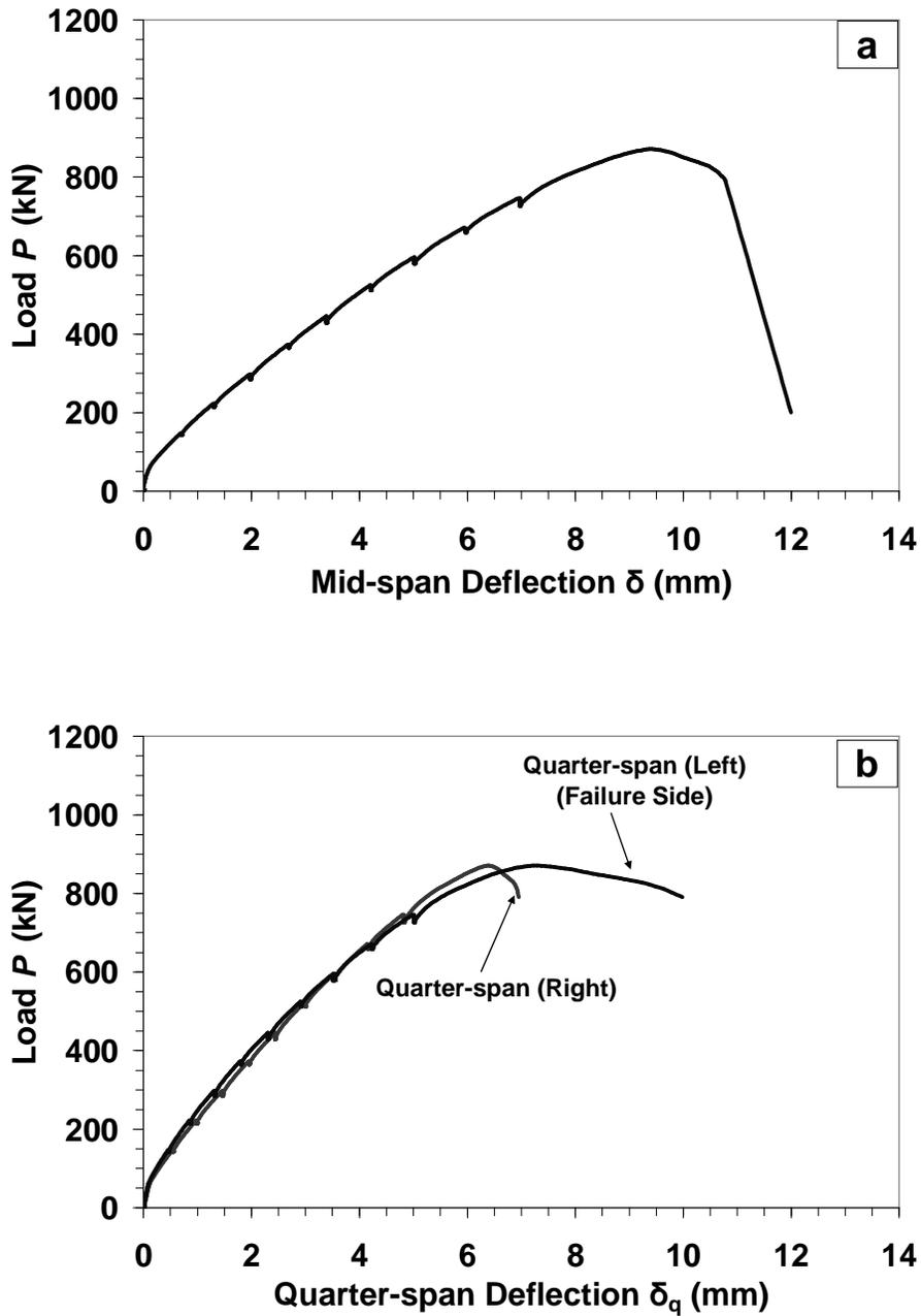
Figure B-38: Load-Deflection response for specimen *H62* at (a) mid-span; (b) quarter-span. (Note: all presented deflection data were corrected for the measured support settlement)
