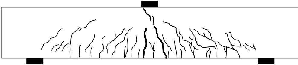
(b) After flexural failure ( $P_{max}=838\text{ kN}$ )
