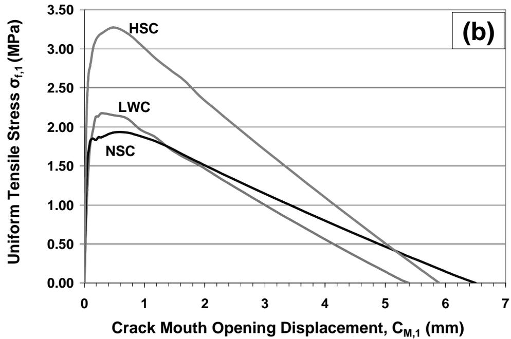
Figure 4-17: Equivalent uniform tensile stress versus CMOD for a)  $V_f=0.5\%$
