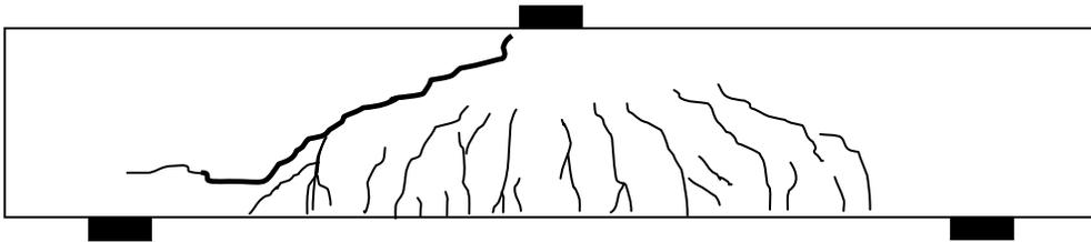
(b) After shear failure ( $P_{max}=405\text{ kN}$ )
