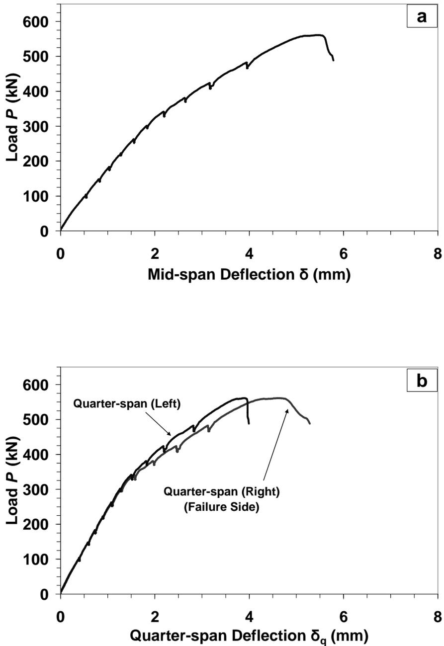
Figure B-6: Load-Deflection response for specimen N32 at (a) mid-span; (b) quarter-span. (Note: all presented deflection data were corrected for the measured support settlement)
