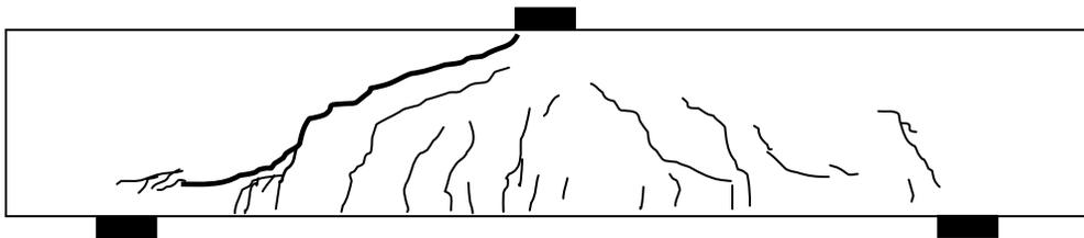
(b) After shear failure ( $P_{max}=476\text{ kN}$ )
