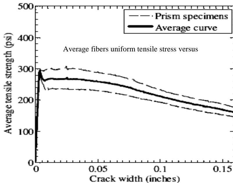
Figure 2-7: Average tensile stress versus CMOD (*Dinh 2009*)
