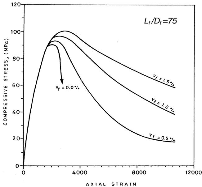
Figure 2-2: Compressive response of high strength SFRC with different volume fractions of hooked end steel fibers (adapted from *Wafa and Ashour 1992*).
