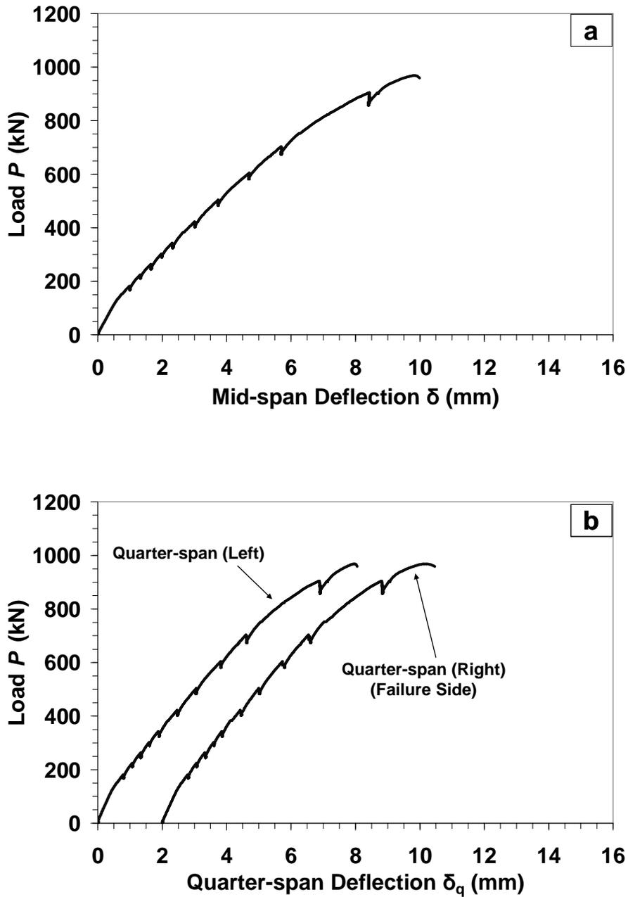
Figure B-54: Load-Deflection response for specimen *N10-2* at (a) mid-span; (b) quarter-span. (Note: all presented deflection data were corrected for the measured support settlement)
