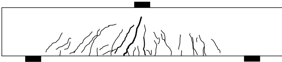
(b) After flexural failure ( $P_{max}=692\text{ kN}$ )
