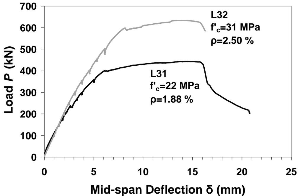
Figure 8-2: Load-deflection response at mid-span for lightweight SFRC specimens with  $h=308$  mm.
