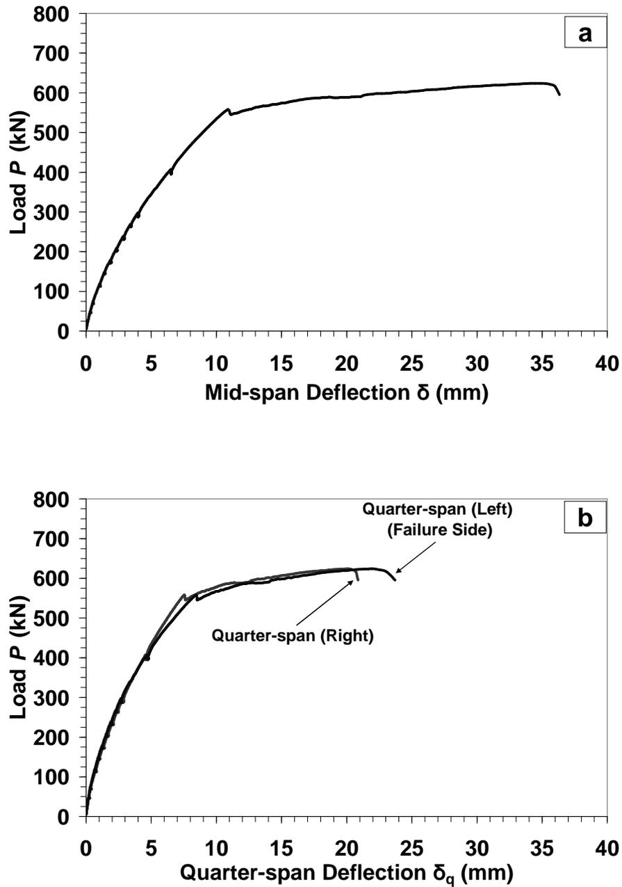
Figure B-46: Load-Deflection response for specimen *L62* at (a) mid-span; (b) quarter-span. (Note: all presented deflection data were corrected for the measured support settlement)
