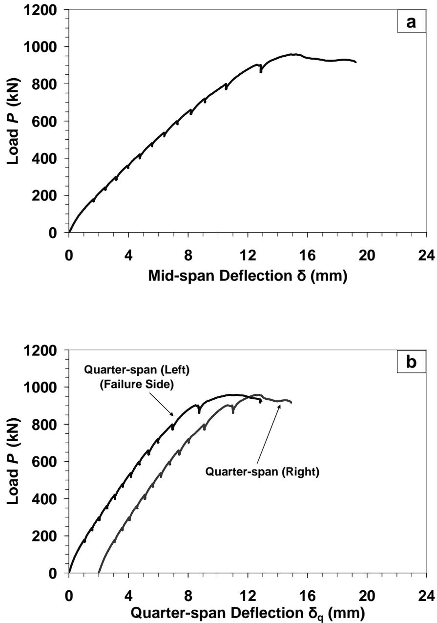
Figure B-50: Load-Deflection response for specimen *N10-1* at (a) mid-span; (b) quarter-span. (Note: all presented deflection data were corrected for the measured support settlement)
