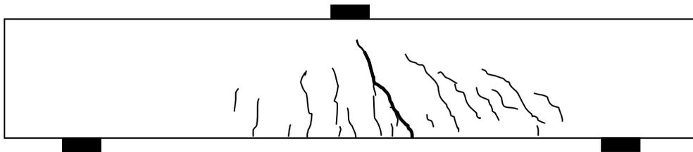
(b) After flexural failure ( $P_{max}=532\text{ kN}$ )
