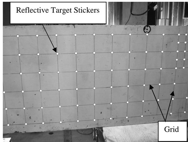
Figure 5-6: Reflective target stickers for photogrammetric system
