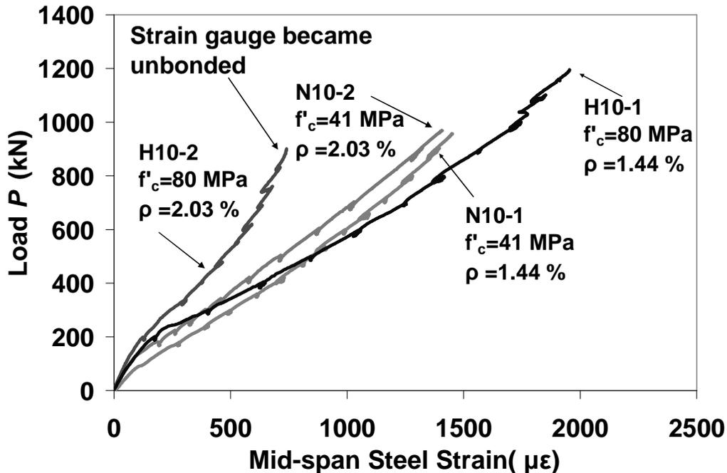
Figure 6-12: Load-steel strain response at mid-span for specimens with  $h=1000 \text{ mm}$ .
