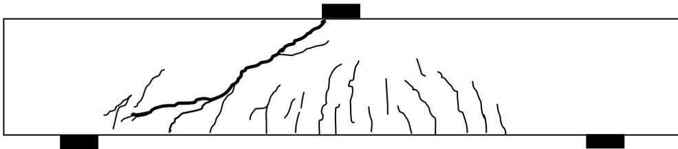
(b) After shear failure ( $P_{max}=496\text{ kN}$ )
