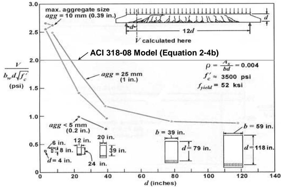
Figure 2-14: Influence of member depth and maximum aggregate size on the normalized shear stress at failure from tests performed by *Shioya et al.* 1989 and *Shioya* 1989 (figure adapted from *Lubell et al.* 2004).
