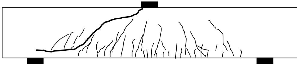
(b) After shear failure ( $P_{max}=1265\text{ kN}$ )
