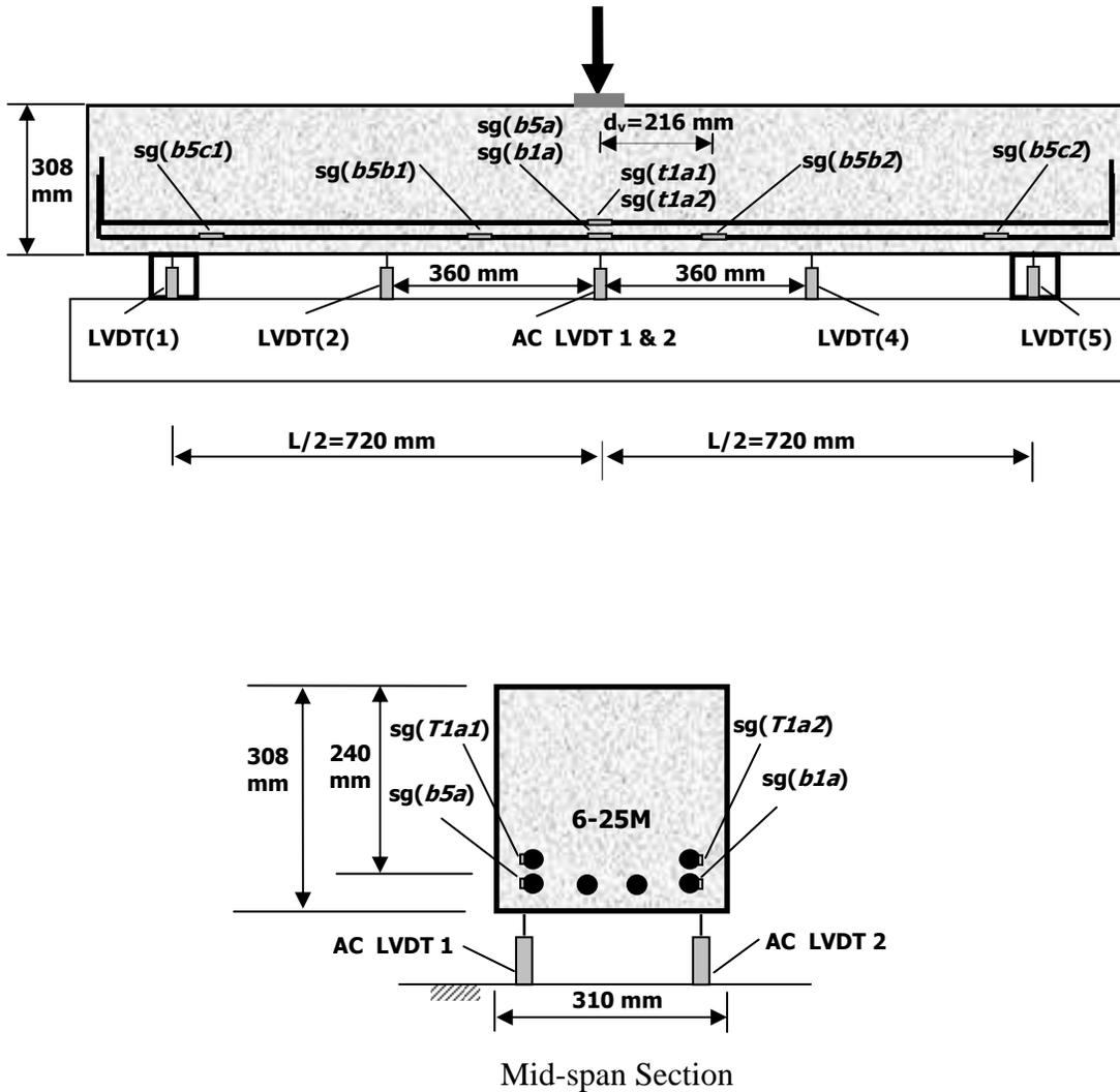
Figure B-5: Instrumentation for specimen N32 (sg: strain gauge).
