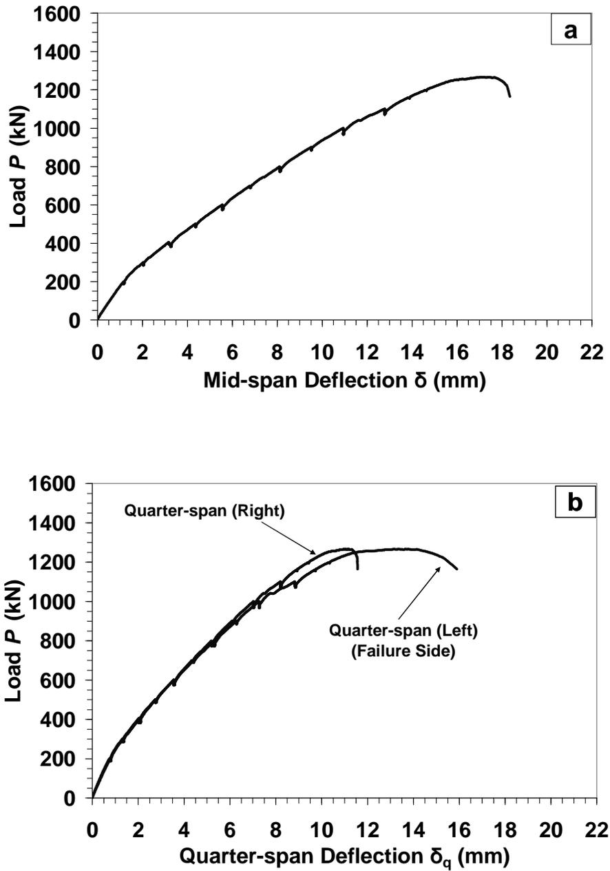
Figure B-58: Load-Deflection response for specimen *H10-1* at (a) mid-span; (b) quarter-span. (Note: all presented deflection data were corrected for the measured support settlement)
