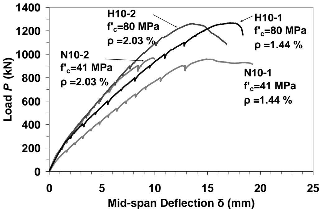
Figure 6-11: Load-Deflection response at mid-span for specimens with  $h=1000$  mm.
