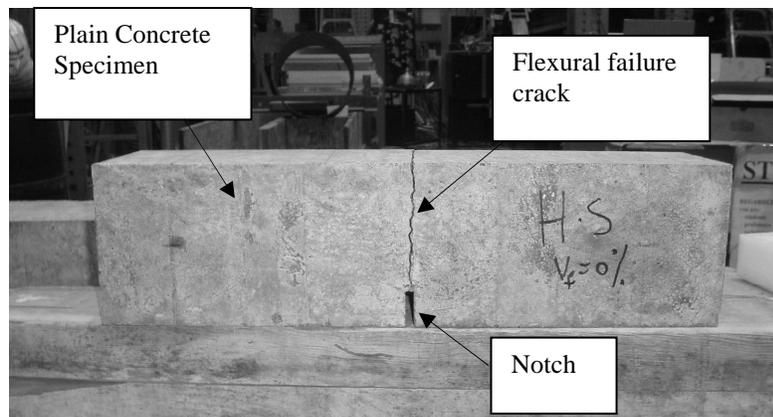
Figure 3-7: A notched specimen failed in flexure
