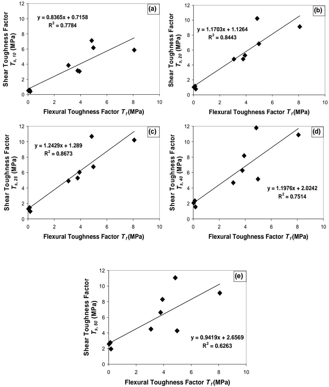
Figure 4-13: Correlation between the Flexural and Shear Toughness Factors of all mixes for a)  $\delta_s = h/10$  b)  $\delta_s = h/20$  c)  $\delta_s = h/25$  d)  $\delta_s = h/40$  e)  $\delta_s = h/50$
