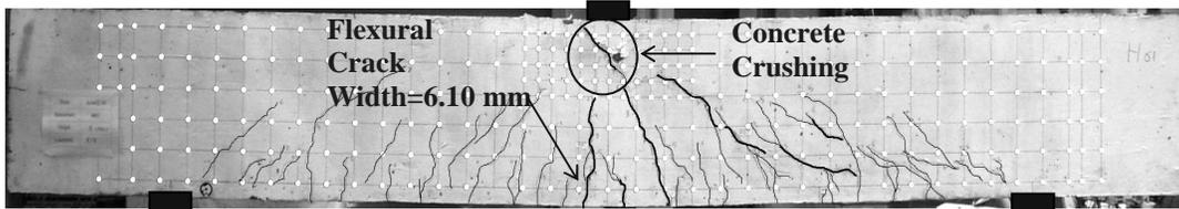
Figure 6-6: Crack pattern after flexural failure for specimen *H61* with  $h=600\text{mm}$ ,  $f'_c=41\text{ MPa}$ , and  $\rho=1.88\%$ . Size of grid on the specimen surface is 100 mm.
