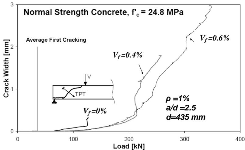
Figure 2-12: Load-crack width curve (TPT: Potentiometric transducer placed at the mid-height with a  $40^\circ$  inclination to the longitudinal axis for crack width measurement) (adapted from Minelli and Plizzari 2006).
