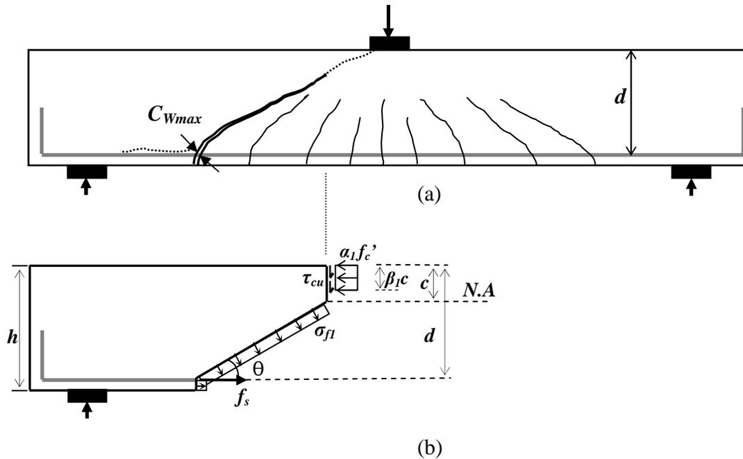
Figure 7-1: a) A critical shear crack before shear failure b) Distribution of stress along diagonal crack and compression zone for proposed model
