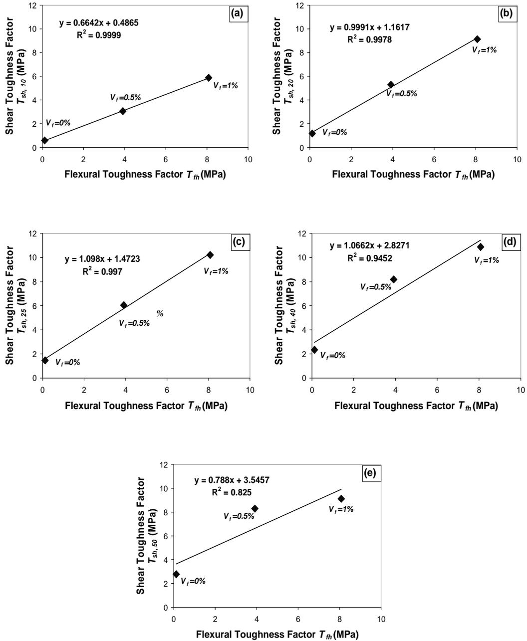
Figure 4-12: Correlation between the Flexural and Shear Toughness Factors of High Strength Concrete for a)  $\delta_s = h/10$  b)  $\delta_s = h/20$  c)  $\delta_s = h/25$  d)  $\delta_s = h/40$  e)  $\delta_s = h/50$
