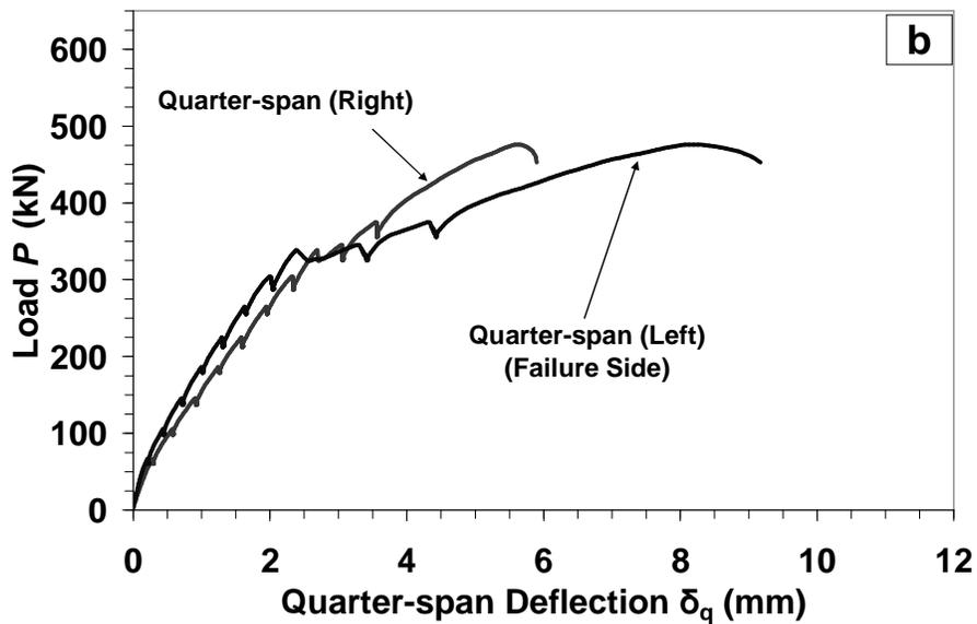
Figure B-26: Load-Deflection response for specimen *N61* at (a) mid-span; (b) quarter-span. (Note: all presented deflection data were corrected for the measured support settlement)
