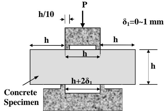
Figure 2-10: Direct shear test configuration according to *JSCE-G 53-1999*.
