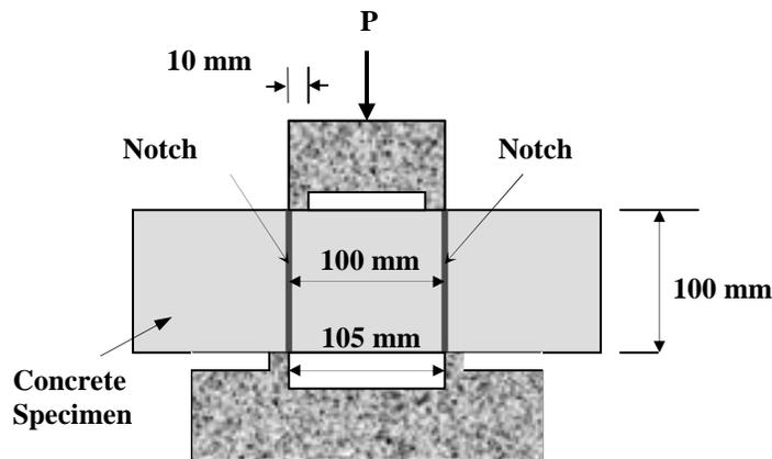
Figure 3-8: Schematic of the Direct Shear Test
