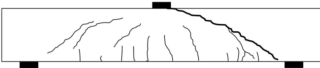
(b) After shear failure ( $P_{max}=560\text{ kN}$ )
