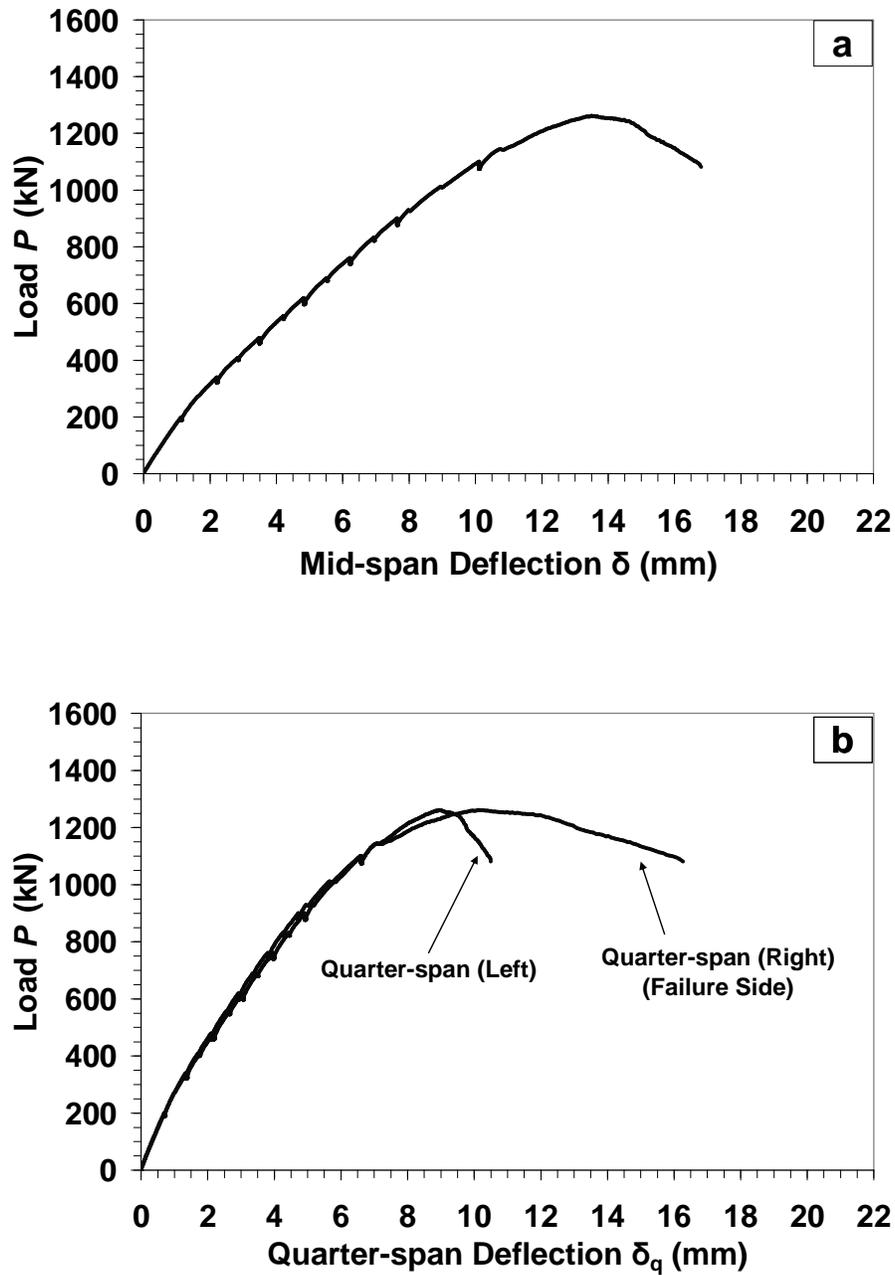
Figure B-62: Load-Deflection response for specimen *H10-2* at (a) mid-span; (b) quarter-span. (Note: all presented deflection data were corrected for the measured support settlement)
