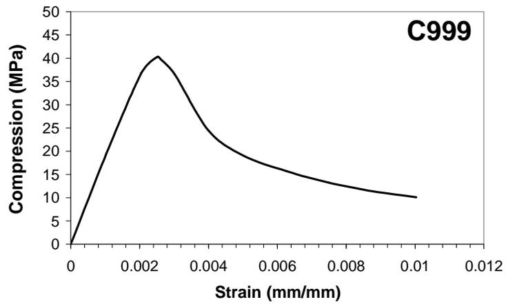
Figure A-21: Compressive Stress-Strain Response for Lightweight Concrete
