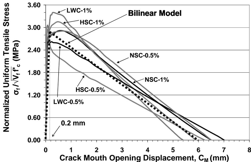
Figure 4-18: Normalized equivalent uniform tensile stress versus CMOD
