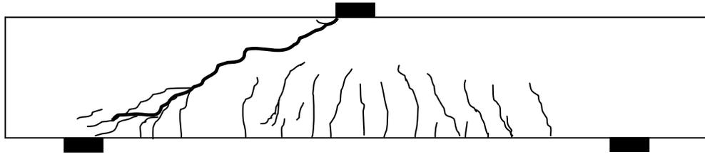
(b) After shear failure ( $P_{max}=880\text{ kN}$ )
