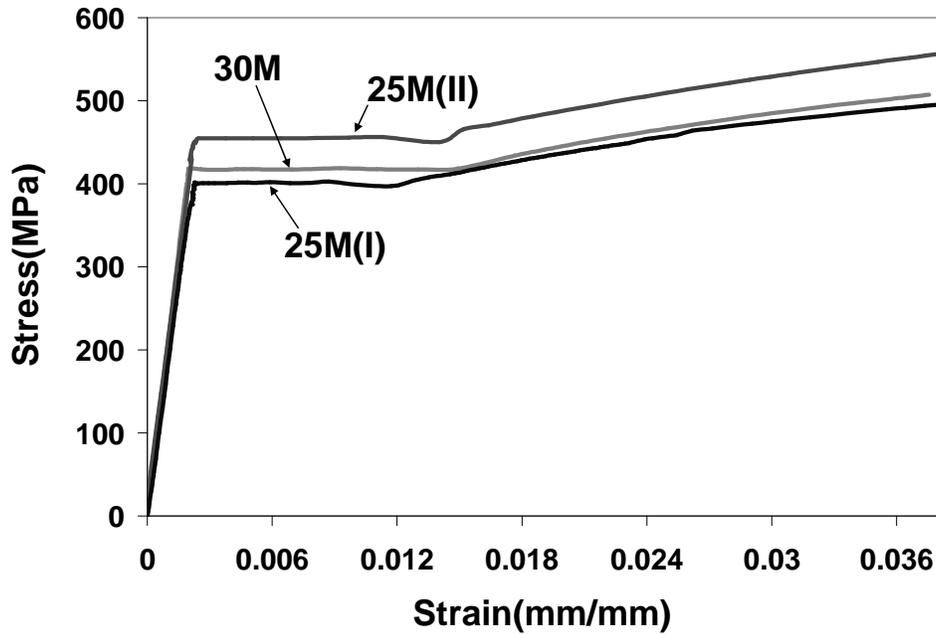
Figure 5-3: Representative tensile stress-strain response of Steel rebars
