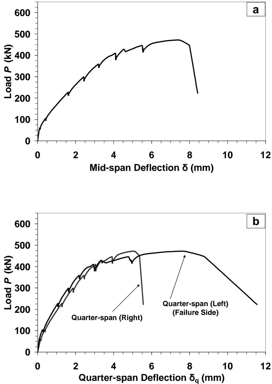
Figure B-30: Load-Deflection response for specimen *N62* at (a) mid-span; (b) quarter-span. (Note: all presented deflection data were corrected for the measured support settlement)
