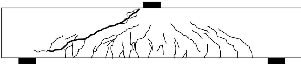
(b) After shear failure ( $P_{max}=915 \text{ kN}$ )
