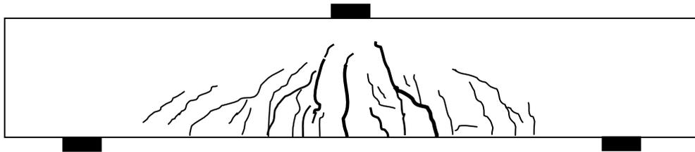
(b) After flexural failure ( $P_{max}=497\text{ kN}$ )
