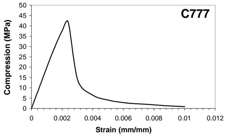
Figure A-19: Compressive Stress-Strain Response for Lightweight Concrete
