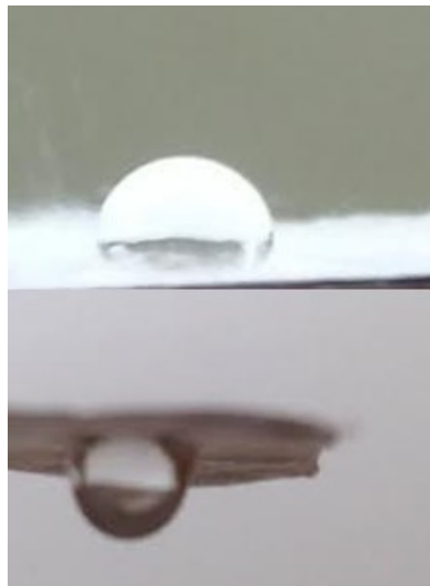
Figure 6. 15: Observation of the rose petal effect on the PS electrospun samples
