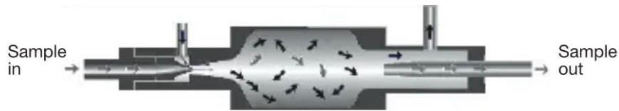
Figure 3.6: Dekati DI-1000 diluter schematic [2]
