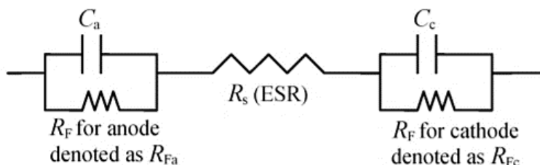
Figure 2.11. A single cell supercapacitor RC equivalent circuit. [85]
