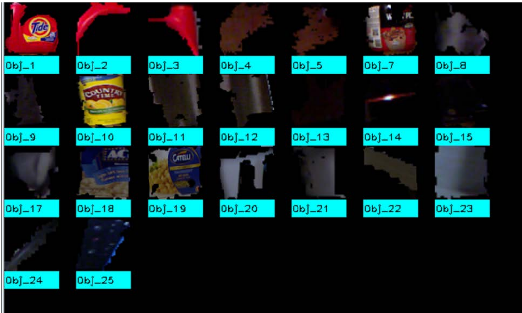
Figure 5.5: Example of object detection using the segmentation framework. The objects collected using object discovery are shown in this image. Obj_X is the name of the object generated automatically.
