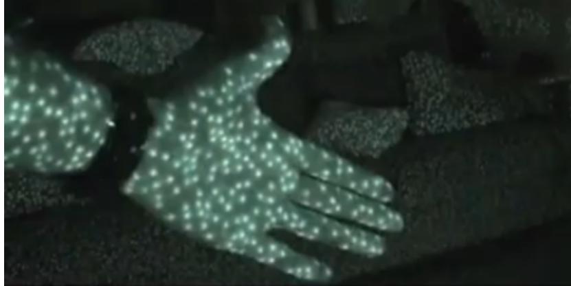
Figure 2.2: Structured light pattern projected by Kinect. Source: http://blogs.msdn.com/b/msroboticsstudio/archive/2011/11/29/kinect-for-robotics.aspx
