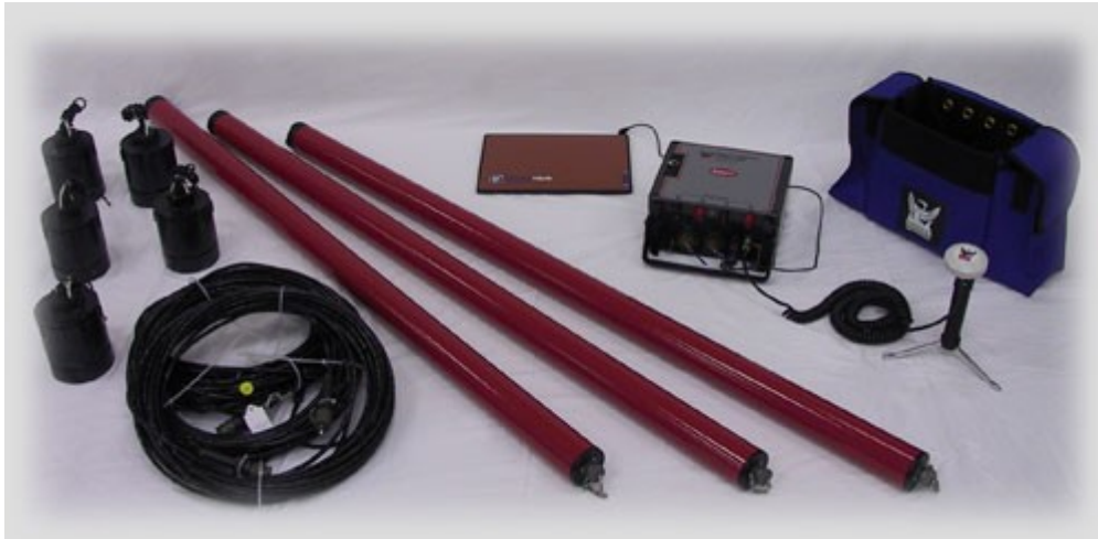
Figure 5.3: The Phoenix Geophysics V5-2000 system 4 .
