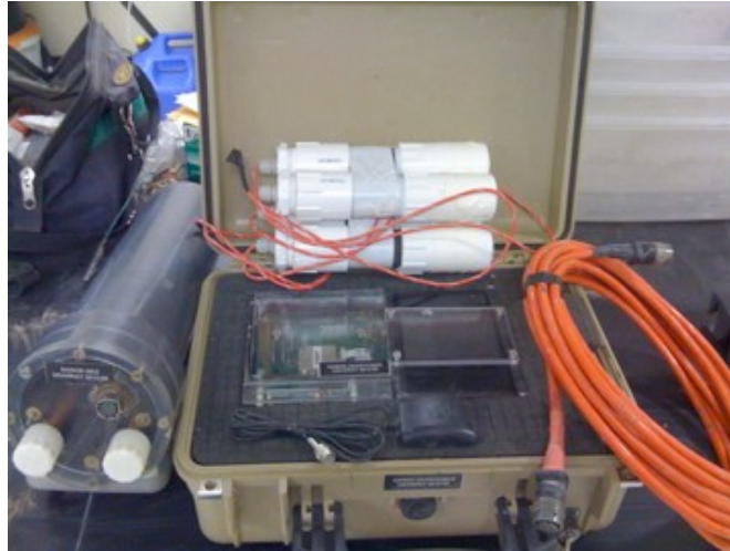
Figure 5.4: The Narod Intelligent Magnetotelluric System 5 (NIMS).
