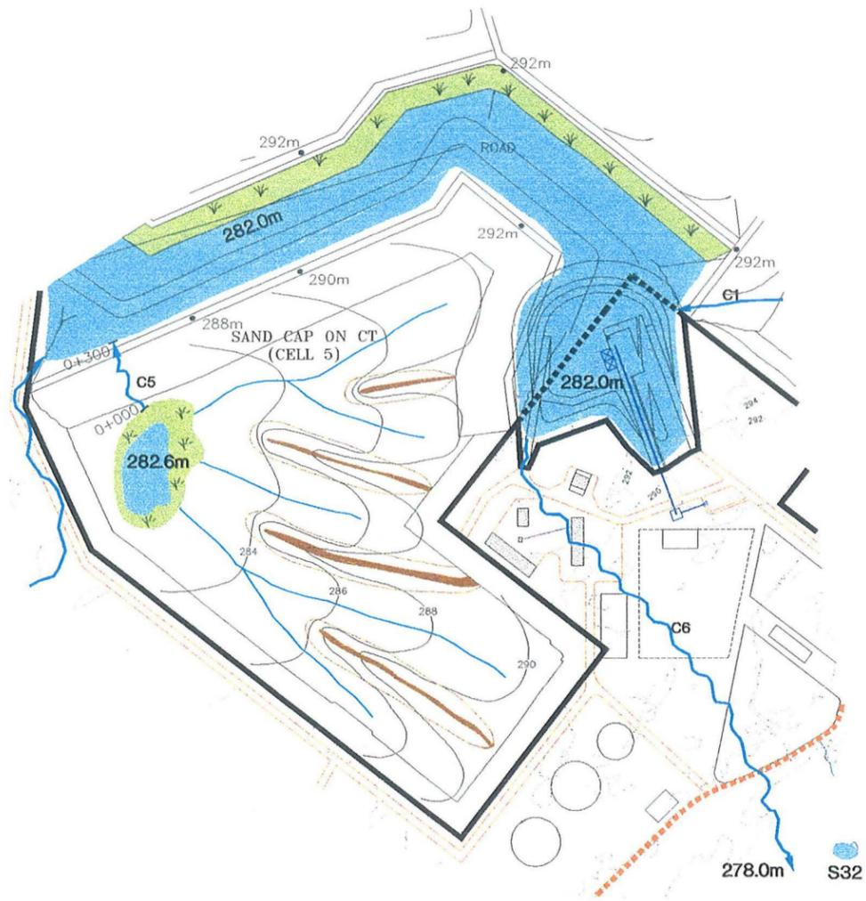
**PLAN OF MAIN DRAINAGE CHANNEL FOR CELL 5**
