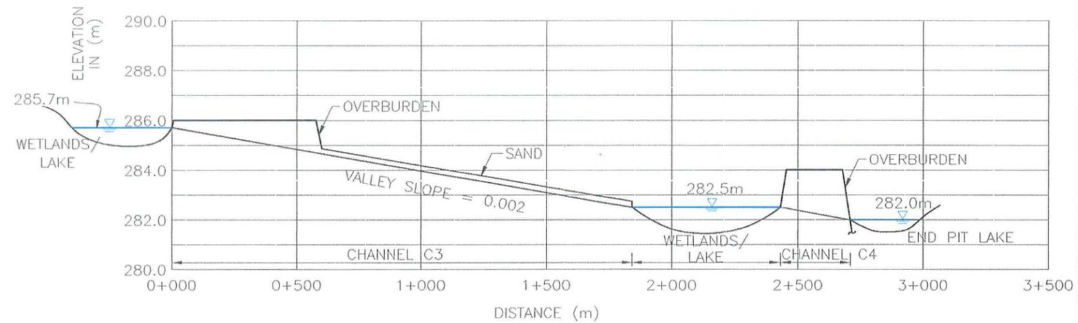
PROFILE OF MAIN DRAINAGE CHANNELS C3 AND C4
