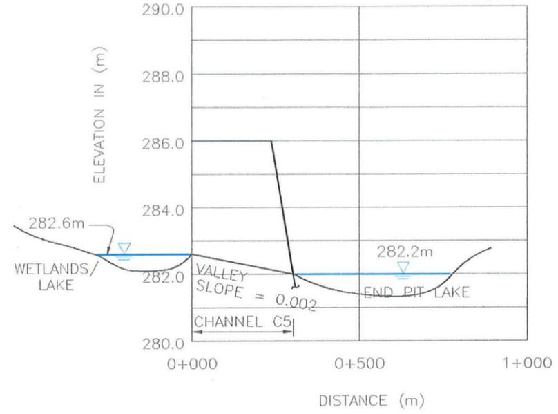
**PROFILE OF MAIN DRAINAGE CHANNEL C5**
