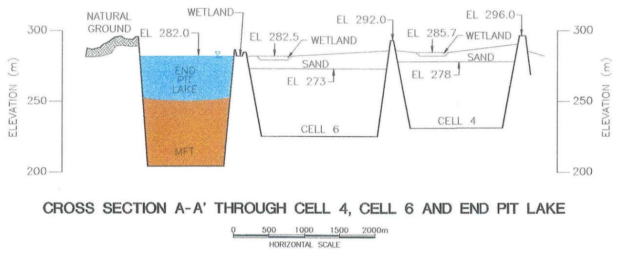
CROSS SECTION A-A' THROUGH CELL 4, CELL 6 AND END PIT LAKE
