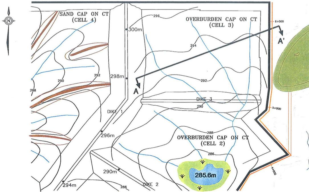
**SECONDARY DRAINAGE CHANNELS AT STORAGE AREAS WITH OVERBURDEN CAP ON CT**
