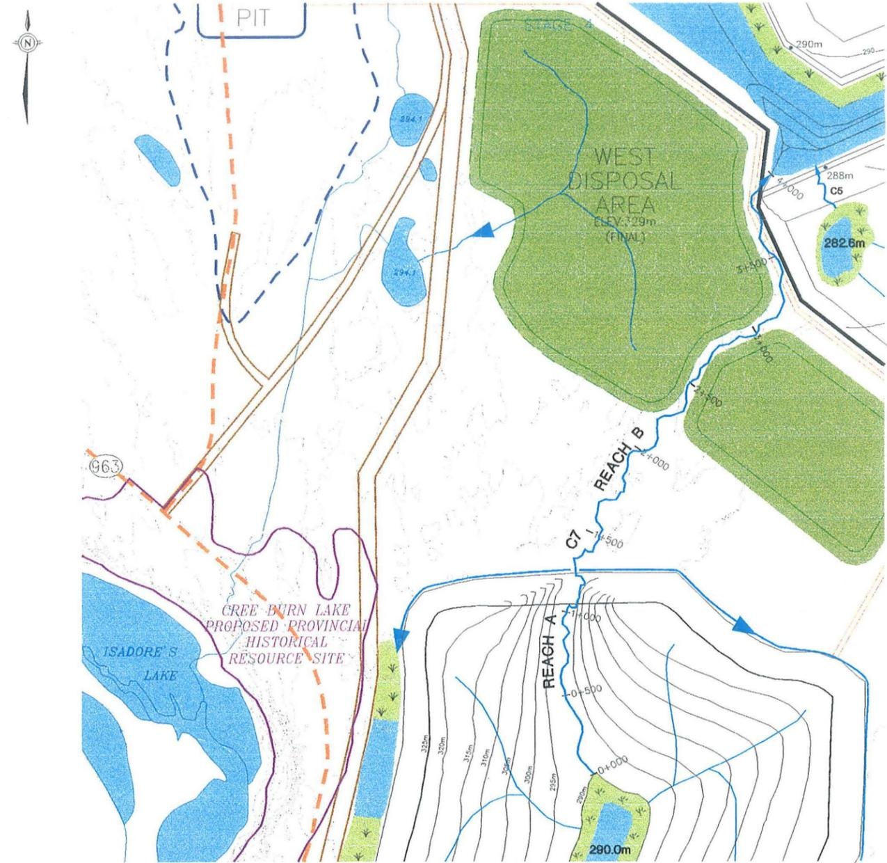
**PLAN OF MAIN DRAINAGE CHANNEL (C7) FROM RECLAIMED TAILINGS SETTLING POND TO END PIT LAKE**
