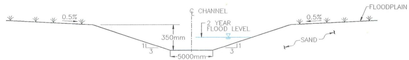
TYPICAL CROSS SECTION FOR MAIN CHANNEL C4
