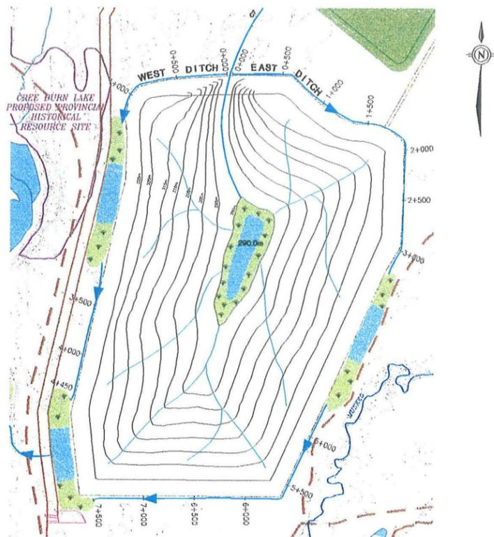
**PLAN OF RECLAIMED TAILINGS SETTLING POND**
