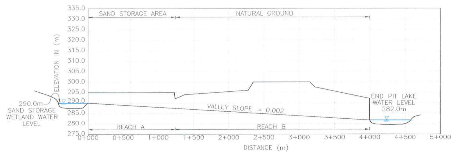
**PROFILE OF MAIN DRAINAGE CHANNEL C7**
