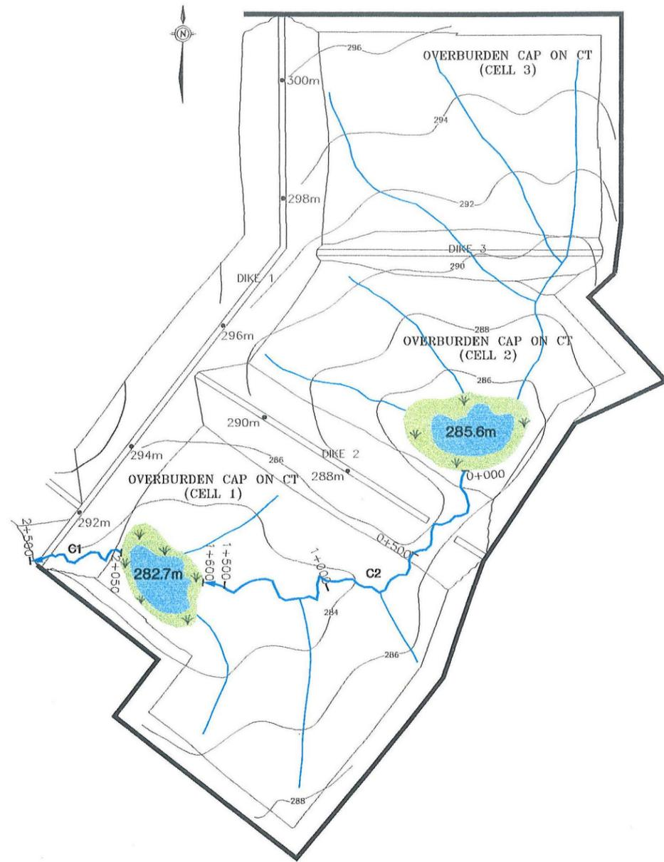
PLAN OF MAIN DRAINAGE CHANNELS FOR CELLS 1, 2 AND 3
