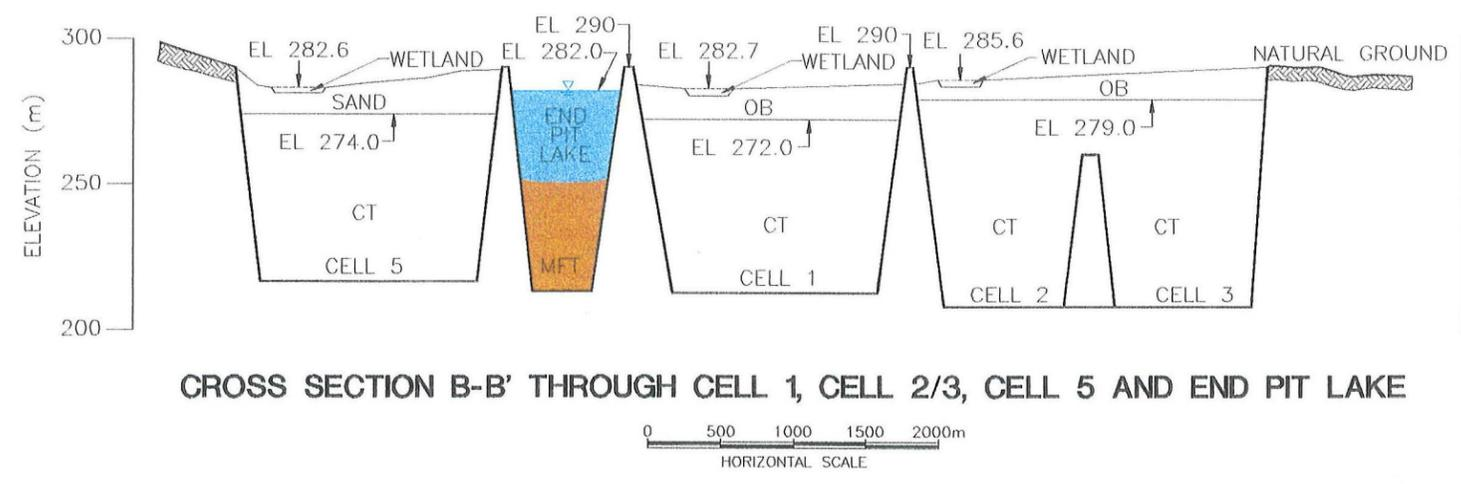
CROSS SECTION B-B' THROUGH CELL 1, CELL 2/3, CELL 5 AND END PIT LAKE
