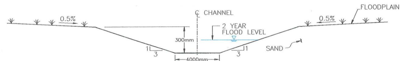
TYPICAL CROSS SECTION FOR MAIN CHANNELS C1 AND C2
