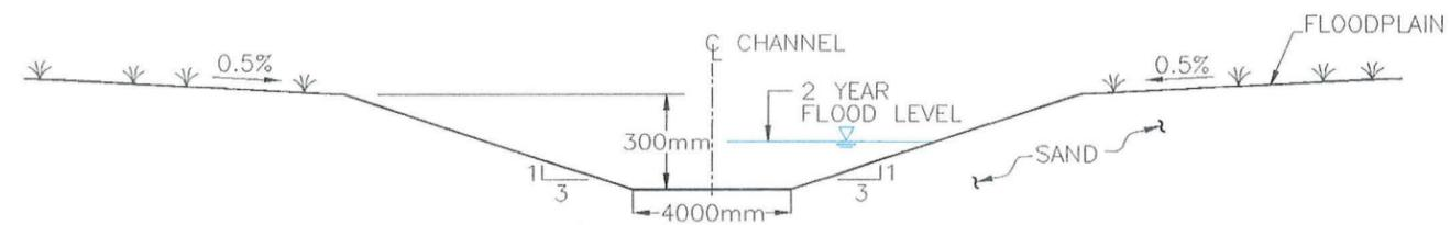
TYPICAL CROSS SECTION FOR MAIN CHANNEL C3
