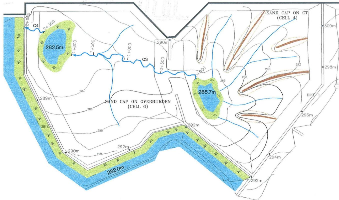
PLAN OF MAIN DRAINAGE CHANNELS FOR CELLS 4 AND 6
