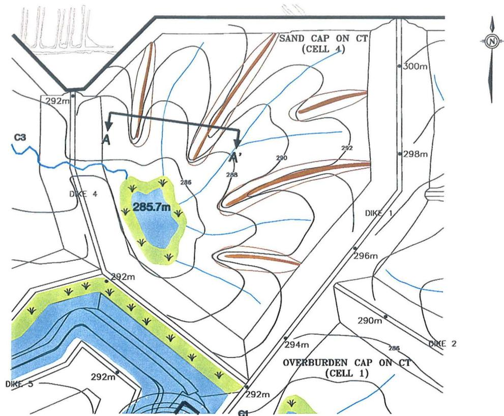
**SECONDARY DRAINAGE CHANNELS AT STORAGE AREAS WITH SAND CAP ON CT**
