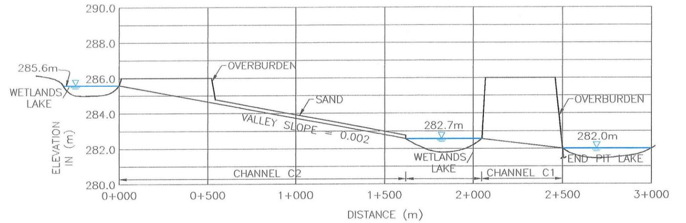
PROFILE OF MAIN DRAINAGE CHANNELS C1 AND C2
