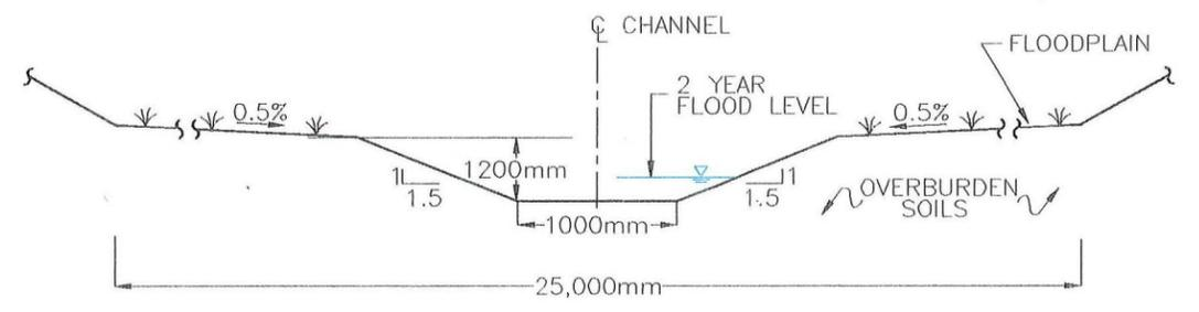
**TYPICAL CROSS SECTION FOR MAIN CHANNEL C6**
