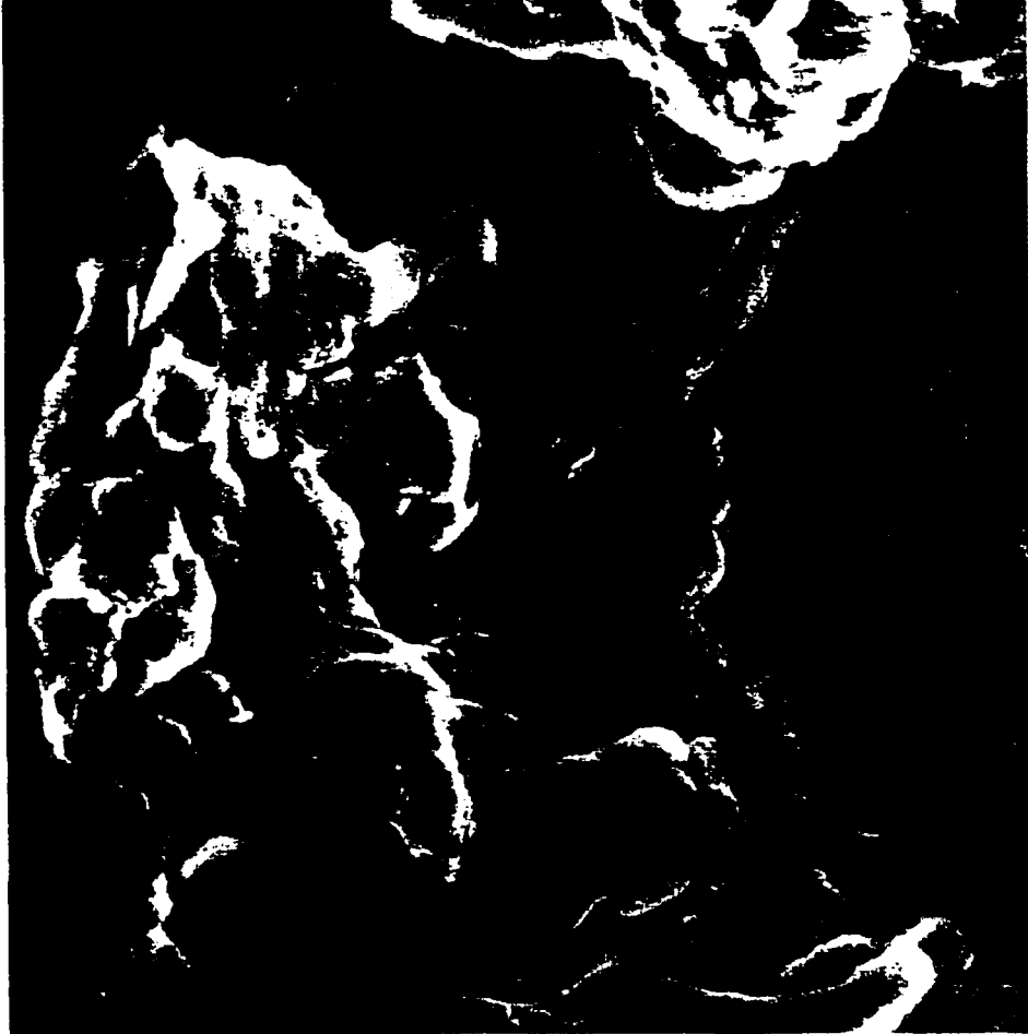
Figure B.1. Cryogenic scanning electron microscopy of Devon hydrocarbon-contaminated soil. X1000. The image illustrates the microorganisms associated with clay aggregates.
