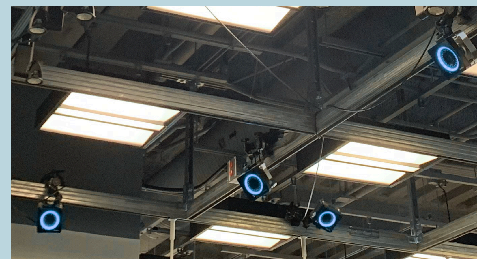
Figure 6: OptiTrack Rig/Camera Setup
