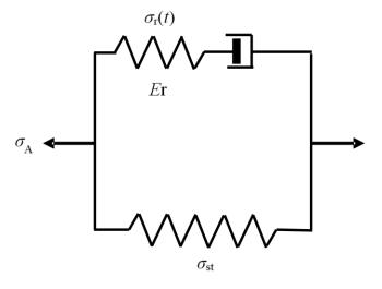
Fig. 4.1 Schematic diagram of the standard, visco-elastic model used in this work.
