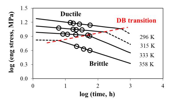
Fig. 5.3 Master curves of engineering stress versus time, including the DB transition and creep test results.
