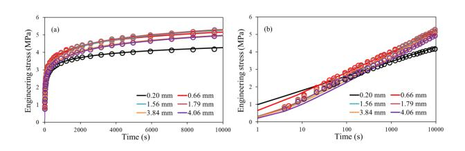
Fig. 4.2 Examples of stress drop obtained from the MR tests (open circles) and generated based on Eq. (4.8) (solid lines) for all stress relaxation stages: (a) with time in the linear scale, and (b) with time in the logarithmic scale.
