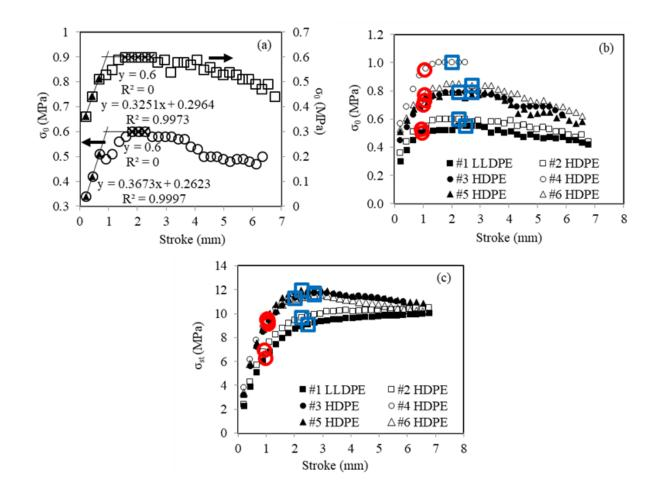
Fig. 4.6 Summary of MR test results: (a) sample curves showing the approach used to determine the stroke for the 1<sup>st</sup> critical point, (b) typical variation of  $\sigma_0$  with stroke, (c) typical variation of  $\sigma_{st}$  with stroke (highlighted open red circles and open blue boxes indicate the 1<sup>st</sup> critical point and the yield point, respectively).
