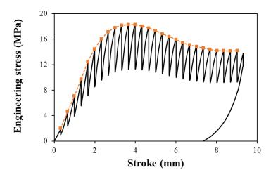
Fig. 5.5 A typical engineering stress-stroke curve (from #5 u-MDPE).
