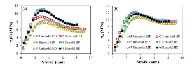
Fig. 5. 11 Two stress components determined from the multi-relaxation tests as a function of stroke for the six PE pipes: (a)  $\sigma_r(0)$  and (b)  $\sigma_{st}$ .
