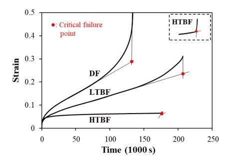
Fig. 3.2 Typical strain-time curves to demonstrate the determination of the critical failure point and the corresponding secondary creep strain rate.
