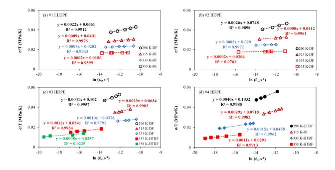
Fig. 3.6 Plots of  $\sigma/T$  versus ln ( $\dot{\varepsilon}_s$ ) for the four PEs used in the study.
