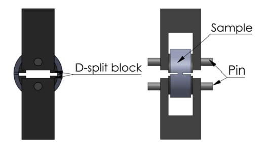
Fig. 5.2 Set-up of the D-split tensile test.
