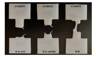
Fig. 2.4 Sample of specimens for #3 HDPE that fractured in a brittle manner (left and centre) and in a mix of brittle initiation and ductile stretch (right).
