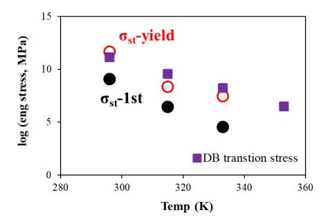
Fig. 5.4 Critical stresses for the DB transition ( $\blacksquare$ ) from creep tests, first critical quasi-static stresses ( $\bullet$ ) and critical quasi-static stress for global yielding ( $\bigcirc$ ) from short-term MR tests at different temperatures.
