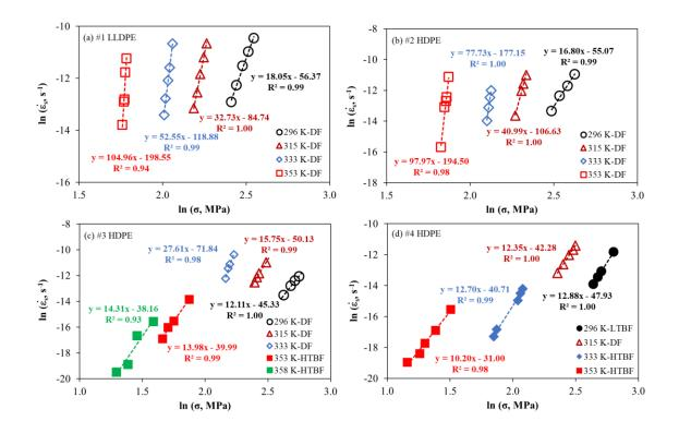
Fig. 3.4 Natural logarithmic plots of strain rate at the secondary creep stage versus the applied stress.
