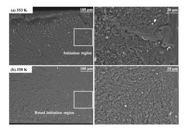
Fig. 2.9 SEM micrographs of selected brittle failure surfaces for #3 HDPE: (a) 353 K and (b) 358 K.
