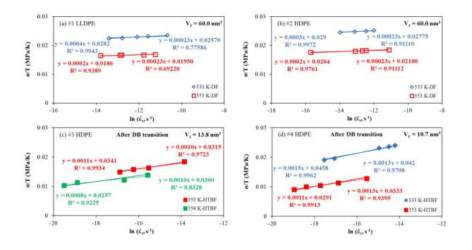
Fig. 3.7 Plots of  $\sigma/T$  versus ln ( $\dot{\epsilon}_s$ ) at two highest temperatures used in the experimental testing, for determining the  $V_1$  values.
