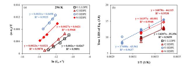
Fig. 3.10 Summary of results for determining  $V_2$ ,  $E_2$  and  $\dot{\varepsilon}_{02}$ : (a) creep data at room temperature to determine  $V_2$  based on Eq. (3.5b), and (b) plot of values from the LHS of Eq. (3.8) generated using the true  $V_2$  values, as a function of 1/T.
