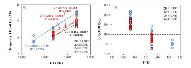
Fig. 3.9 (a) The left-hand side (LHS) of Eq. (3.8) generated using the temporary  $V_2$  values, and (b) plots of  $\frac{\dot{\varepsilon}_s}{\dot{\varepsilon}_{02}} \exp\left(\frac{E_2}{RT}\right)$  versus *T*, using temporary  $E_2$  and  $\dot{\varepsilon}_{02}$  values based on the temporary  $V_2$  values.
