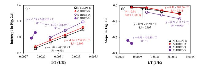
Fig. 2.7 Summary of intercepts (a) and slopes (b) used for the fitting functions in Fig. 2.6, plotted as a function of 1/T ('D' and 'B' in the legends indicate ductile and brittle failures, respectively).
