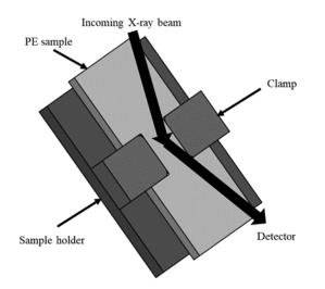
Fig. 4.4 Schematic description of the set-up for the WAXS experiment.
