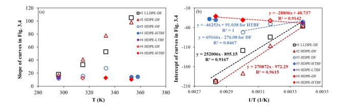
Fig. 3.5 Summary of the NPL-based analysis: (a) slopes (*n*) of the expressions in Fig. 3.4 versus *T*, and (b) intercepts of expressions in Fig. 3.4 versus 1/T. Unfilled symbols are for ductile failure and filled symbols for brittle failure.
