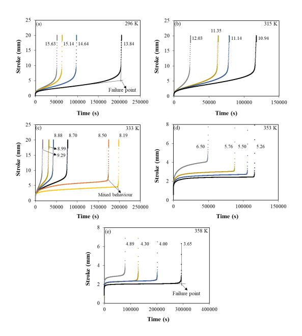
Fig. 2.5 Typical creep curves at different applied stresses and temperatures (selected from #3 HDPE).
