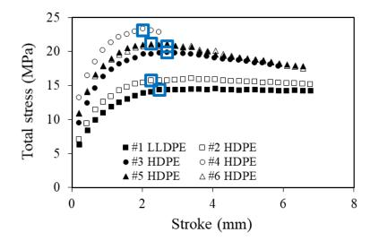
Fig. 4.5 Typical curves from the MR test, of total stress versus stroke with the total stress measured at the beginning of each stress relaxation stage, in which peak points are highlighted using open blue boxes.
