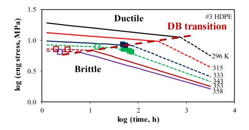
Fig. 2.10 Data from the second batch of creep tests on #3 HDPE (squares), with the line plots identical to those shown in Fig. 2.8(c).
