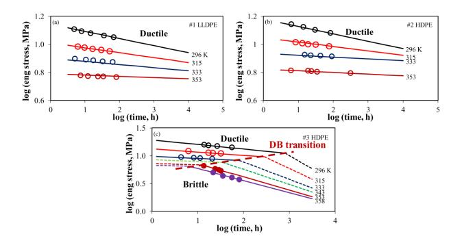
Fig. 2.8 Sample master curves generated based on Eq. (2.1): (a) #1 LLDPE, (b) #2 HDPE and (c) #3 HDPE.
