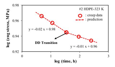
Fig. 2.11 Creep test results for #2 HDPE at 323 K.
