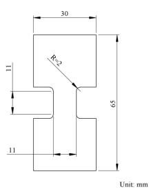
Fig. 4.3 Geometry and dimensions of the modified dog-bone specimens.
