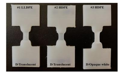
Fig. 2.3 Sample specimens in ductile failure.
