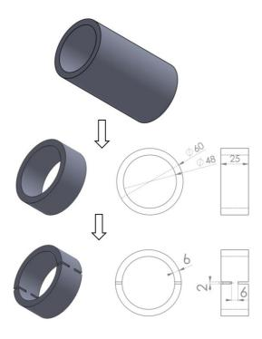
Fig. 5.1 Schematic description of specimen preparation.
