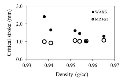
Fig. 4.9 Comparison of critical strokes in Fig. 4.8 and those for the 1st critical point from the MR test.
