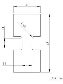
Fig. 2.2 Geometry and dimensions of the modified dog-bone specimens.
