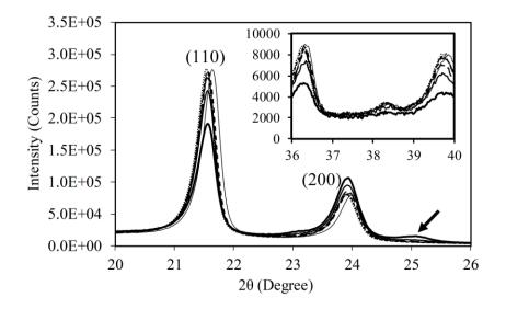
Fig. 4.7 Typical WAXS spectra with different strokes (from #2 HDPE) (Peak intensity for (110) decreases with increase of stroke applied to specimens).
