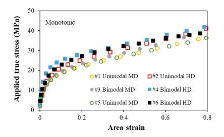
Fig. 5.7 Curves of applied true stress versus area strain for the six PE pipes.
