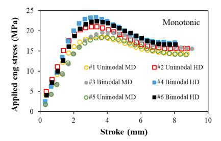
Fig. 5.6 Curves of applied engineering stress versus stroke for the six PE pipes.
