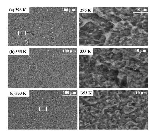
Fig. 3.11 SEM micrographs of surfaces generated by brittle failure of #4 HDPE: (a) LTBF at 296 K, (b) HTBF at 333 K and (c) HTBF at 353 K.
