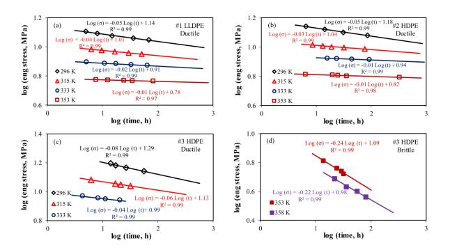
Fig. 2.6 Plots of applied stress versus time for ductile or brittle failures at different temperatures: (a) #1 LLDPE-ductile, (b) #2 HDPE-ductile, (c) #3 HDPE-ductile and (d) #3 HDPE-brittle.
