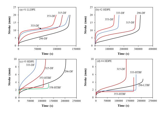
Fig. 3.1 Typical creep curves for four PEs used in the study, with temperatures indicated by the numbers next to each curve, followed by DF (ductile failure), LTBF (low-temperature brittle failure) and HTBF (high-temperature brittle failure).
