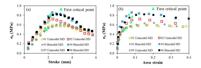
Fig. 5.10 Reference stress ( $\sigma_0$ ) as a function of (a) stroke, and (b) area strain.
