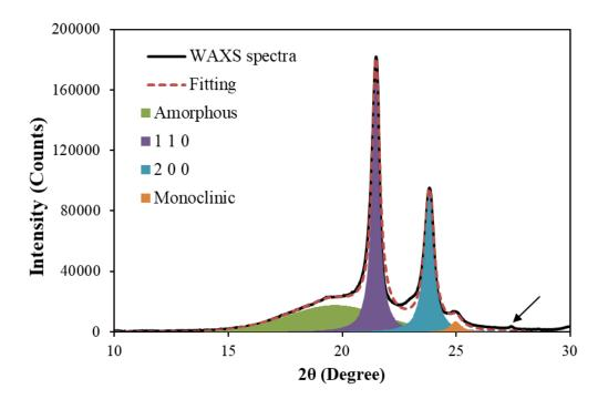
Fig. 6.1 Typical WAXS spectra (from #1 LLDPE with stroke of 5 mm) and the individual contribution of each peak from the deconvolution procedure.
