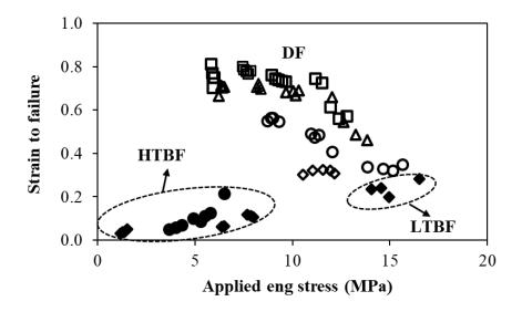
Fig. 3.3 Summary of strains to failure as a function of the applied stress for the four PEs. #1 LLDPE ( $\Box$ ), #2 HDPE ( $\triangle$ ), #3 HDPE ( $\bigcirc$  and  $\blacklozenge$ ), and #4 HDPE ( $\diamondsuit$  and  $\blacklozenge$ ), in which unfilled and filled symbols represent ductile and brittle failures, respectively.
