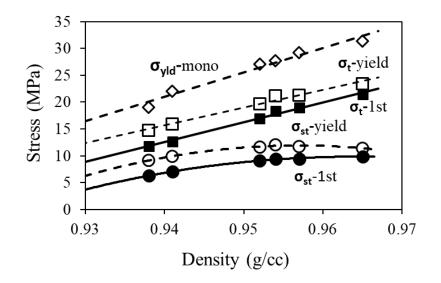
Fig. 4.10 Summary of  $\sigma_{st}$  and  $\sigma_t$  values at the 1<sup>st</sup> critical point and yield point from the MR tests ( $\sigma_{st}$ -1st,  $\sigma_{st}$ -yield,  $\sigma_t$ -1st, and  $\sigma_t$ -yield), and yield strength listed in Tab. 4.1 ( $\sigma_{yld}$ -mono), plotted as functions of PE density.
