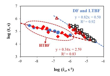
Fig. 3.12 The Monkman-Grant (MG) plot for all data reported here: #1 LLDPE ( $\Box$ ), #2 HDPE ( $\triangle$ ), #3 HDPE ( $\bigcirc$  and  $\spadesuit$ ) and #4 HDPE ( $\diamondsuit$  and  $\blacklozenge$ ) in which unfilled symbols represent ductile failure and filled symbols brittle failure.
