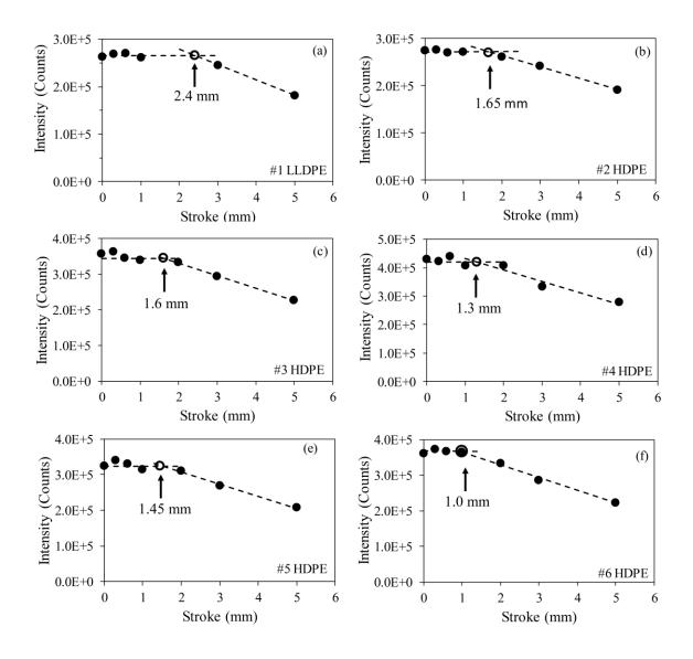
Fig. 4.8 Absolute intensity of peak (110) from the orthorhombic structure of PE, as a function of stroke used to stretch the specimens.
