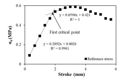
Fig. 5.9 Plot of reference stress ( $\sigma_0$ ) as a function of stroke for a NPR specimen, and depiction of the process to determine the first critical point for deformation transition.
