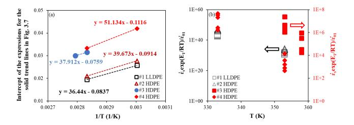
Fig. 3.8 Summary of analysis for process 1 based on the Eyring's model: (a) The intercept values for the solid trend lines in Fig. 3.7, and (b) values for  $\frac{\hat{\varepsilon}_s}{\hat{\varepsilon}_{01}} \exp\left(\frac{E_1}{RT}\right)$  versus *T*.
