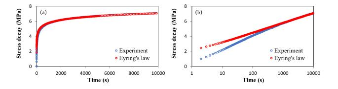
Fig. 5.8 Curve fitting of experimental data according to the Eyring's Law.
