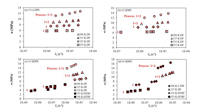
Fig. 3.13 Comparison of experimental measurements (unfilled and filled symbols of large size in black) with predictions based on the Eyring's Law using parameters listed in Tab. 3.2 (unfilled symbols of small size in red).
