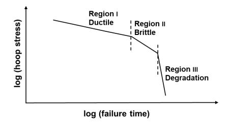
Fig. 1.1 Schematic plot of the typical hoop stress versus failure time for PE pipes.
