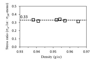
Fig. 4.11 Ratio of  $\sigma_{st}$  at the 1<sup>st</sup> critical point from the MR test ( $\sigma_{st}$ -1st) to yield stress from the standard tensile test ( $\sigma_{yld}$ -mono) listed in Tab. 4.1, plotted as a function of PE density.
