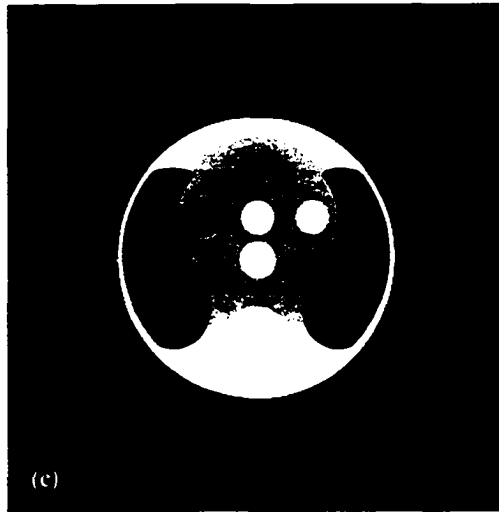
Figure 4-5 – Truncated images for FOVs of (a) 24 cm (b) 22 cm and (c) 20 cm. Images are shown in a window of 400 and level of 1000 (HU + 1000).
