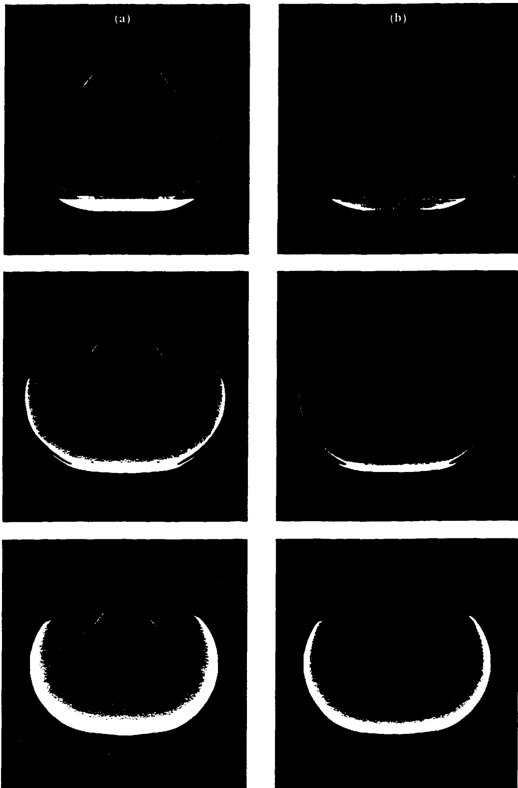
Figure 4-12 – Effect of the stationary couch in the sinogram merging technique. All images are merged images. Top row is 24 cm field-of-view (FOV), middle row is 22 cm FOV, and bottom row is 20 cm FOV. Transmission data normalized to (a) airscan without couch (b) airscan with couch. Images are shown in a window of 400 and level of 1000 (HU + 1000).
