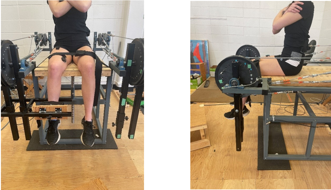
Figure 3-3: Maximum isometric leg extension apparatus.
