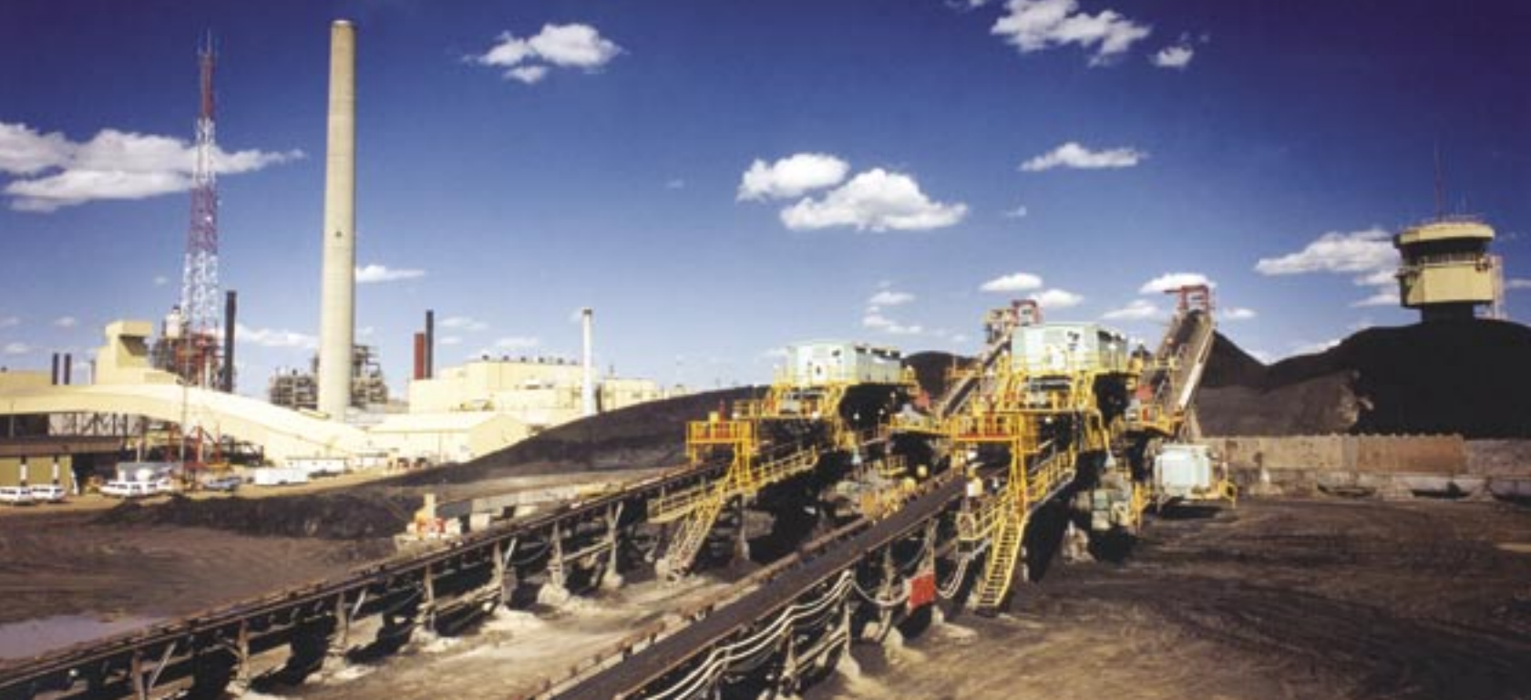
A conveyor moves mined oil sand toward the Mildred Lake extraction facility.
