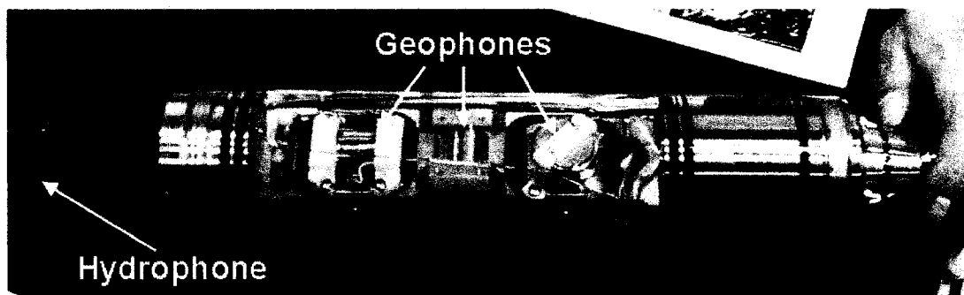
Figure 4-3) A cutaway view of the OYO 4 Component sensor. The gimballed geophones can be seen and the hydrophone is situated at the left end of the sensor.
