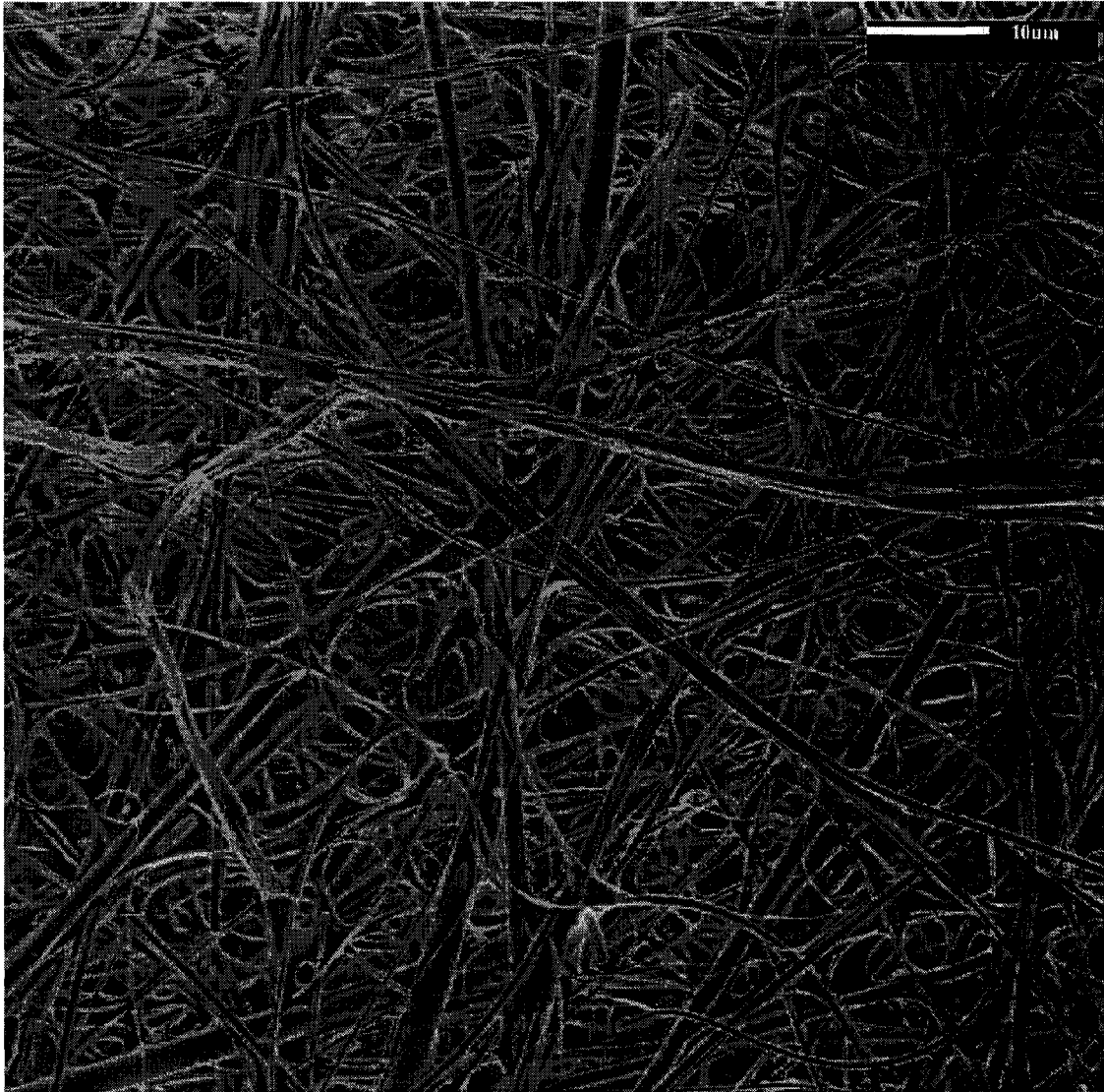
Figure 13. Pallflex Pure Quartz-fiber - Surface as Observed by SEM (1000x)
