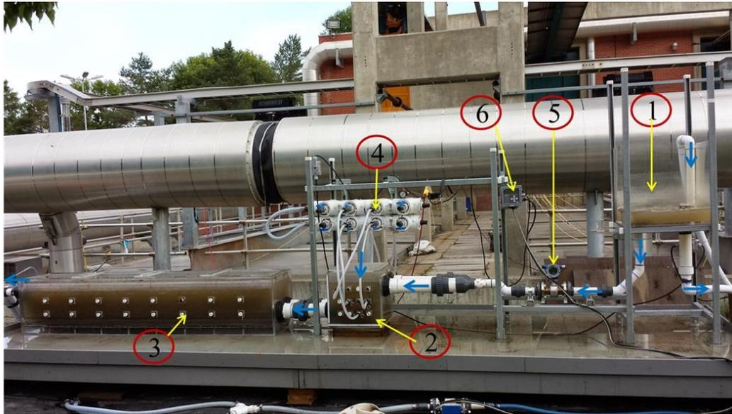
Fig. 34: Photo of experimental setup showing the components: (1) constant head tank, (2) mixing tank, (3) grit tank, (4) manifold for cross jets, (5) flow meter for the longitudinal flow and (6) flow meter for the transverse flow; Arrows show the flow direction.
