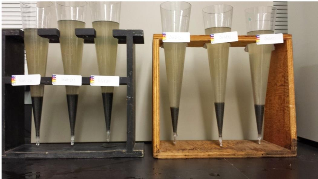
Fig. 35: Imhoff cone experiment showing three samples of each of the two tests; Settleable grit is shown at bottom of the cones with black colors.
