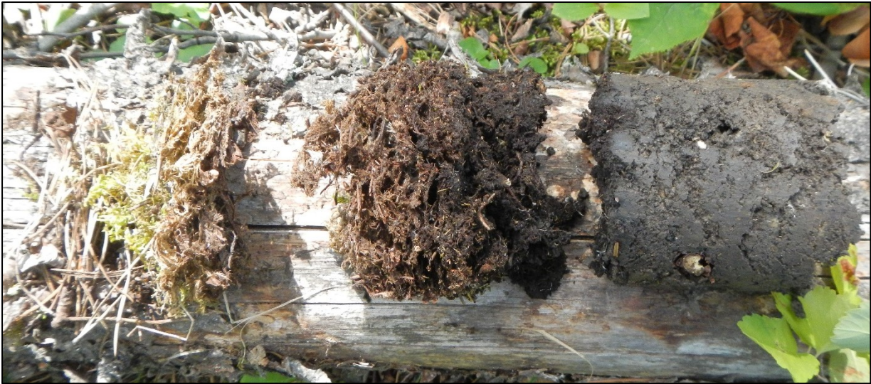
Figure 6. A standard site soil core. Litter layer with fine litter and loose surface moss (left), Duff layer with characteristic wafer-like semi-decomposed organic transition on top and dark completely decomposed organic on bottom (middle), and Mineral layer (right).
