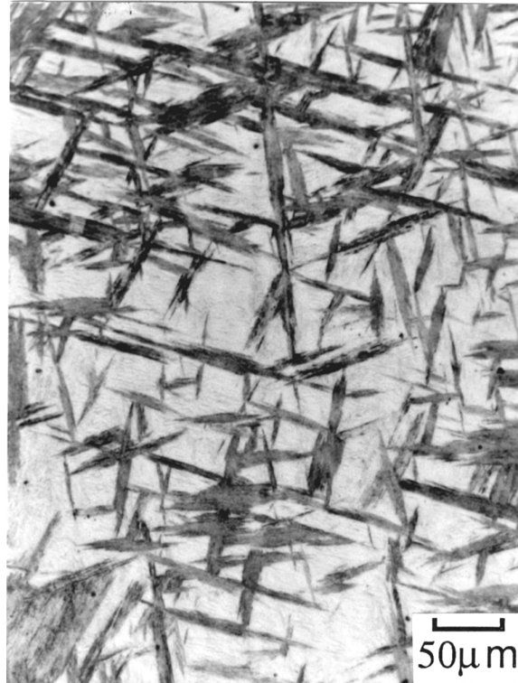
Figure 2-26: Optical micrograph illustrating sheaves of bainitic ferrite in a partially transformed (395°C) Fe-0.3C-4Cr wt% alloy [Bhadeshia, 2001] (Reprinted with permission).
