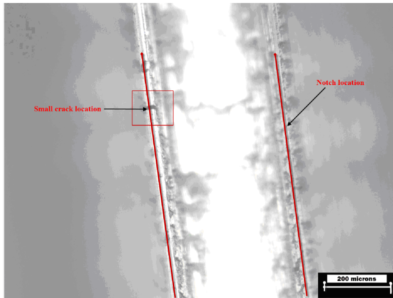
Figure 5-28: Full size Charpy notch location showing a pre-existing crack (indicated by the red box). The specimen is Steel X. Steel Y also had these types of cracks.
