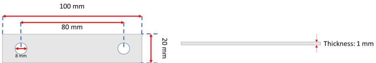
Fig. 7-5. The dimensions of a U-bending sample used in this study.
