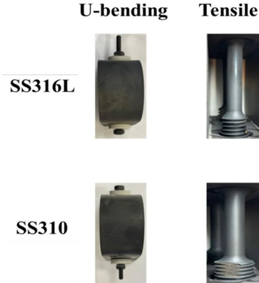
Fig. 7-10. Photographic images of U-bending and uniaxial tensile specimens after testing in 0.5 M  $K_2CO_3$  + 3500 ppm  $Cl^-$  + 2500 ppm  $S^{2-}$  +10 wt.% acetic acid at 365 °C.
