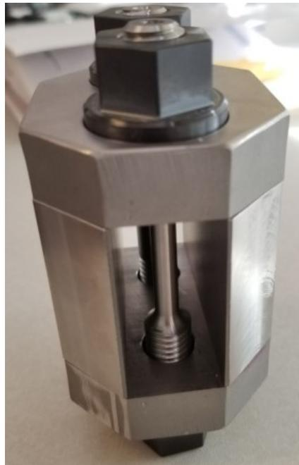
Fig. 7-3. A photographic image of loading stressing frame and testing specimens before accommodating into a static autoclave.
